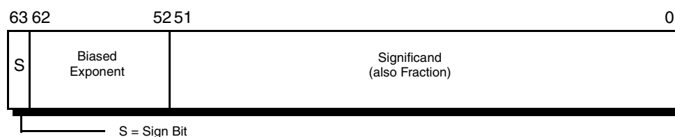
Figure 4-15. 128-Bit Media Floating-Point Data Types
