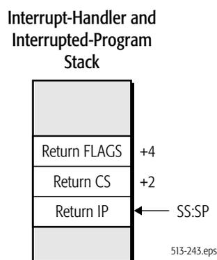
**Figure 8-6. Stack After Interrupt in Real Mode**
