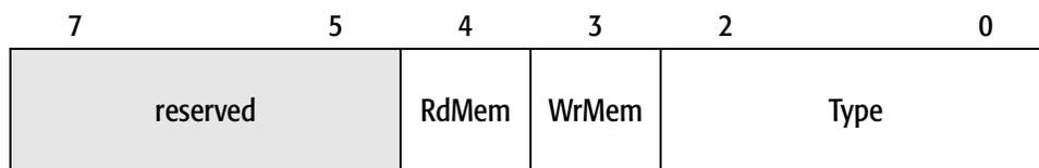
**Figure 7-11. Extended MTRR Type-Field Format (Fixed-Range MTRRs)**
