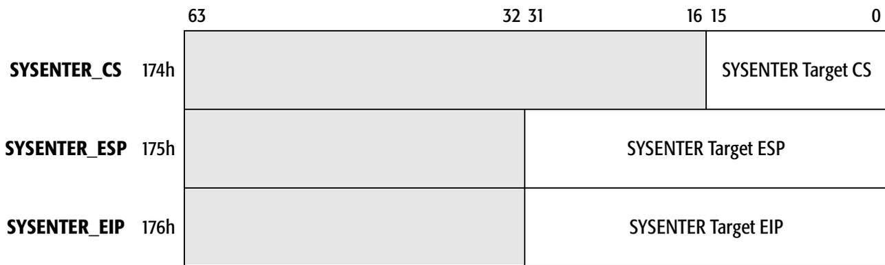
**Figure 6-2. SYSENTER\_CS, SYSENTER\_ESP, SYSENTER\_EIP MSRs**
