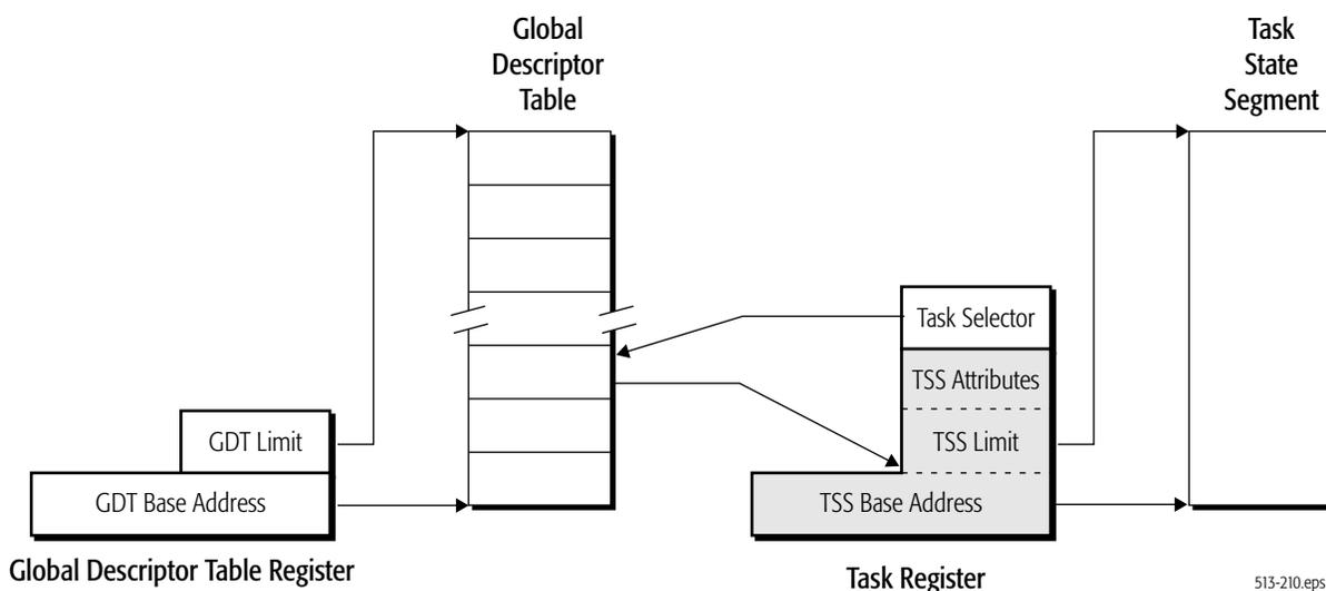
**Figure 12-5. Relationship between the TSS and GDT**
