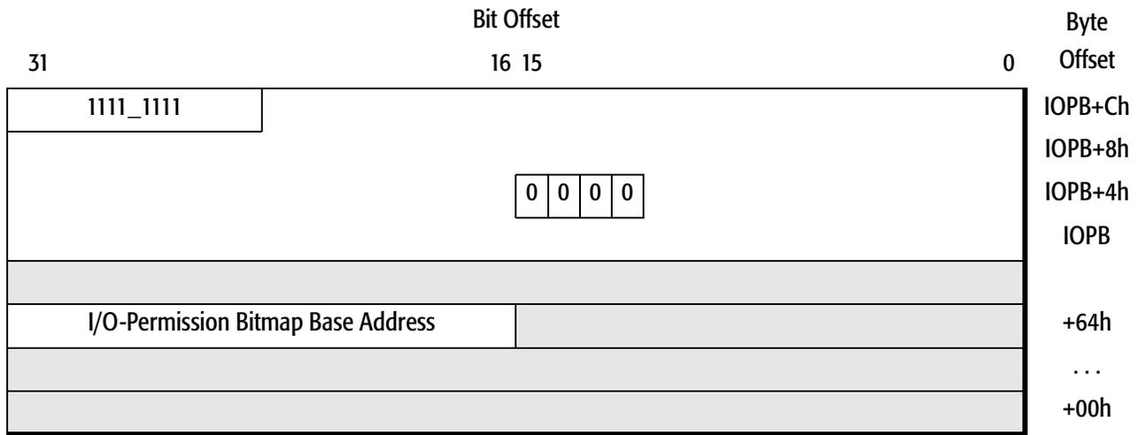
Figure 12-7. I/O-Permission Bitmap Example
