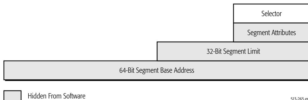
**Figure 4-5. FS and GS Segment-Register Format–64-Bit Mode**
