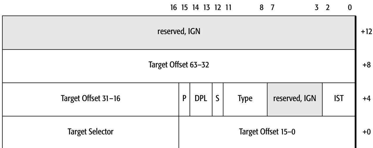
**Figure 4-24. Interrupt-Gate and Trap-Gate Descriptors—Long Mode**
