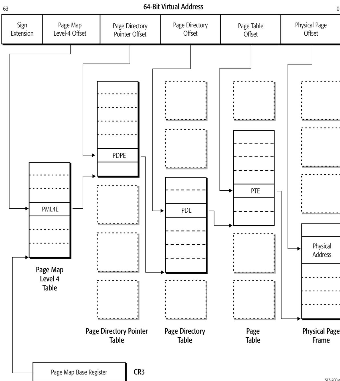
**Figure 5-1. Virtual to Physical Address Translation—Long Mode**
