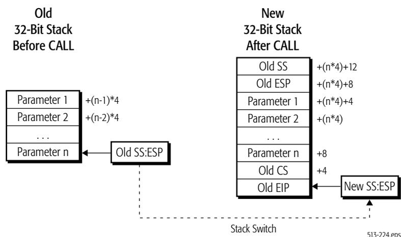
**Figure 4-33. Legacy-Mode 32-Bit Stack Switch, with Parameters**
