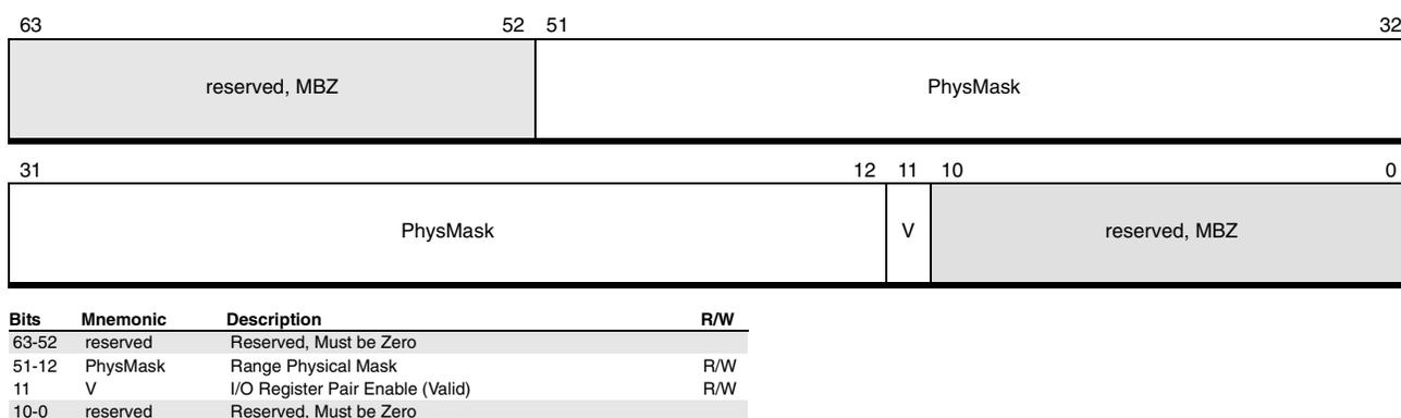
**Figure 7-13. IORRMask<sub>n</sub> Register**
