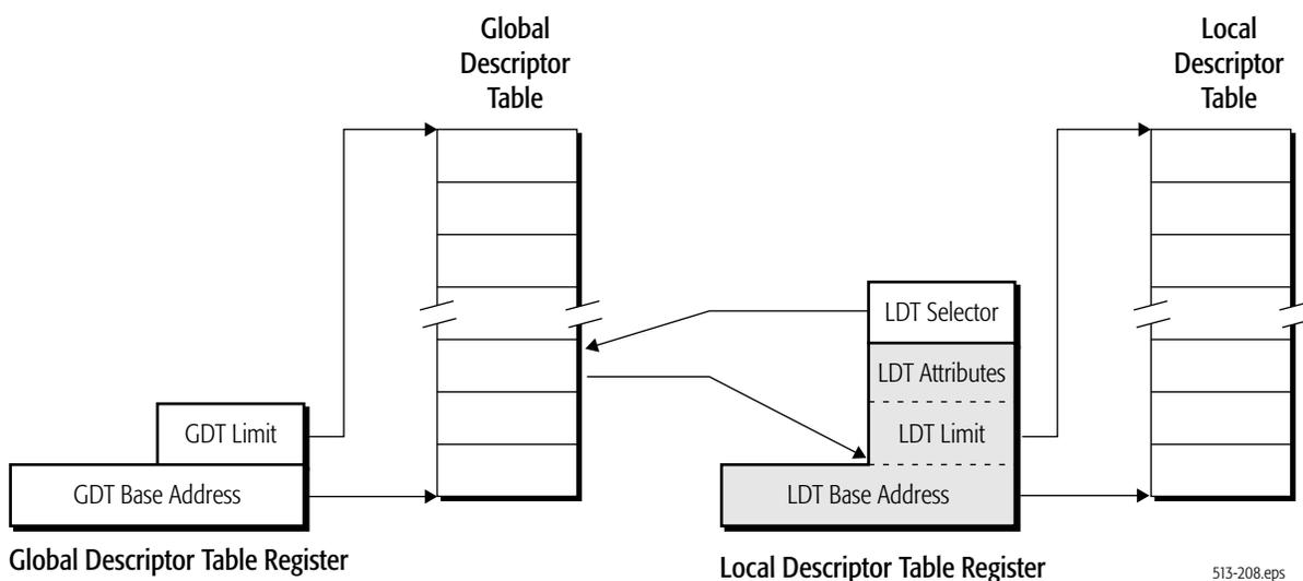
**Figure 4-9. Relationship between the LDT and GDT**
