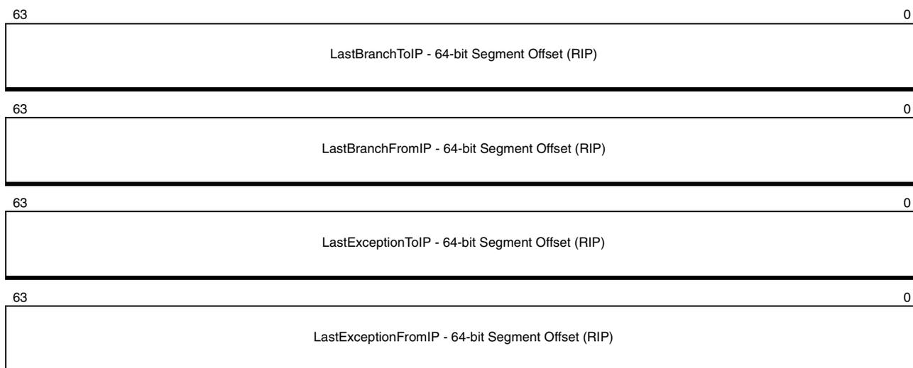
**Figure 13-5. Control-Transfer Recording MSRs**
