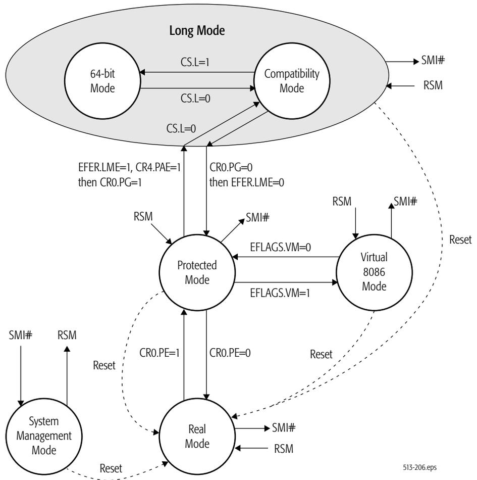
**Figure 1-6. Operating Modes of the x86-64 Architecture**
