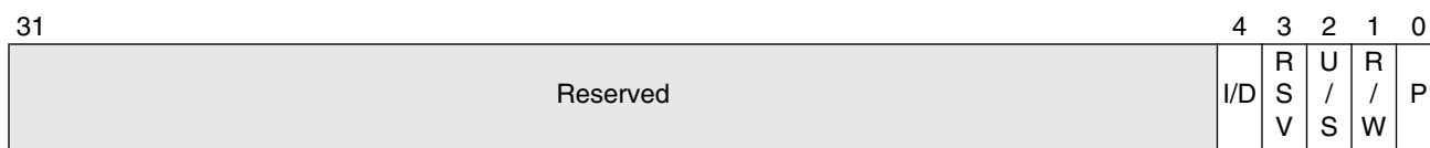
Figure 8-3. Page-Fault Error Code
