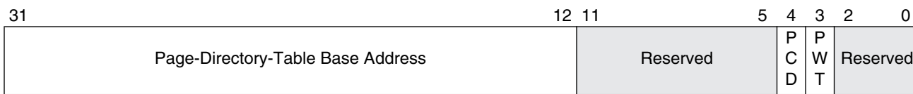
Figure 3-4. Control Register 3 (CR3)—Legacy-Mode Non-PAE Paging
