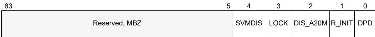
Figure 15-25. Layout of VM_CR MSR (C001_0114h)
