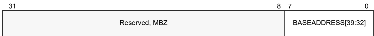
Figure 15-9. Format of DEV_BASE_HI[n] Registers
