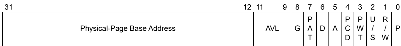
Figure 5-6. 4-Kbyte PTE—Non-PAE Paging Legacy-Mode
