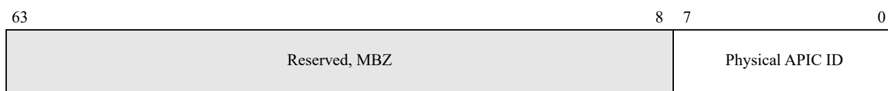
Figure 15-22. Doorbell Register, MSR C001_011Bh
