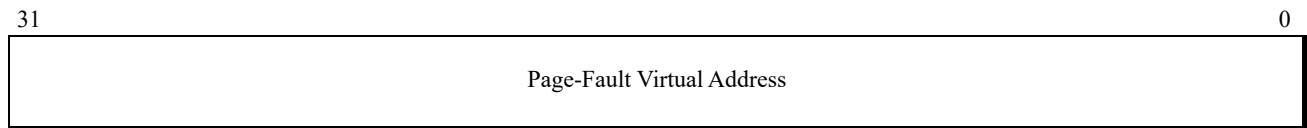
Figure 3-2. Control Register 2 (CR2)—Legacy-Mode
