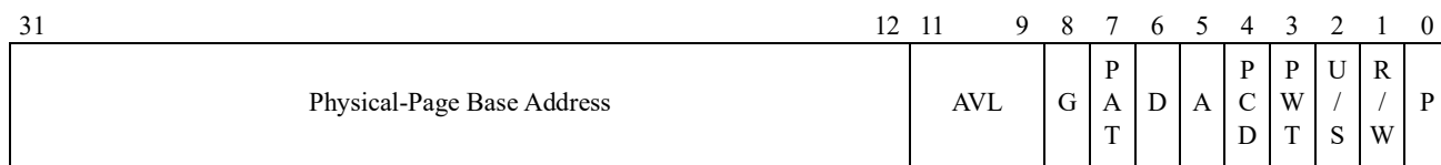
Figure 5-6. 4-Kbyte PTE—Non-PAE Paging Legacy-Mode
