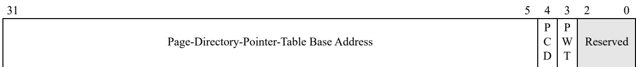
Figure 3-5. Control Register 3 (CR3)—Legacy-Mode PAE Paging
