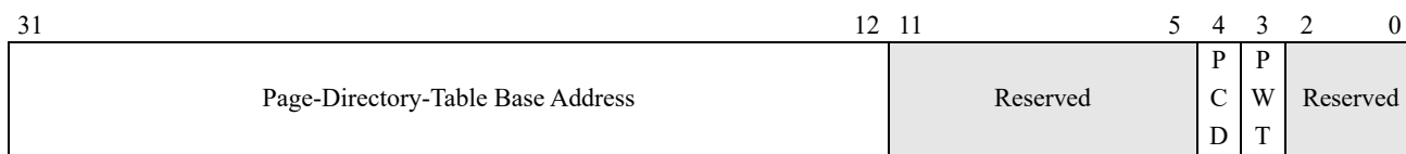
Figure 5-2. Control Register 3 (CR3)—Non-PAE Paging Legacy-Mode
