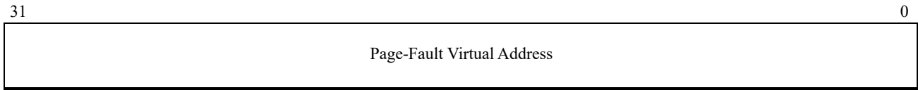
Figure 3-2. Control Register 2 (CR2)—Legacy-Mode
