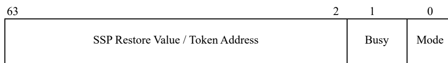
Figure 18-4. Shadow Stack Restore Token
