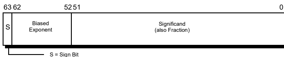
Figure 4-4. Floating-Point Data Types
