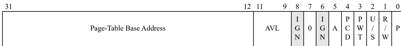
Figure 5-5. 4-Kbyte PDE—Non-PAE Paging Legacy-Mode
