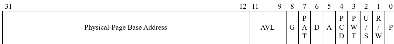
Figure 5-6. 4-Kbyte PTE—Non-PAE Paging Legacy-Mode
