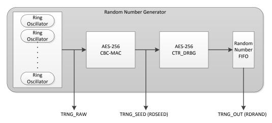
Note that any values that are returned to software via the TRNG\_RAW or TRNG\_SEED registers are immediately discarded and not used in the rest of the RNG hardware. All 3 registers are built so a different value is returned automatically on every read.
