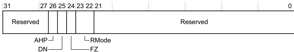
Figure B3-21 FPDSCR bit assignments
