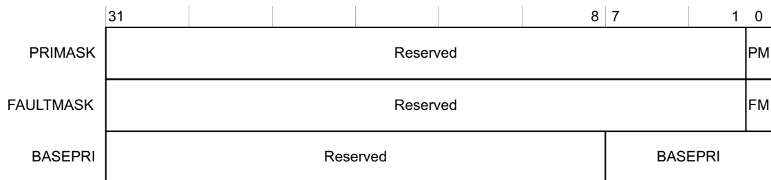
Figure B1-2 The special-purpose mask registers
