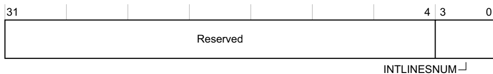
Figure B3-22 ICTR bit assignments
