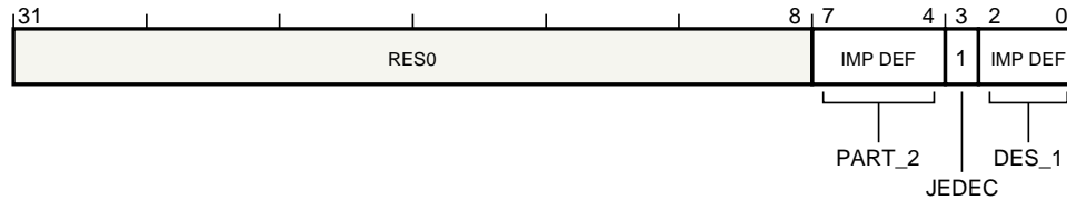
Figure 4.53: ERRPIDR2 the component uses a 16-bit part number
