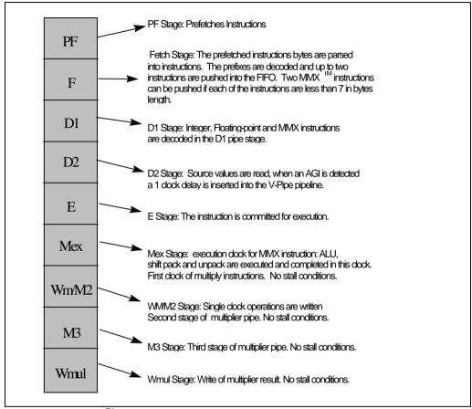
Figure 2-2. MMX<sup>™</sup> Instruction Flow in a Pentium ® Family Processor with MMX Technology
