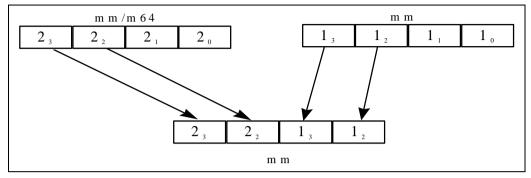
Figure 5-4. Result of Non-Interleaved Unpack in MM1
