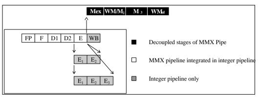
Figure 2-1 . MMX<sup>™</sup> Pipeline Structure
