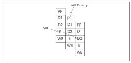
Figure 3-1. Pipeline Example of AGI Stall
