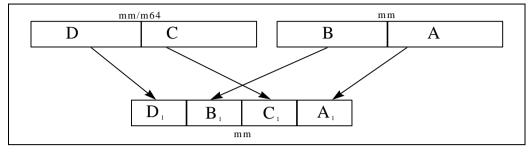
Figure 5-2. Interleaved Pack with Saturation Example
