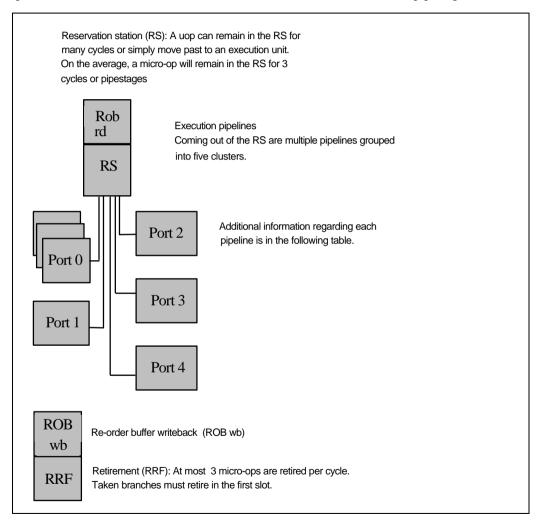
Figure 2-4. Out-Of-Order Core and Retirement Pipeline
