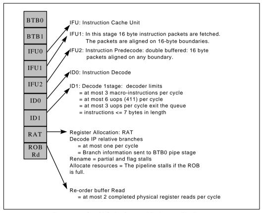
Figure 2-3. Out-Of-Order Core and Retirement Pipeline
