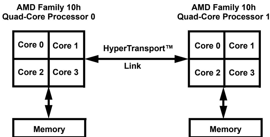
**Figure 5. Dual Quad-Core AMD Family 10h Processor Configuration**
