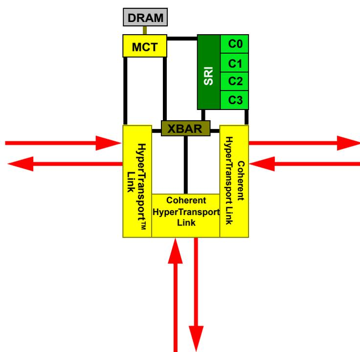
**Figure 7. Internal Resources Associated with a Multiprocessor Node**
