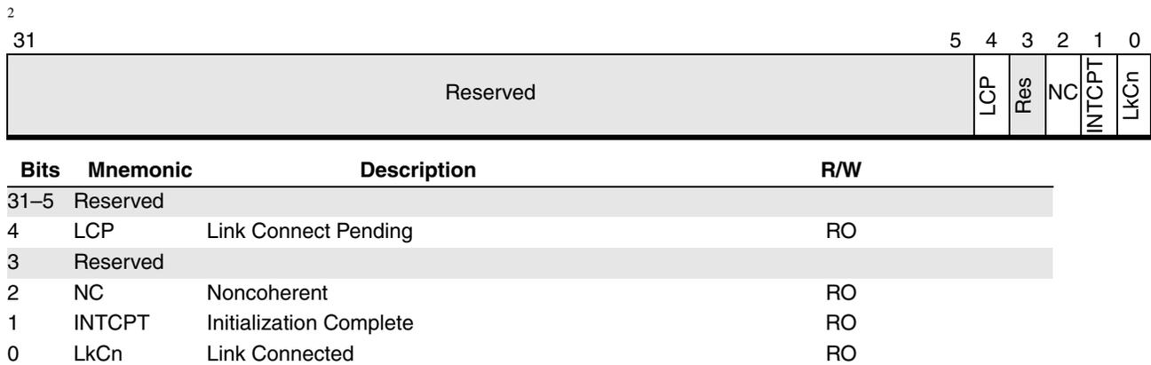
**Figure 14. Link Type Registers F0x[F8, D8, B8, 98]**
