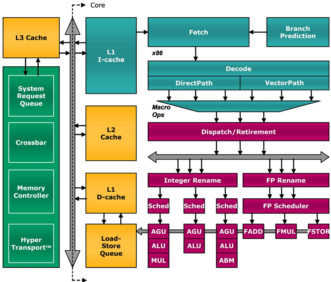
Figure 8. AMD Family 10h Processors Block Diagram
