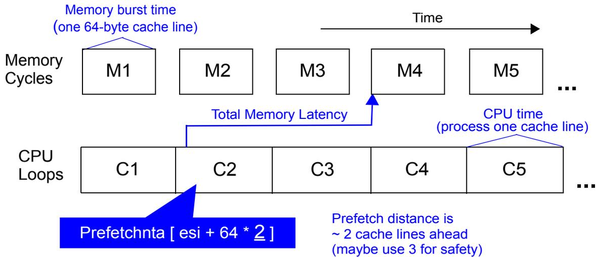
**Figure 2. Processor-Limited Code**
