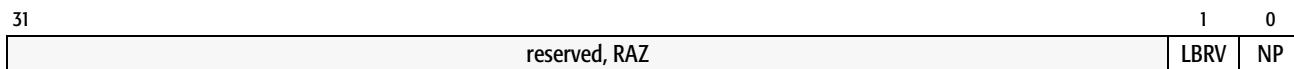
Figure B-3. SVM Revision and Feature Identification in EDX, Extended Function 8000_000Ah
