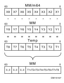
The subtraction operation presented above is an absolute difference, that is, t = abs(x-y). The byte values are stored in temporary space, all values are summed together, and the result is written into the lower word of the destination register.
