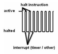
As shown in the illustration of Figure 9-2, the processor is in either active or idle (halted) state. ACPI defines four C-state types (C0, C1, C2 and C3). Processor-specific C states of an IA-32 processor can be mapped to an ACPI C-state type via ACPI standard mechanisms. The C-state types are divided into two categories: active (C0), in which the processor consumes full power; and idle (C1-3), in which the processor is idle and may consume significantly less power.
