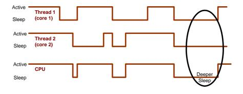
2. Enabling both core to take advantage of Intel Enhanced Deeper Sleep:
