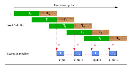
The following relationship calculates the prefetch scheduling distance (or prefetch iteration distance) for the case when memory throughput latency is greater than the compute latency.
