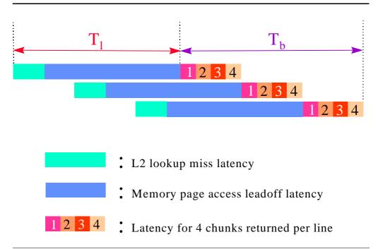
Assume that three cache lines are accessed per iteration and four chunks of data are returned per iteration for each cache line. Also assume these 3 accesses are pipelined in memory subsystem. Based on these assumptions,
