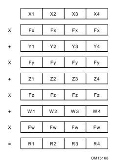
Figure 5-2 shows how 1 result would be computed for 7 instructions if the data were organized as AoS and using SSE alone: 4 results would require 28 instructions.
