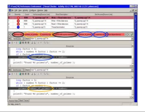
Figure A-2 shows Intel Thread Checker displaying the source code of the selected instance from a list of detected data race conditions that occurred during threaded execution. The target operands (a synchronization variable shared by more than one threads) of the race condition, the type of data operation on the target operand, and source code locations are displayed in the graphical user interface.
