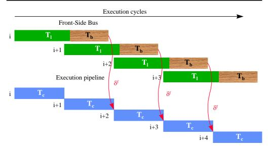
For this particular example the prefetch scheduling distance is greater than 1. Data being prefetched for iteration i will be consumed in iteration i+2.
