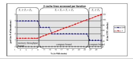
The prefetch scheduling distance is a step function of  $T_c$ , the computation latency. The steady state iteration latency (il) is either memory-bound or compute-bound depending on  $T_c$  if prefetches are scheduled effectively.
