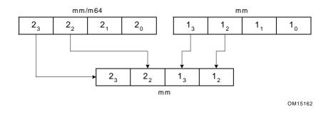
Code in the Example 4-6 unpacks two packed-word sources in a non-interleaved way. The goal is to use the instruction which unpacks doublewords to a quadword, instead of using the instruction which unpacks words to doublewords.
