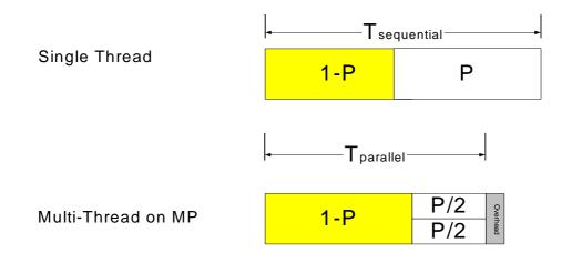
When optimizing application performance in a multithreaded environment, control flow parallelism is likely to have the largest impact on performance scaling with respect to the number of physical processors and to the number of logical processors per physical processor.
