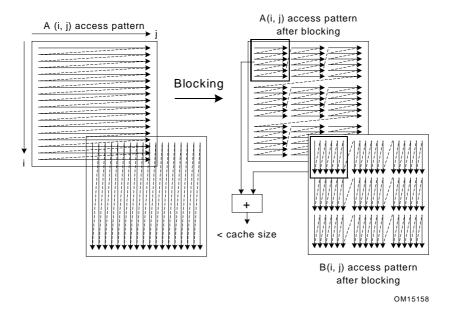
As one can see, all the redundant cache misses can be eliminated by applying this loop blocking technique. If MAX is huge, loop blocking can also help reduce the penalty from DTLB (data translation look-aside buffer) misses. In addition to improving the cache/memory performance, this optimization technique also saves external bus bandwidth.
