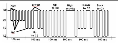
Figure 9-3 Application of C-states to Idle Time
