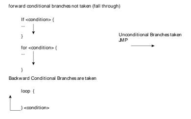
Examples 2-6, Example 2-7 provide basic rules for a static prediction algorithm.
