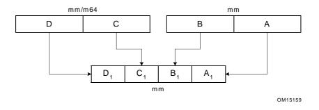
Figure 4-2 illustrates two values interleaved in the destination register, and Example 4-4 shows code that uses the operation. The two signed doublewords are used as source operands and the result is interleaved signed words. The pack instructions can be performed with or without saturation as needed.
