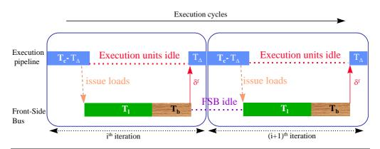
As you can see from Figure E-2, the execution pipeline is stalled while waiting for data to be returned from memory. On the other hand, the front side bus is idle during the computation portion of the loop. The memory access latencies could be hidden behind execution if data could be fetched earlier during the bus idle time.
