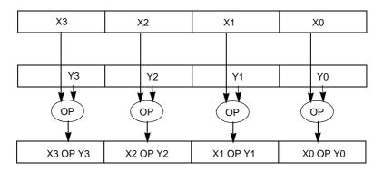
The AoS data structure is often used in 3D geometry computations. SIMD technology can be applied to AoS data structure using a horizontal computation model. This means that the x, y, z, and w components of a single vertex structure (that is, of a single vector
