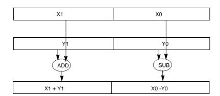
Figure 5-4 Asymmetric Arithmetic Operation of the SSE3 Instruction
