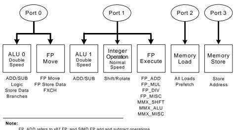
Figure 1-4 Execution Units and Ports in the Out-Of-Order Core
