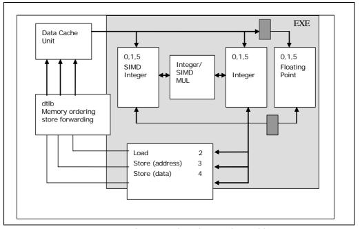
Figure 2-2. Execution Core of Intel Core Microarchitecture
