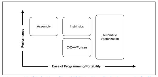
Figure 4-2. Hand-Coded Assembly and High-Level Compiler Performance Trade-offs
