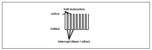
Figure 11-2. Active Time Versus Halted Time of a Processor
