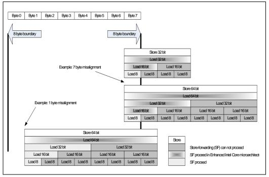
Figure 2-3. Store-Forwarding Enhancements in Enhanced Intel Core Microarchitecture
