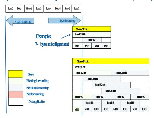
Figure 2-8. Store-Forwarding Enhancement in Intel Microarchitecture (Nehalem)
