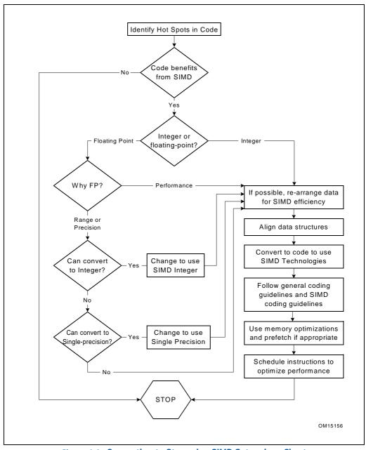
Figure 4-1. Converting to Streaming SIMD Extensions Chart
