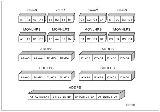
Figure 6-4. Horizontal Add Using MOVHLPS/MOVLHPS
