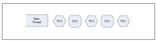
Figure 8-2. Single-threaded Execution of Producer-consumer Threading Model
