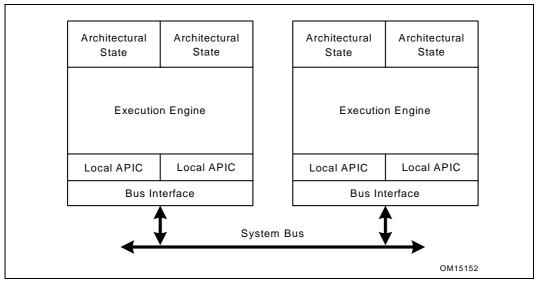
Figure 2-12. Hyper-Threading Technology on an SMP
