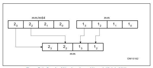
Figure 5-4. Result of Non-Interleaved Unpack High in MM1
