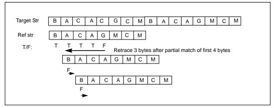
Figure 10-2. Retrace Inefficiency of Byte-Granular, Brute-Force Search
