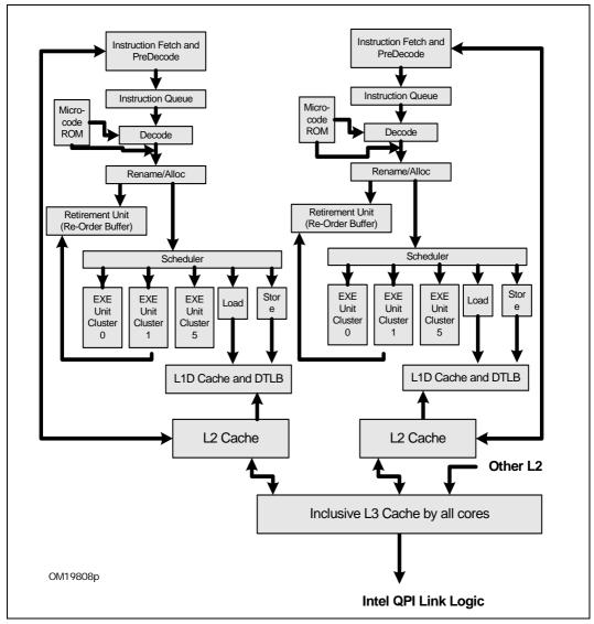
Figure 2-5. Intel Microarchitecture (Nehalem) Pipeline Functionality
