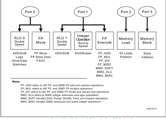
Figure 2-10. Execution Units and Ports in Out-Of-Order Core
