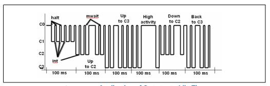
Figure 11-3. Application of C-states to Idle Time
