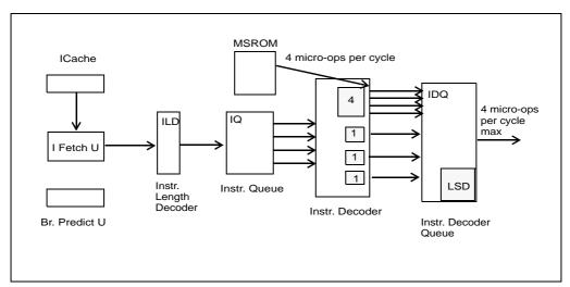
Figure 2-6. Front End of Intel Microarchitecture (Nehalem)
