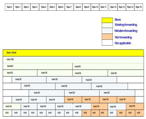
Intel microarchitecture (Nehalem) allows store-to-load forwarding to proceed regardless of store address alignment (The white space in the diagram does not
