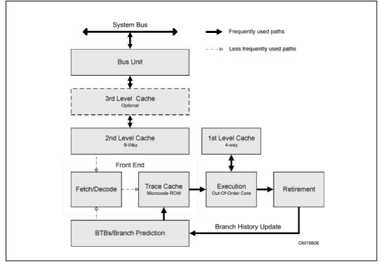
Figure 2-9. The Intel NetBurst Microarchitecture
