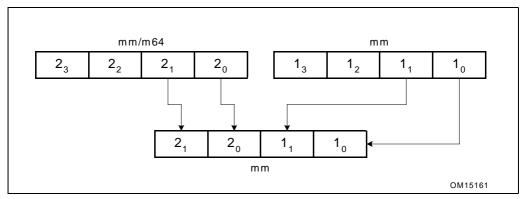
Figure 5-3. Result of Non-Interleaved Unpack Low in MMO
