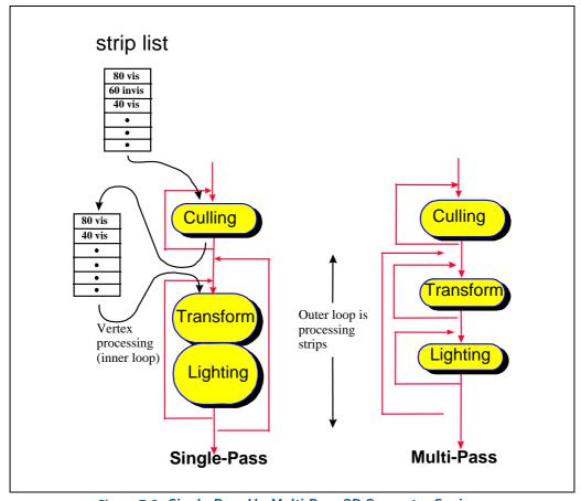
Figure 7-9. Single-Pass Vs. Multi-Pass 3D Geometry Engines
