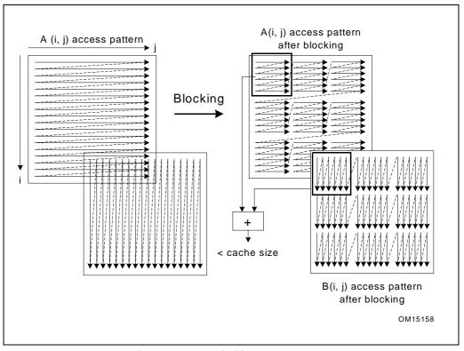
Figure 4-3. Loop Blocking Access Pattern
