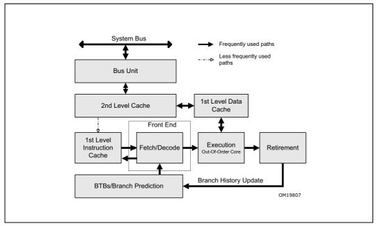
Figure 2-11. The Intel Pentium M Processor Microarchitecture
