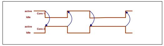
Figure 11-5. Thread Migration in a Multicore Processor
