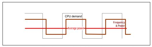
Figure 11-4. Profiles of Coarse Task Scheduling and Power Consumption
