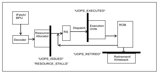
Figure B-2. PMU Specific Event Logic Within the Pipeline
