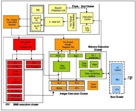
Figure 12-1. Intel Atom Microarchitecture Pipeline
