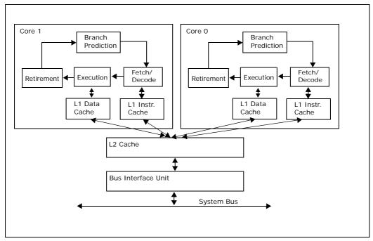
Figure 2-4. Intel Advanced Smart Cache Architecture
