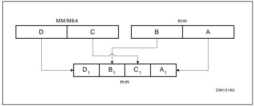
Figure 5-2. Interleaved Pack with Saturation
