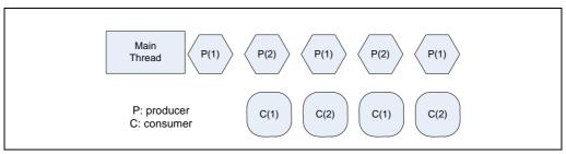
Figure 8-3. Execution of Producer-consumer Threading Model on a Multicore Processor
