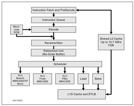
Figure 2-1. Intel Core Microarchitecture Pipeline Functionality
