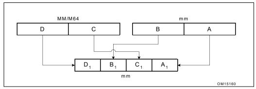
Figure 5-2. Interleaved Pack with Saturation
