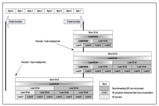
Figure 2-10. Store-Forwarding Enhancements in Enhanced Intel Core Microarchitecture
