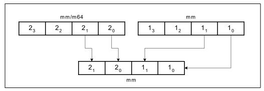
Figure 5-3. Result of Non-Interleaved Unpack Low in MMO
