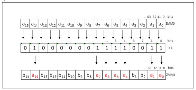
The result of the execution with zeroing masking is (notice the  $\{z\}$  in the instruction): vmovaps zmm1  $\{k1\}\{z\}$ , zmm0
