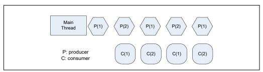
Figure 9-3. Execution of Producer-consumer Threading Model on a Multicore Processor
