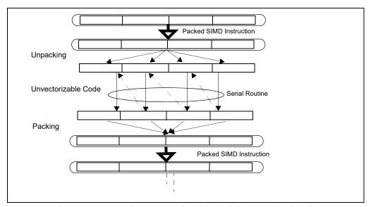
Figure 3-1. Generic Program Flow of Partially Vectorized Code
