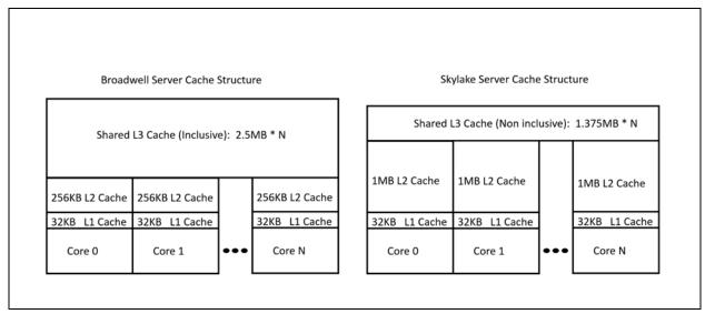
Figure 2-2. Broadwell Microarchitecture and Skylake Server Microarchitecture Cache Structures
