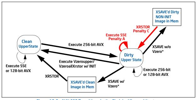
Figure 12-2. AVX-SSE Transitions in the Skylake Microarchitecture
