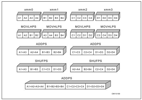
Figure 6-4. Horizontal Add Using MOVHLPS/MOVLHPS
