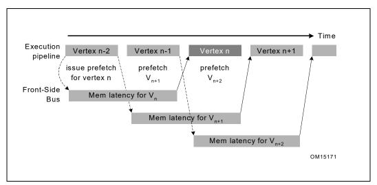
Figure 7-4. Memory Access Latency and Execution With Prefetch
