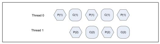
Figure 9-4. Interlaced Variation of the Producer Consumer Model
