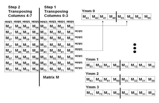
The following figure describes step 1 of the 8x8 matrix transpose with vinsertf128. Step 2 performs the same operations on different columns.
