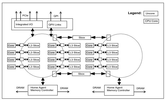
Figure 2-6. An Example of the Haswell-E Microarchitecture Supporting 12 Processor Cores
