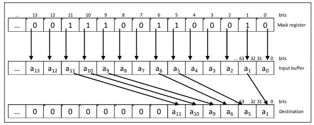
Figure 15-4. Data Compress Operation
