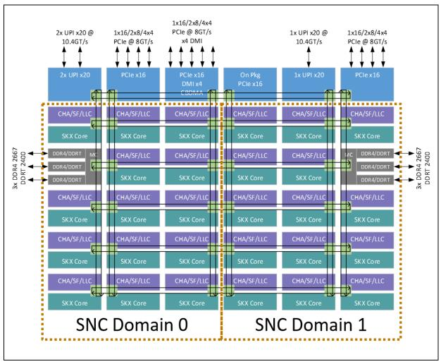
Figure 8-1. Example of SNC Configuration
