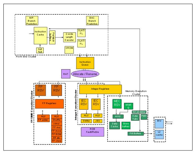
Figure 16-3. Silvermont Microarchitecture Pipeline
