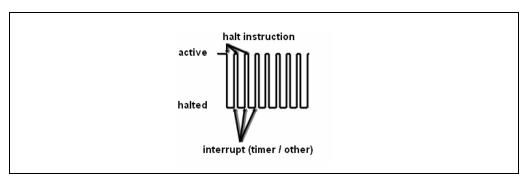
Figure 14-2. Active Time Versus Halted Time of a Processor
