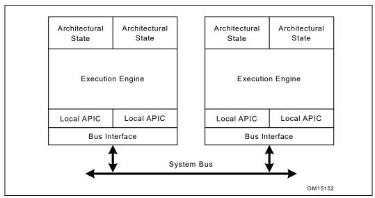
Figure 2-16. Hyper-Threading Technology on an SMP
