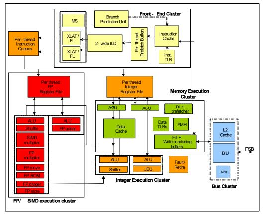
Figure D-1. Intel Atom Microarchitecture Pipeline
