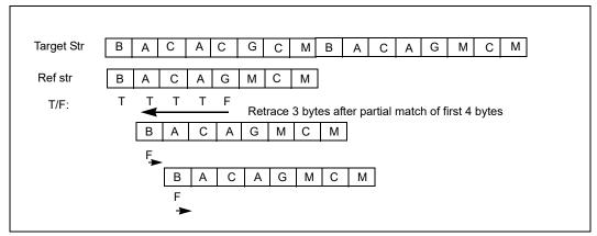
Figure 11-2. Retrace Inefficiency of Byte-Granular, Brute-Force Search
