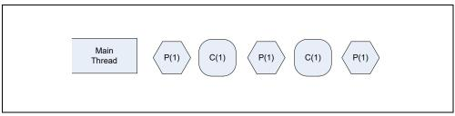
Figure 9-2. Single-threaded Execution of Producer-consumer Threading Model
