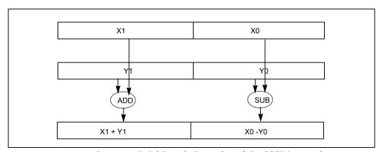
Figure 6-5. Asymmetric Arithmetic Operation of the SSE3 Instruction
