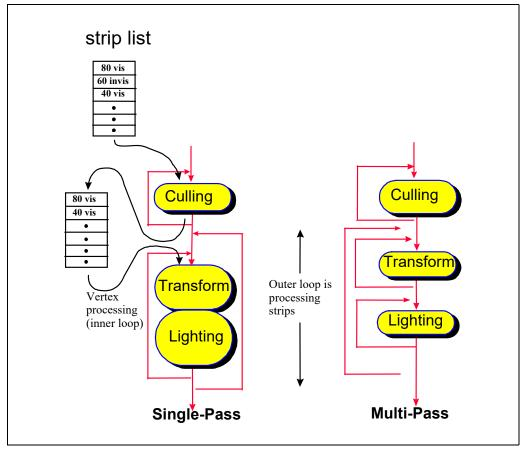
Figure 7-10. Single-Pass Vs. Multi-Pass 3D Geometry Engines
