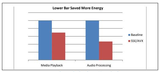
Figure 14-8. Energy Saving due to Vectorization
