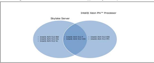
Figure 15-1. Intel® AVX-512 Extensions Supported by Skylake Server Microarchitecture and Knights
