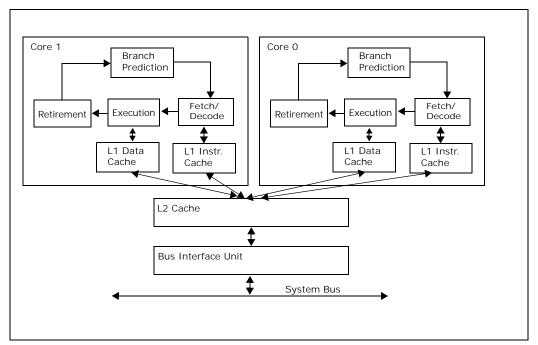
Figure 2-11. Intel Advanced Smart Cache Architecture
