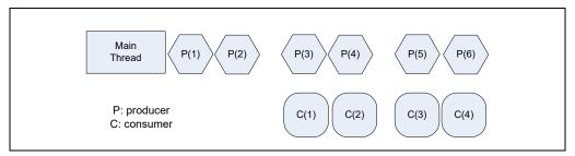
Figure 9-5. Batched Approach of Producer Consumer Model
