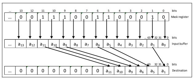
Figure 15-5. Data Expand Operation
