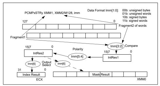
Figure 11-1. SSE4.2 String/Text Instruction Immediate Operand Control
