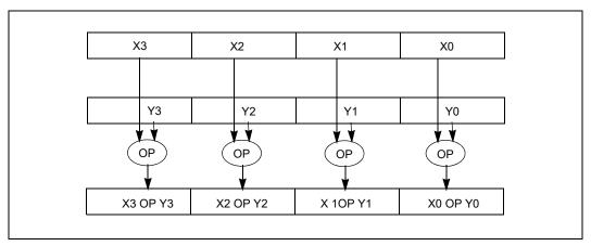
Figure 6-1. Homogeneous Operation on Parallel Data Elements
