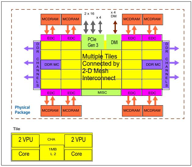
Figure 17-1. Tile-Mesh Topology of the Knights Landing Microarchitecture
