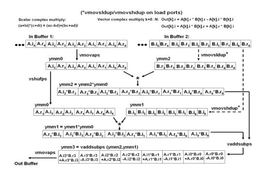
Example 12-21 includes two versions of the complex multiply. Both versions are unrolled twice. Alternative 1 shuffles all the data in registers. Alternative 2 shuffles data while it is loaded from memory.
