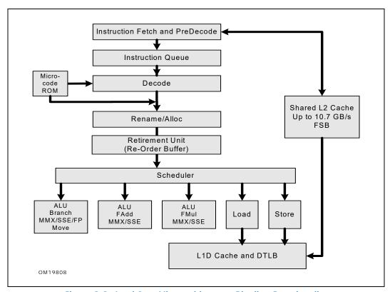
Figure 2-8. Intel Core Microarchitecture Pipeline Functionality
