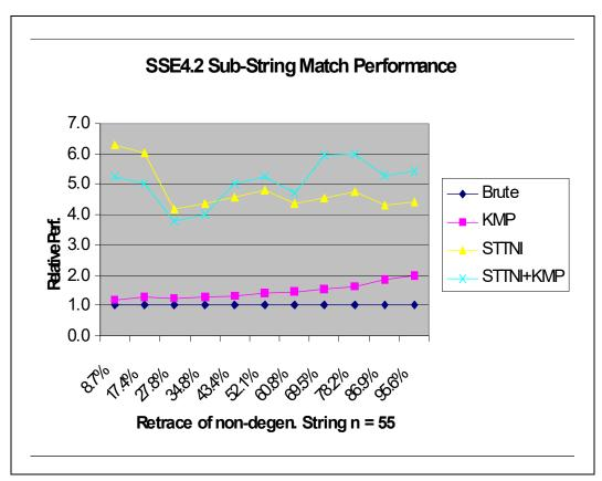
Figure 11-3. SSE4.2 Speedup of SubString Searches
