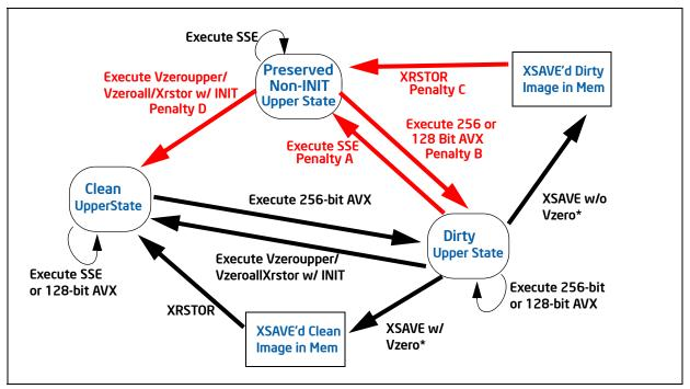
Figure 12-1. AVX-SSE Transitions in the Broadwell, and Prior Generation Microarchitectures
