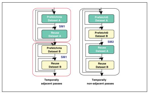
Figure 7-9. Examples of Prefetch and Strip-mining for Temporally Adjacent and Non-Adjacent Passes Loops
