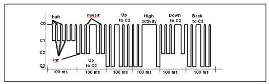
Figure 14-3. Application of C-states to Idle Time
