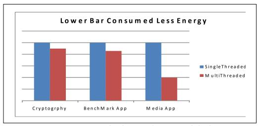
Figure 14-7. Energy Saving due to Performance Optimization
