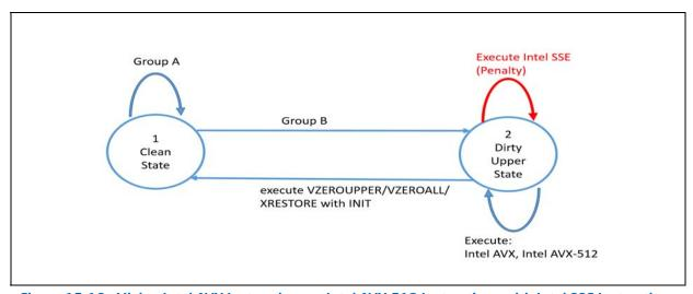
Figure 15-16. Mixing Intel AVX Instructions or Intel AVX-512 Instructions with Intel SSE Instructions
