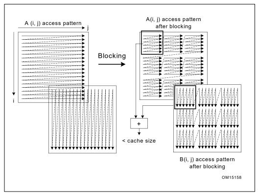
Figure 4-5. Loop Blocking Access Pattern
