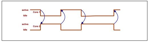
Figure 14-5. Thread Migration in a Multicore Processor
