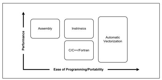
Figure 4-4. Hand-Coded Assembly and High-Level Compiler Performance Trade-offs
