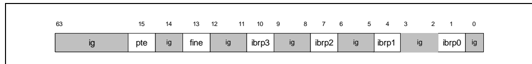
Figure 3-14. Instruction Address Range Configuration Register (PMC_IAM_CFG)
