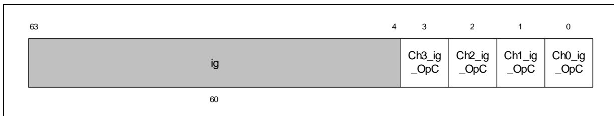
Figure 3-17. Opcode Match Configuration Register
