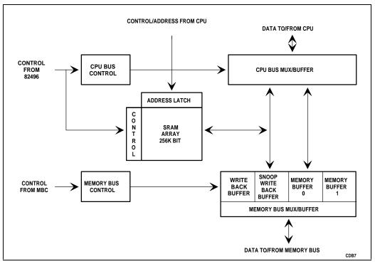
Figure 2-2. 82491 Cache SRAM Block Diagram
