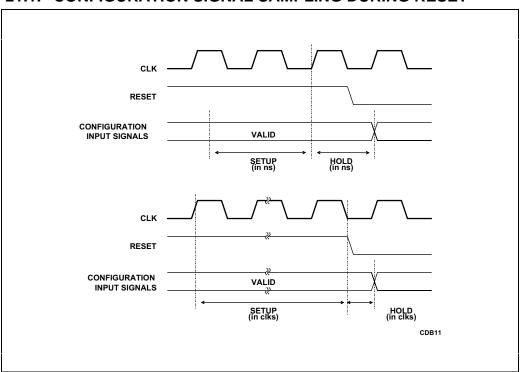
21.1. CONFIGURATION SIGNAL SAMPLING DURING RESET
