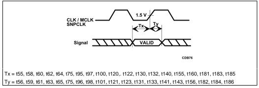
Figure 23-7. Setup and Hold Timings
