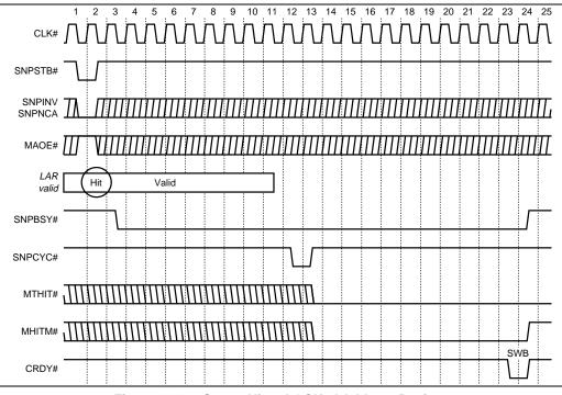
Figure 22-17. Snoop Hit to LOCKed Address Register
