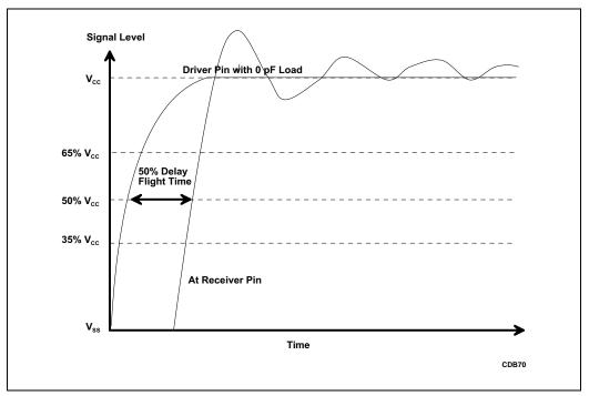
Figure 7-1. Determination of Flight Time
