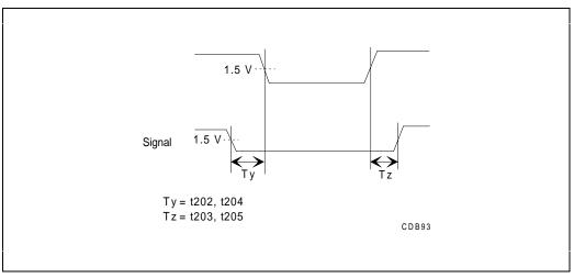
Figure 14-9. Setup and Hold Timings to Strobes
