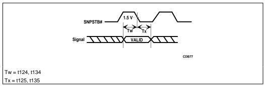
Figure 7-8. Setup and Hold Timings in Strobed Snooping Mode
