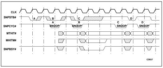
Figure 5-9. Fastest Asynchronous Snooping
