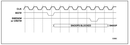
Figure 22-12. Snoop Response Blocking Using BGT#
