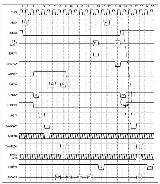
Figure 22-3. Non-Split LOCKed Read Miss with Clean Replacement
