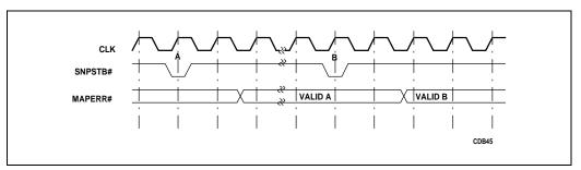
Figure 5-17. MAPERR# Timing for Synchronous Snoop Mode
