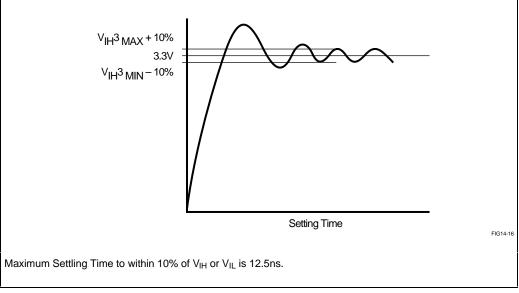
Figure 14-16. Settling Time
