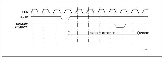
Figure 5-13. Snoop Response Blocking Using BGT#
