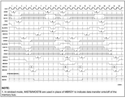
Figure 6-8. Locked Read Modify Write Cycles
