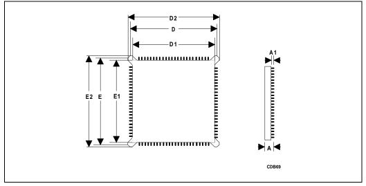
Figure 9-3. 82491 Cache SRAM Mechanical Specifications
