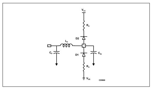
Figure 24-4. Complete Input Model Including Diode
