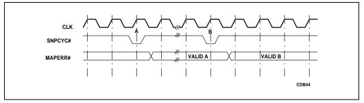
Figure 5-27. MAPERR# Timing
