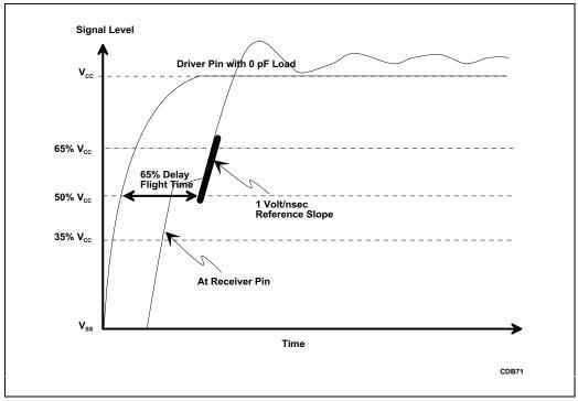
Figure 23-2. Derating the Flight Time
