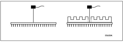
Figure 26-1. Technique For Measuring Tcase
