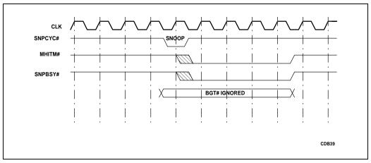
Figure 5-14. Snoop Executing before BGT# is Asserted
