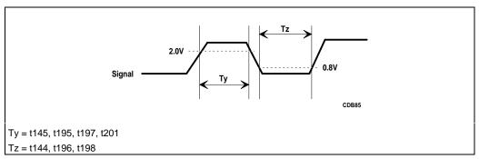
Figure 7-16. Active/Inactive Timings
