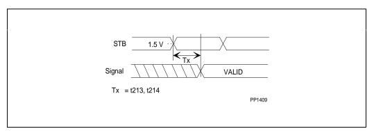
Figure 14-11. Valid Delay Timings From Strobes
