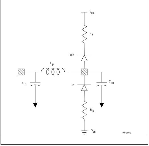
Figure 15-1. Input Buffer Model, Except for Group CPU-CCTL5T
