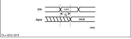
Figure 7-13. Valid Delay Timings from Strobes
