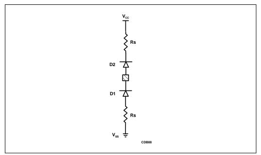
Figure 8-3. Input Diode Model
