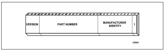
Figure 11-2. Device ID Register
