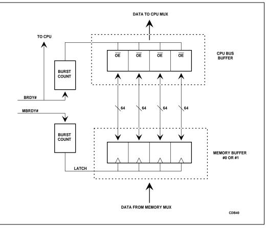
Figure 5-20. 82491 Cache SRAM Read Data Path
