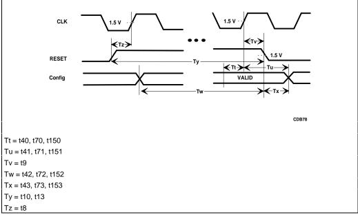
Figure 7-9. Reset and Configuration Timings
