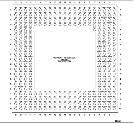
Figure 1-2. Pentium<sup>®</sup> Processor Pinout (Bottom View)
