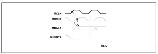
Figure 5-29. Increasing Hold Time of Output Burst Data
