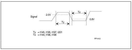
Figure 14-14. Active/Inactive Timings
