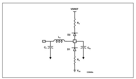
Figure 24-5. Complete 5V Tolerant Input Model Including Diode
