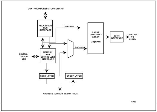
Figure 2-1. 82496 Cache Controller Block Diagram
