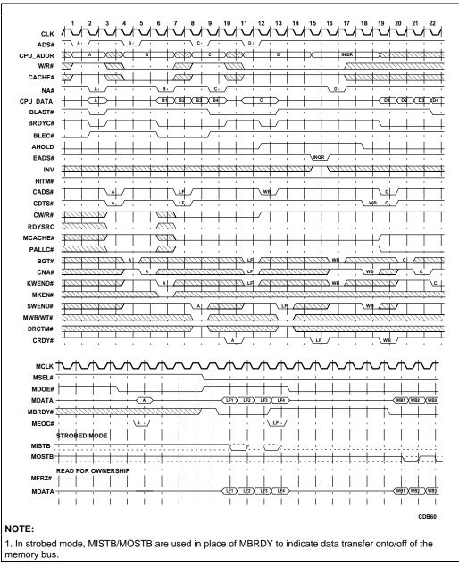
Figure 6-7. Write Miss with Allocation to Modified Line
