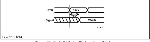
Figure 23-13. Valid Delay Timings from Strobes
