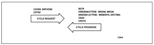
Figure 5-2. Memory Bus Cycle Progress and Attribute Signals
