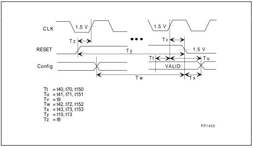
Figure 14-7. Reset and Configuration Timings
