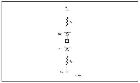
Figure 24-3. Input Diode Model
