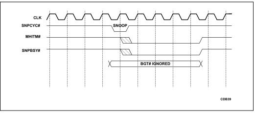
Figure 22-13. Snoop Executing before BGT# Is Asserted
