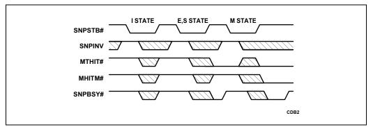
**NOTE:** For E,S states, SNPBSY# is activated because back-invalidation is needed and one is already In progress.
