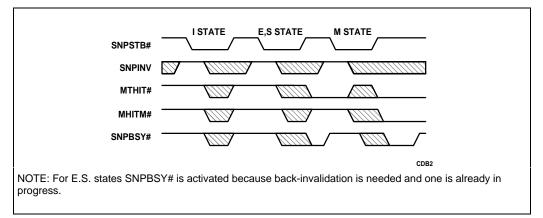
Figure 5-11. Snoops with Invalidation
