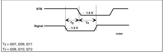
Figure 23-11. Setup and Hold Timings to Strobes
