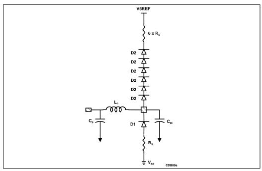
Figure 24-6. Complete 5V Tolerant Input Model Including 6 Diodes
