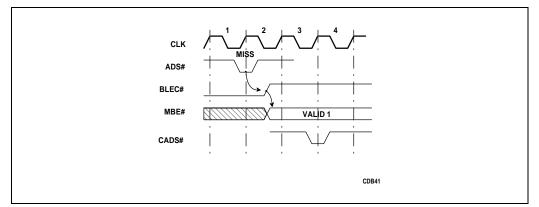
Figure 5-23. BLEC# Deassertion Due to ADS# Assertion
