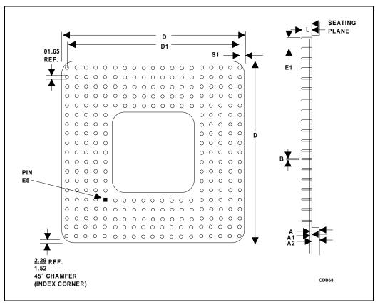
Figure 9-2. 82496 Cache Controller Mechanical Specifications
