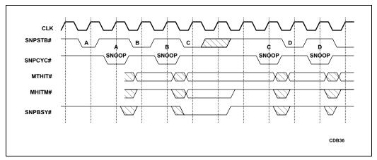
Figure 22-7. Fastest Synchronous Snooping
