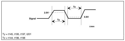
Figure 23-16. Active/Inactive Timings
