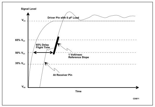
Figure 7-2. Derating the Flight Time
