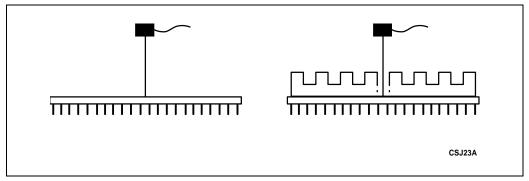
Figure 10-1. Technique for Measuring Tcase
