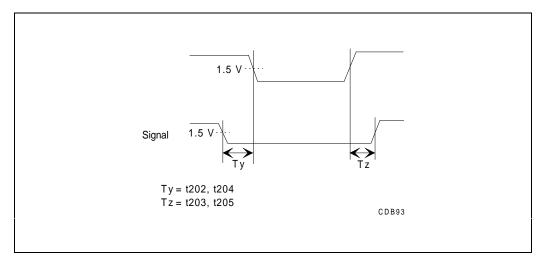
Figure 14-10. Setup and Hold Timings MxST
