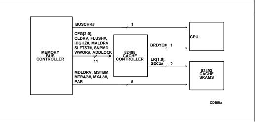
Figure 21-3. CPU-Cache Chip Set Configuration Inputs
