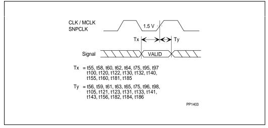
Figure 14-5. Setup and Hold Timings
