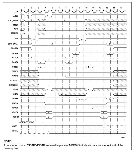
Figure 6-10. I/O Cycles
