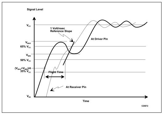
Figure 7-3. In-System Measurement of Flight Time
