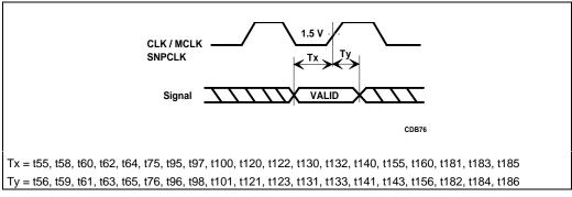
Figure 7-7. Setup and Hold Timings
