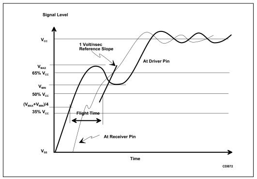
Figure 23-3. In-System Measurement of Flight Time
