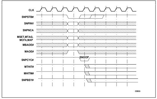
Figure 5-4. Synchronous Snoop Mode
