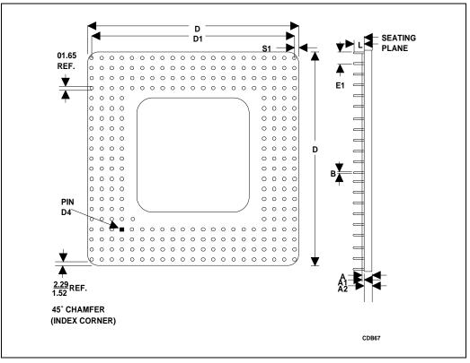
Figure 9-1. Pentium® Processor Mechanical Specifications
