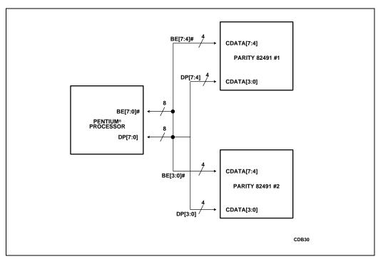
Figure 5-21. Pentium<sup>®</sup> Processor/82491 Cache SRAM Data Parity Connections
