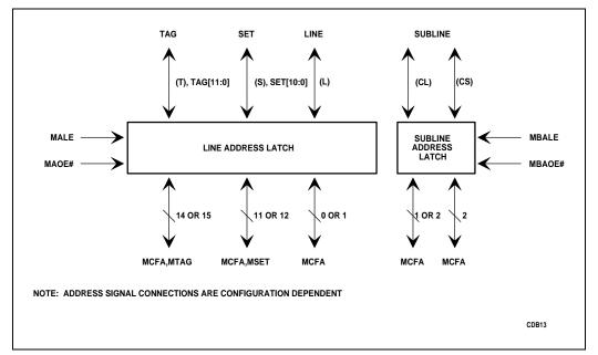
Figure 4-5. Address Latching
