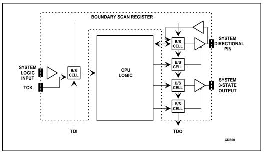
Figure 11-1. Boundary Scan Register Structure of a Component
