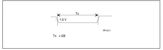
Figure 14-13. Test Reset Timings
