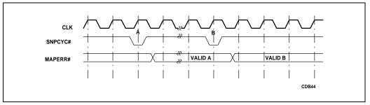
Figure 5-18. MAPERR# Timing for Asynchronous Snoop Modes
