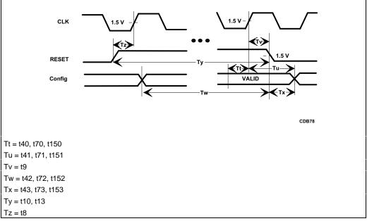
Figure 23-9. Reset and Configuration Timings
