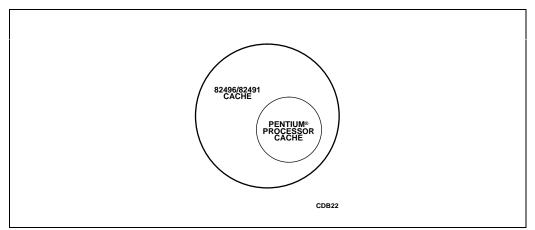
Figure 3-2. Pentium<sup>®</sup> Processor Cache Chip Set Cache Inclusion
