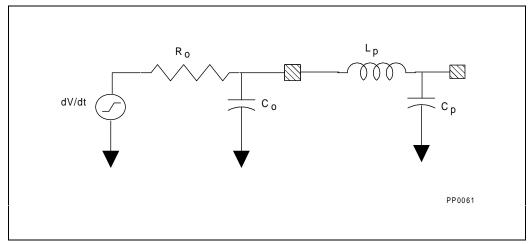
Figure 15-3. First Order Output Buffer Model
