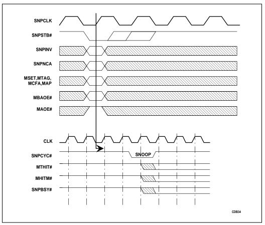
Figure 5-5. Clocked Snoop Mode
