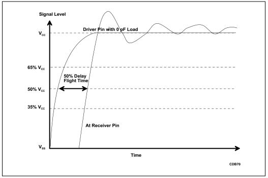
Figure 23-1. Determination of Flight Time
