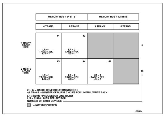
Figure 21-1. 82498 Cache Controller/82493 Cache SRAM Configurations with the Pentium<sup>®</sup> Processor (735\90, 815\100, 1000\120, 1110\133)
