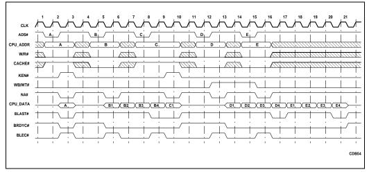
Figure 6-1. Pipe-lined Read Hits
