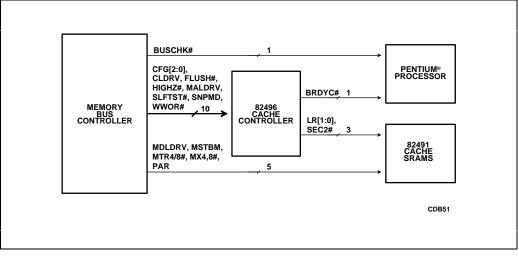
Figure 4-3. CPU-Cache Chip Set Configuration Inputs
