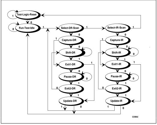
Figure 11-3. TAP Controller State Diagram
