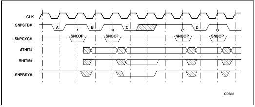
Figure 5-8. Fastest Synchronous Snooping
