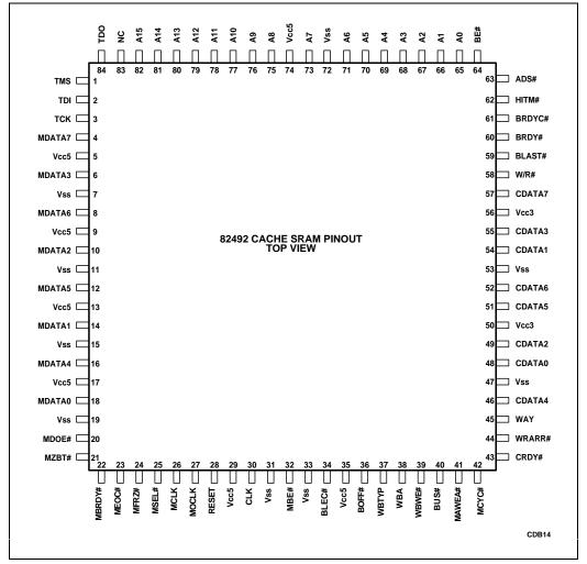
Figure 12-3. 82492 Cache SRAM Memory Pinout (Top View)
