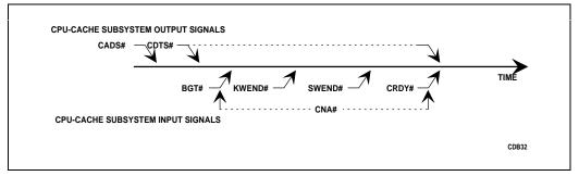
Figure 5-3. Cycle Progress Signals and Responses
