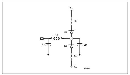
Figure 8-4. Complete Input Model Including Diode
