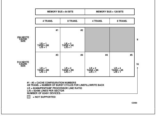
Figure 4-1. 82491 Cache Controller/82491 Cache SRAM Configurations with the Pentium<sup>®</sup> Processor
