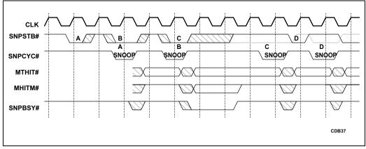
Figure 22-8. Fastest Asynchronous Snooping
