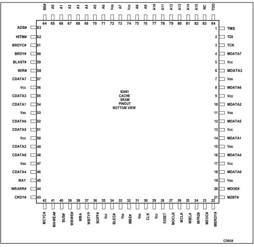
Figure 1-6. 82491 Cache SRAM Pinout (Bottom View)
