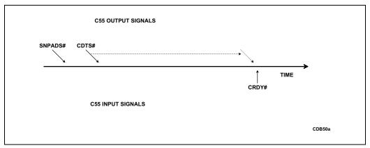
Figure 22-15. Cycle Progress for Snoop Write Back Cycles
