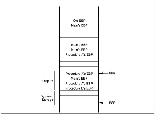
Figure 6-9. Stack Frame after Entering Procedure B
