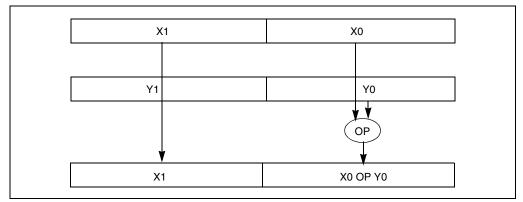
Figure 11-4. Scalar Double-Precision Floating-Point Operations
