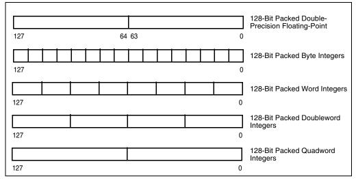
Figure 11-2. Data Types Introduced with the SSE2 Extensions
