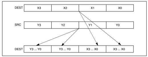
Figure 10-7. SHUFPS Instruction Packed Shuffle Operation
