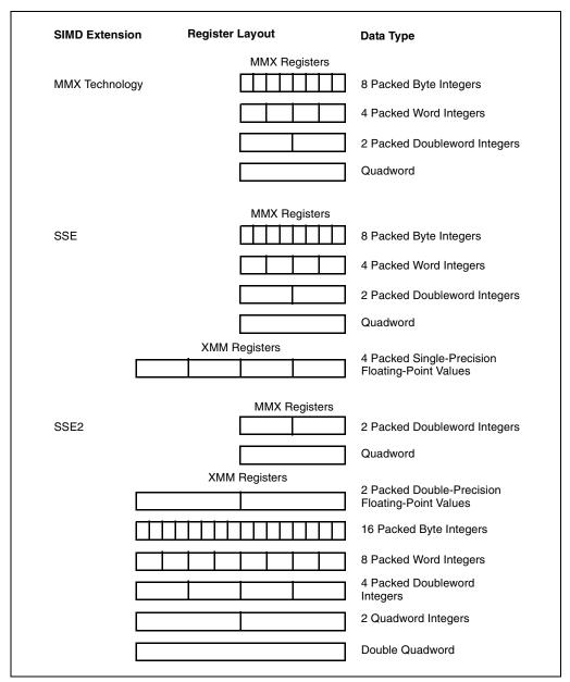
Figure 5-1. SIMD Extensions, Register Layouts, and Data Types
