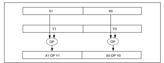
Figure 11-3. Packed Double-Precision Floating-Point Operations
