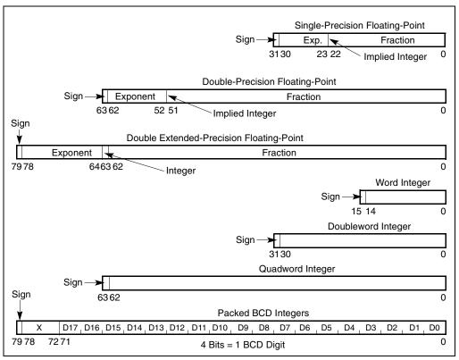
Figure 8-13. x87 FPU Data Type Formats
