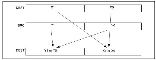
Figure 11-5. SHUFPD Instruction Packed Shuffle Operation
