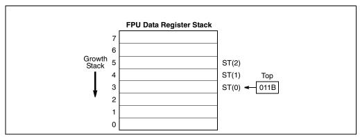
Figure 8-2. x87 FPU Data Register Stack
