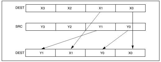
Figure 10-9. UNPCKLPS Instruction Low Unpack and Interleave Operation
