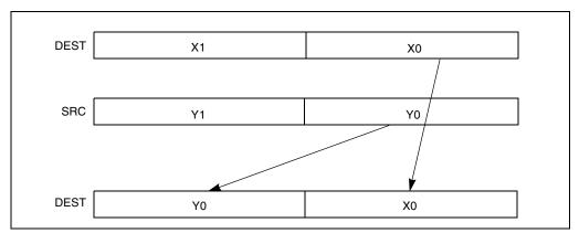
Figure 11-7. UNPCKLPD Instruction Low Unpack and Interleave Operation
