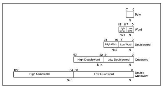
Figure 4-1. Fundamental Data Types
