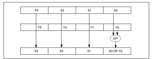
Figure 10-6. Scalar Single-Precision Floating-Point Operation
