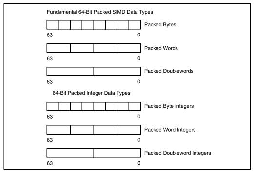
Figure 4-6. 64-Bit Packed SIMD Data Types
