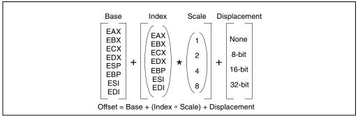
Figure 3-9. Offset (or Effective Address) Computation
