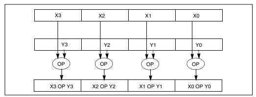
Figure 10-5. Packed Single-Precision Floating-Point Operation
