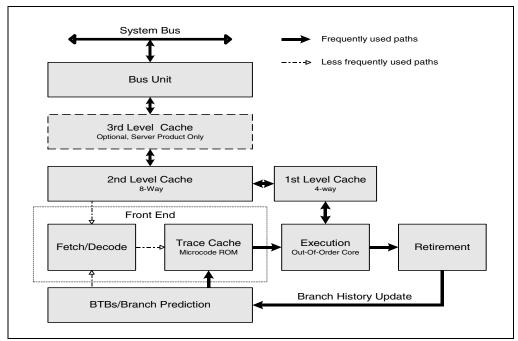
Figure 2-2. The Intel NetBurst Micro-Architecture
