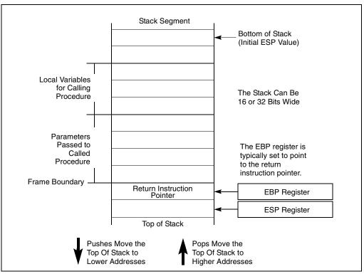
Figure 6-1. Stack Structure
