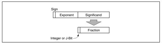
Figure 4-10. Binary Floating-Point Format
