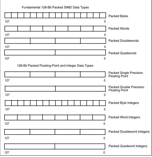
Figure 4-7. 128-Bit Packed SIMD Data Types
