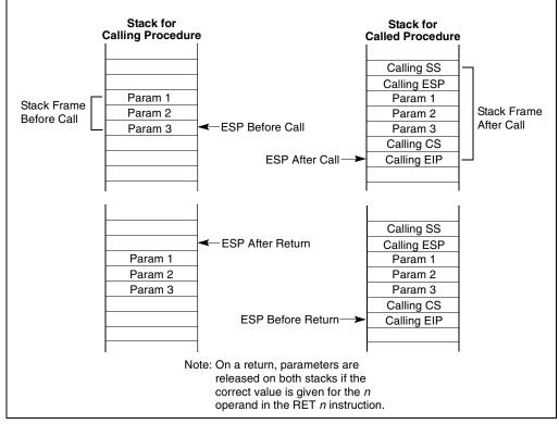
Figure 6-4. Stack Switch on a Call to a Different Privilege Level
