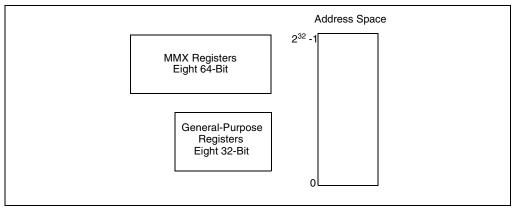
Figure 9-1. MMX Technology Execution Environment
