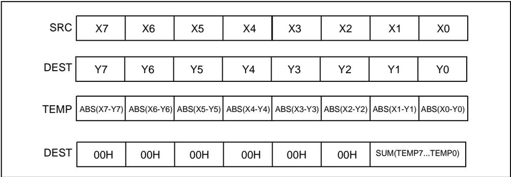
**Figure 3-9. PSADBW Instruction Operation Using 64-bit Operands**
