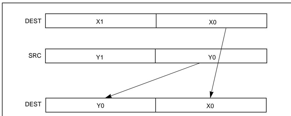
Figure 3-20. UNPCKLPD Instruction Low Unpack and Interleave Operation
