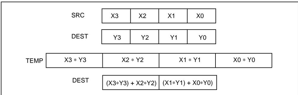
Figure 3-6. PMADDWD Execution Model Using 64-bit Operands
