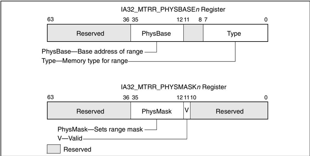
**Figure 10-6. IA32\_MTRR\_PHYSBASE<sub>n</sub> and IA32\_MTRR\_PHYSMASK<sub>n</sub> Variable-Range Register Pair**
