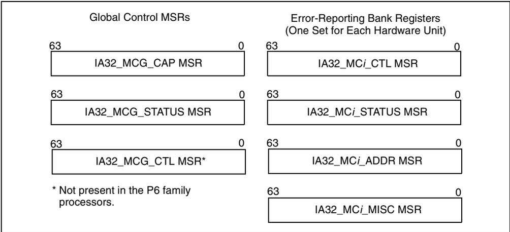
Figure 14-1. Machine-Check MSRs
