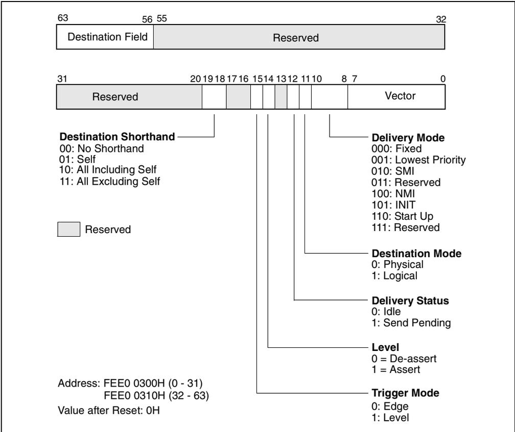
Figure 8-12. Interrupt Command Register (ICR)
