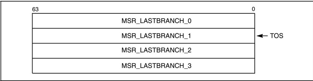
Figure 15-3. LBR MSR Stack Structure
