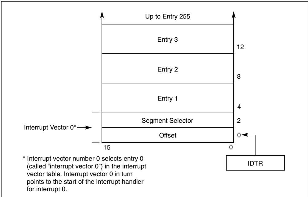
**Figure 16-2. Interrupt Vector Table in Real-Address Mode**
