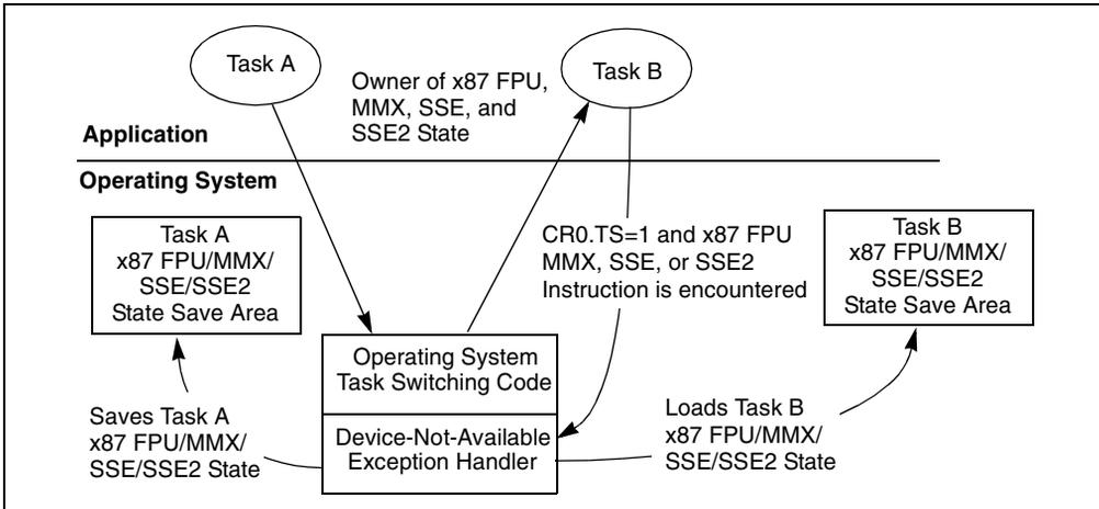
**Figure 12-1. Example of Saving the x87 FPU, MMX, SSE, and SSE2 State During an Operating-System Controlled Task Switch**
