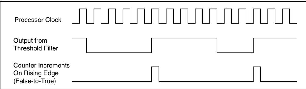
Figure 15-14. Effects of Edge Filtering
