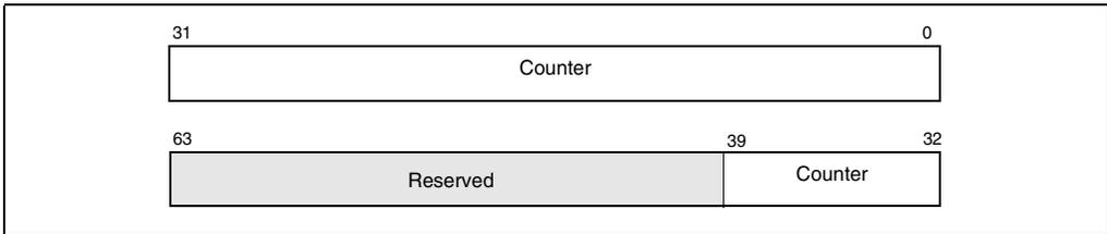
**Figure 15-8. Performance Counter (Pentium 4 and Intel Xeon Processors)**
