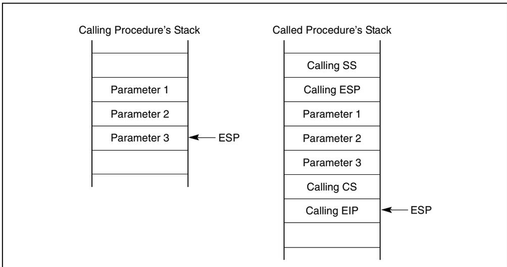
**Figure 4-11. Stack Switching During an Interprivilege-Level Call**
