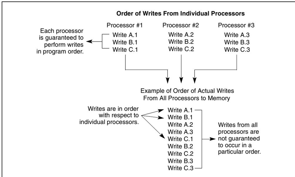
**Figure 7-1. Example of Write Ordering in Multiple-Processor Systems**
