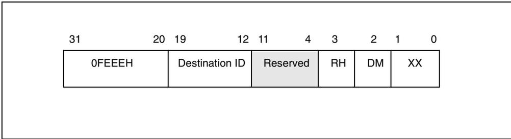
**Figure 8-23. Layout of the MSI Message Address Register**
