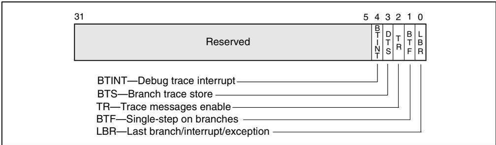
**Figure 15-2. IA32\_DEBUGCTL MSR (Pentium 4 and Intel Xeon Processors)**
