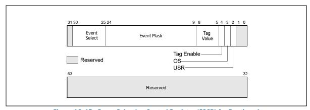
Figure 18-45. Event Selection Control Register (ESCR) for Pentium 4 and Intel Xeon Processors without Intel HT Technology Support
