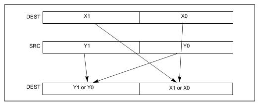
Figure 11-5. SHUFPD Instruction, Packed Shuffle Operation
