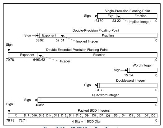
Figure 8-13. x87 FPU Data Type Formats
