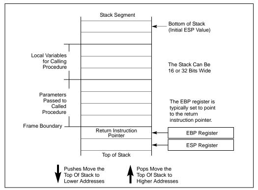
Figure 6-1. Stack Structure
