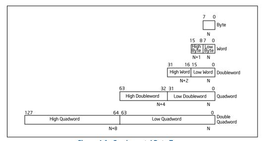
Figure 4-1. Fundamental Data Types
