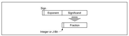
Figure 4-11. Binary Floating-Point Format
