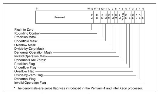
Figure 10-3. MXCSR Control/Status Register
