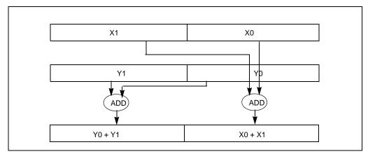
Figure 12-2. Horizontal Data Movement in HADDPD
