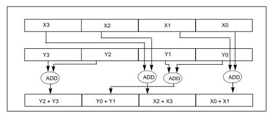
Figure 12-3. Horizontal Data Movement in PHADDD
