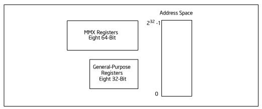
Figure 9-1. MMX Technology Execution Environment
