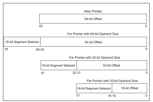
Figure 4-5. Pointers in 64-Bit Mode
