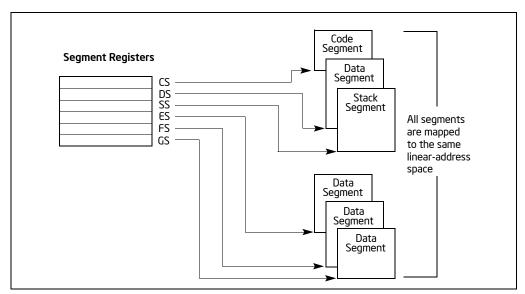
Figure 3-7. Use of Seament Registers in Seamented Memory Model
