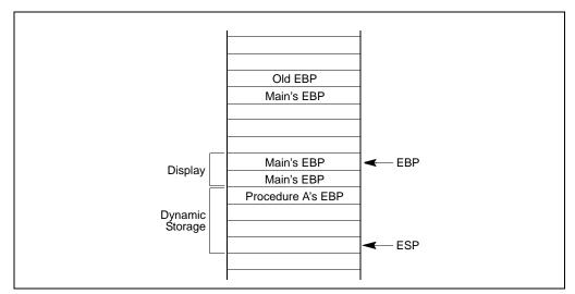
Figure 6-8. Stack Frame After Entering Procedure A
