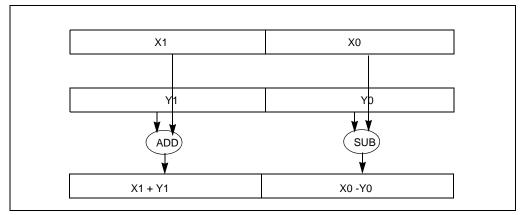
Figure 12-1. Asymmetric Processing in ADDSUBPD
