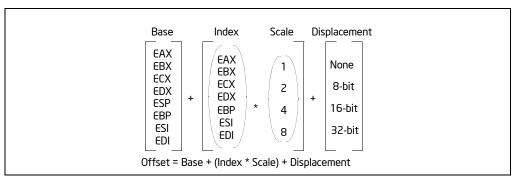
Figure 3-11. Offset (or Effective Address) Computation
