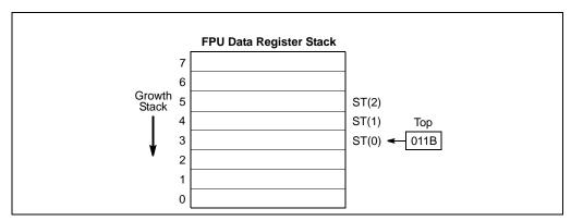
Figure 8-2. x87 FPU Data Register Stack
