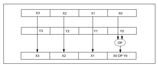
Figure 10-6. Scalar Single-Precision Floating-Point Operation
