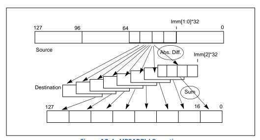
Figure 12-4. MPSADBW Operation
