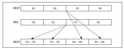
Figure 10-7. SHUFPS Instruction, Packed Shuffle Operation
