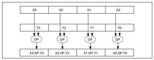
Figure 10-5. Packed Single-Precision Floating-Point Operation
