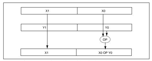
Figure 11-4. Scalar Double-Precision Floating-Point Operations
