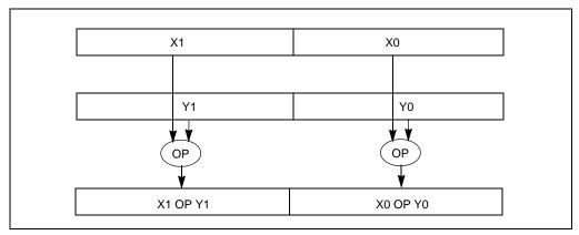
Figure 11-3. Packed Double-Precision Floating-Point Operations
