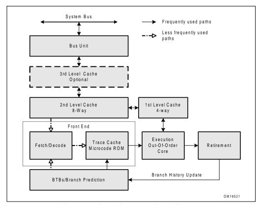
Figure 2-2. The Intel NetBurst Microarchitecture
