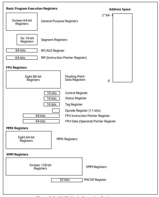
Figure 3-2. 64-Bit Mode Execution Environment
