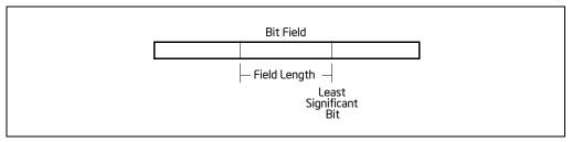
Figure 4-6. Bit Field Data Type
