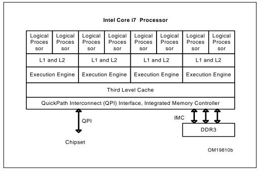
Figure 2-8. Intel Core i7 Processor
