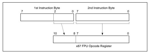
Figure 8-8. Contents of x87 FPU Opcode Registers
