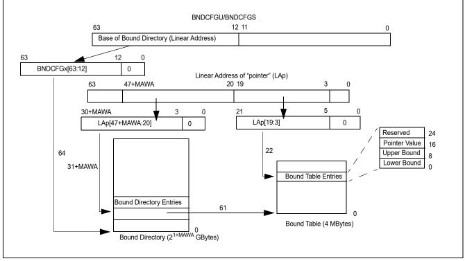
Figure E-4. Bound Paging Structure and Address Translation in 64-Bit Mode
