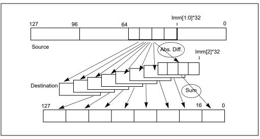
Figure 12-4. MPSADBW Operation
