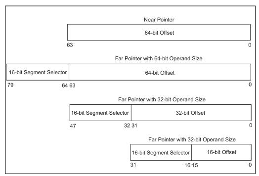
Figure 4-5. Pointers in 64-Bit Mode
