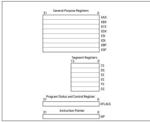
Figure 3-4. General System and Application Programming Registers
