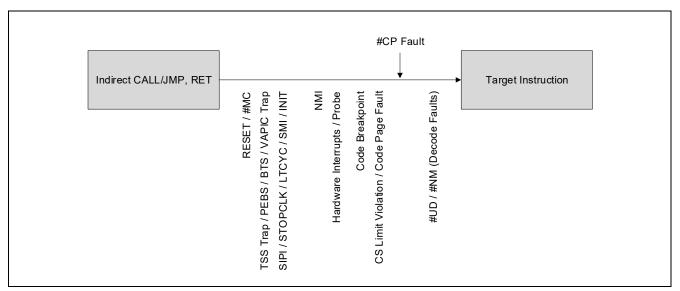
Figure 17-4. Priority of Control Protection Exception on Missing ENDBRANCH
