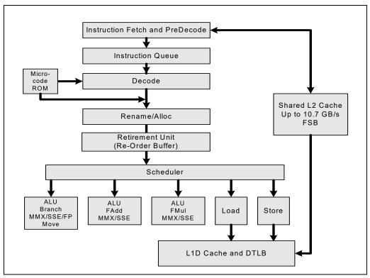
Figure 2-3. The Intel<sup>®</sup> Core<sup>™</sup> Microarchitecture Pipeline Functionality
