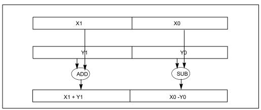
Figure 12-1. Asymmetric Processing in ADDSUBPD
