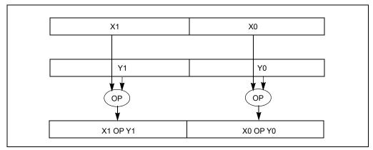
Figure 11-3. Packed Double Precision Floating-Point Operations
