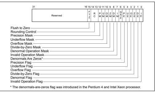
Figure 10-3. MXCSR Control/Status Register
