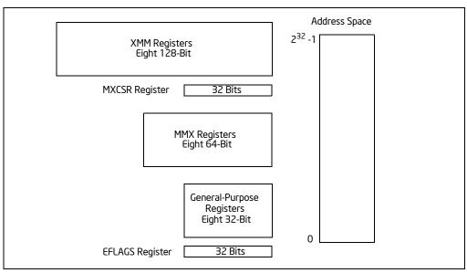
Figure 10-1. Intel® SSE Execution Environment
