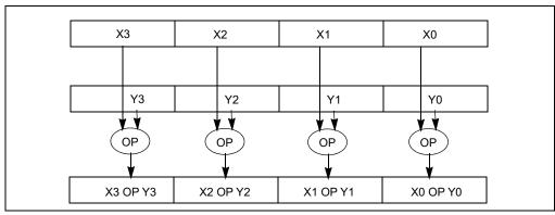
Figure 10-5. Packed Single Precision Floating-Point Operation
