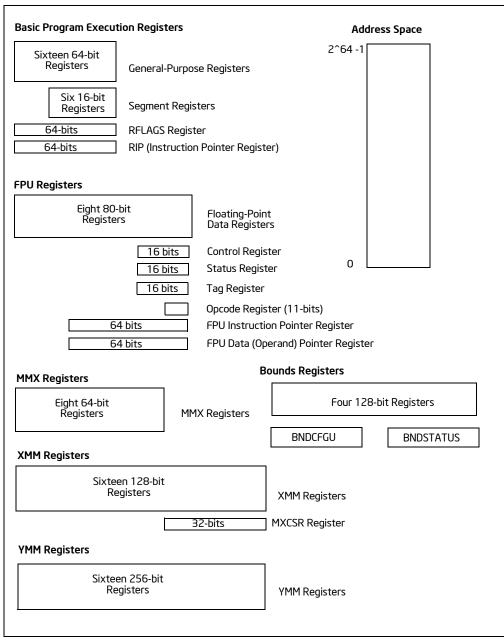
Figure 3-2. 64-Bit Mode Execution Environment
