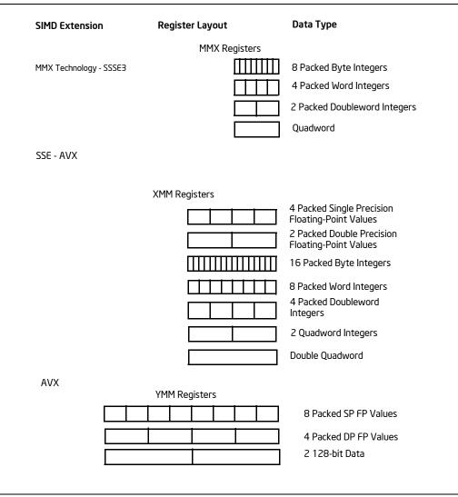
Figure 2-4. SIMD Extensions, Register Layouts, and Data Types
