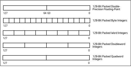
Figure 11-2. Data Types Introduced with Intel<sup>®</sup> SSE2
