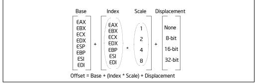
Figure 3-11. Offset (or Effective Address) Computation
