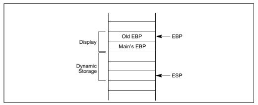
Figure 6-10. Stack Frame After Entering the MAIN Procedure
