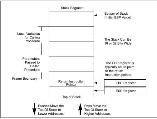
Figure 6-1. Stack Structure
