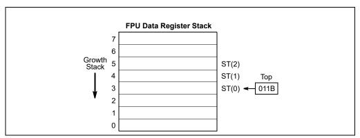
Figure 8-2. x87 FPU Data Register Stack
