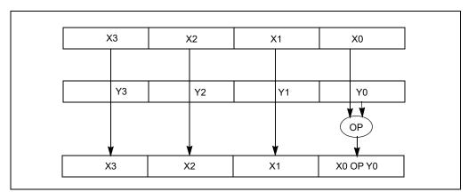
Figure 10-6. Scalar Single Precision Floating-Point Operation
