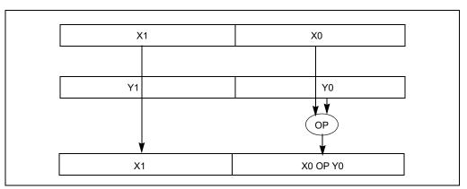
Figure 11-4. Scalar Double Precision Floating-Point Operations
