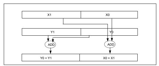
Figure 12-2. Horizontal Data Movement in HADDPD
