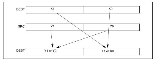
Figure 11-5. SHUFPD Instruction, Packed Shuffle Operation
