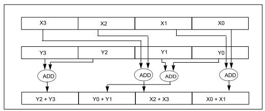
Figure 12-3. Horizontal Data Movement in PHADDD
