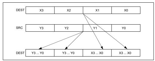
Figure 10-7. SHUFPS Instruction, Packed Shuffle Operation
