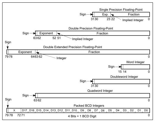
Figure 8-13. x87 FPU Data Type Formats
