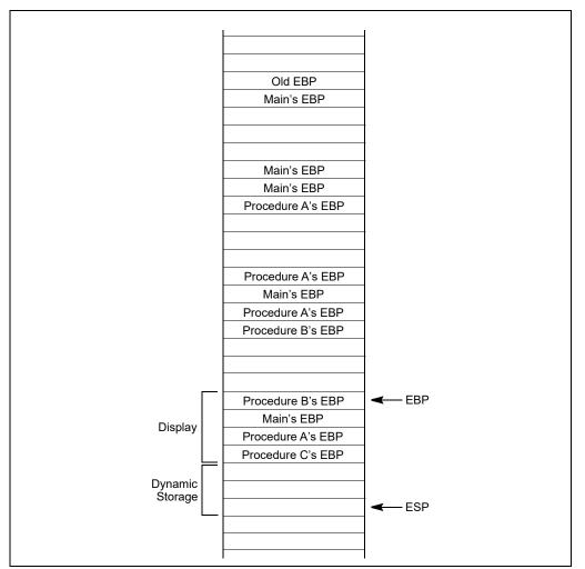
Figure 6-13. Stack Frame After Entering Procedure C
