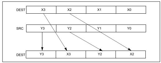
Figure 10-8. UNPCKHPS Instruction, High Unpack and Interleave Operation
