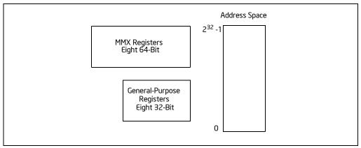
Figure 9-1. MMX Technology Execution Environment
