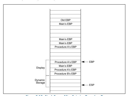
Figure 6-12. Stack Frame After Entering Procedure B
