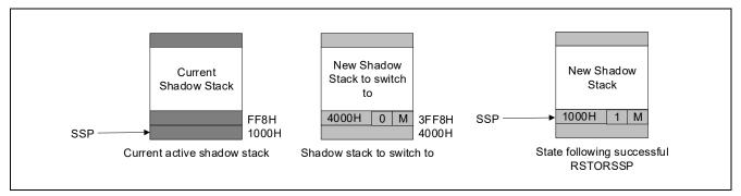
Figure 17-2. RSTORSSP to Switch to New Shadow Stack
