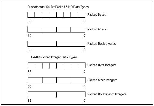
Figure 4-7. 64-Bit Packed SIMD Data Types
