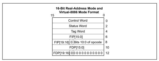
Figure 8-12. Real Mode x87 FPU State Image in Memory, 16-Bit Format
