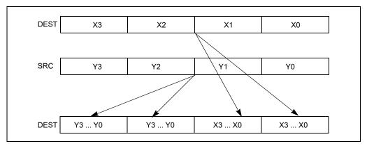
Figure 10-7. SHUFPS Instruction, Packed Shuffle Operation
