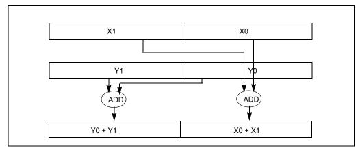
Figure 12-2. Horizontal Data Movement in HADDPD
