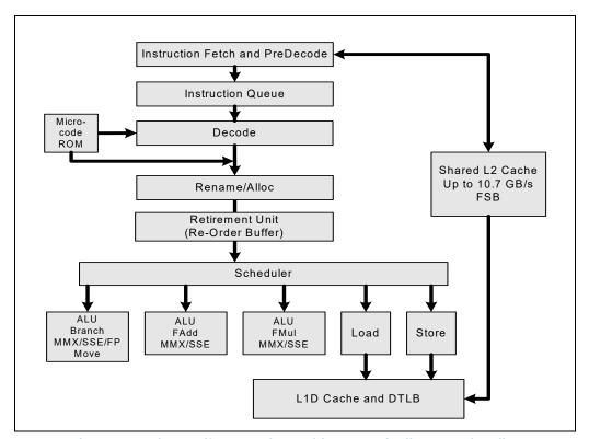
Figure 2-3. The Intel® Core™ Microarchitecture Pipeline Functionality
