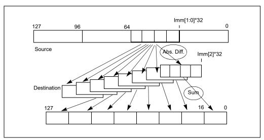
Figure 12-4. MPSADBW Operation
