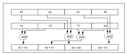
Figure 12-3. Horizontal Data Movement in PHADDD
