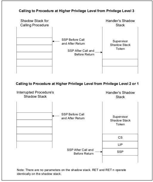
Figure 6-6. Shadow Stack Switch on a Call to a Different Privilege Level
