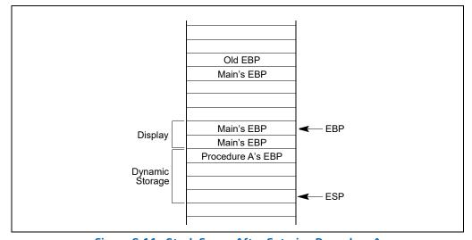
Figure 6-11. Stack Frame After Entering Procedure A
