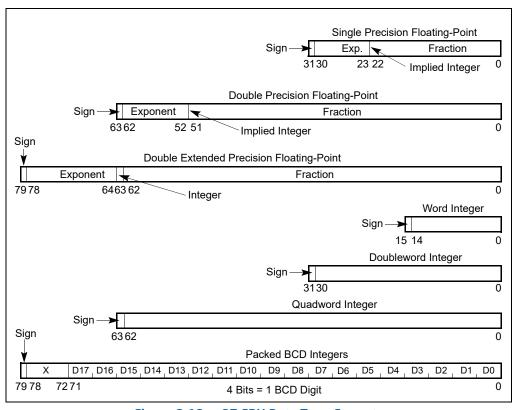
Figure 8-13. x87 FPU Data Type Formats
