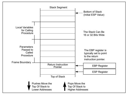
Figure 6-1. Stack Structure
