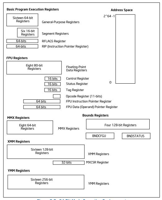
Figure 3-2. 64-Bit Mode Execution Environment
