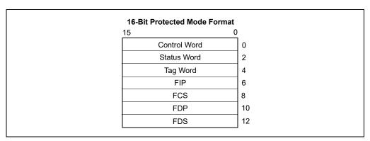
Figure 8-11. Protected Mode x87 FPU State Image in Memory, 16-Bit Format
