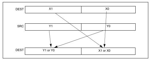
Figure 11-5. SHUFPD Instruction, Packed Shuffle Operation
