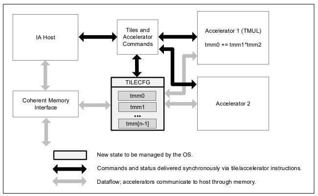
Figure 18-1. Intel® AMX Architecture
