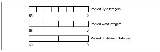
Figure 9-3. Data Types Introduced with the MMX Technology
