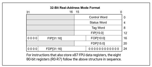
Figure 8-10. Real Mode x87 FPU State Image in Memory, 32-Bit Format
