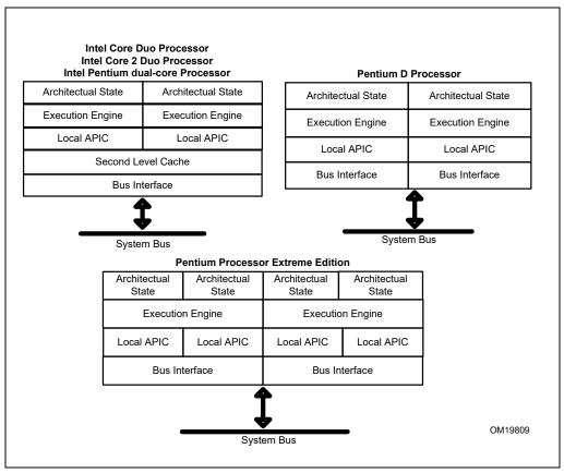
Figure 2-6. Intel 64 and IA-32 Processors that Support Dual-Core
