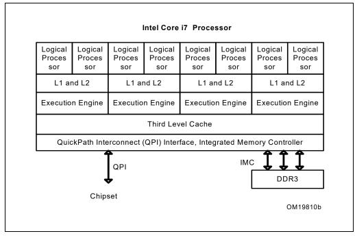
Figure 2-8. Intel® Core™ i7 Processor
