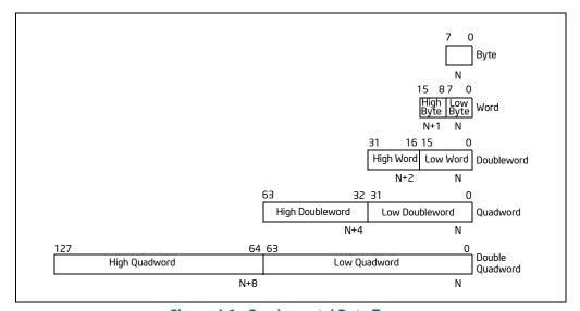
Figure 4-1. Fundamental Data Types
