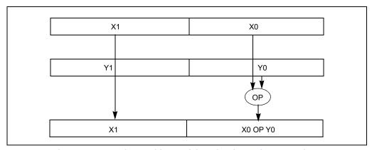
Figure 11-4. Scalar Double Precision Floating-Point Operations
