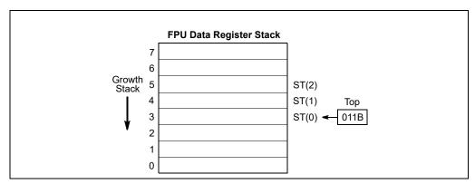
Figure 8-2. x87 FPU Data Register Stack
