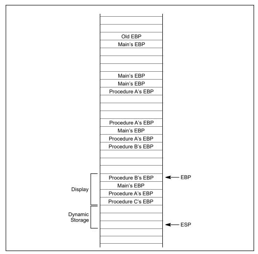
Figure 6-13. Stack Frame After Entering Procedure C
