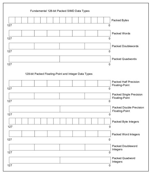
Figure 4-8. 128-Bit Packed SIMD Data Types
