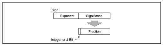
Figure 4-11. Binary Floating-Point Format
