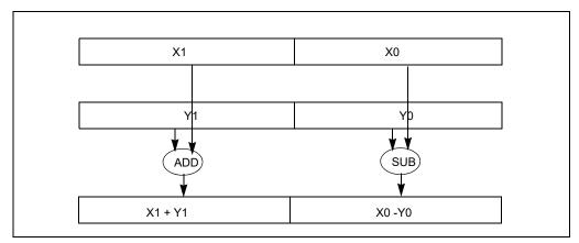
Figure 12-1. Asymmetric Processing in ADDSUBPD
