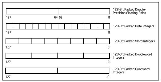
Figure 11-2. Data Types Introduced with Intel® SSE2
