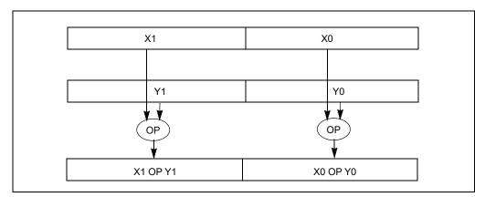
Figure 11-3. Packed Double Precision Floating-Point Operations
