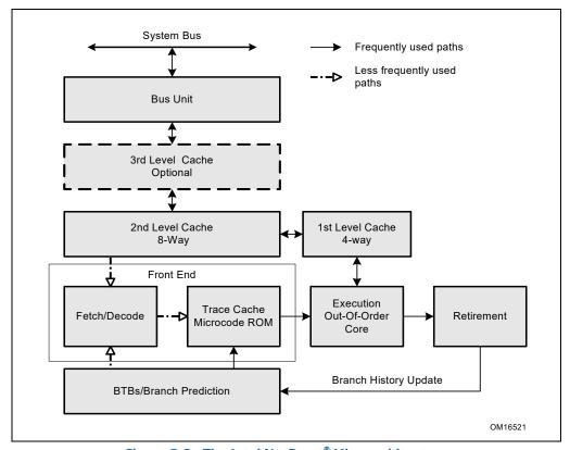
Figure 2-2. The Intel NetBurst® Microarchitecture
