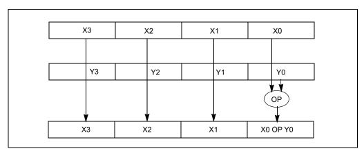
Figure 10-6. Scalar Single Precision Floating-Point Operation
