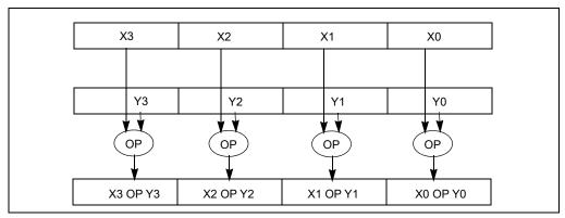
Figure 10-5. Packed Single Precision Floating-Point Operation
