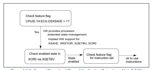
Figure 14-2. General Procedural Flow of Application Detection of Intel® AVX
