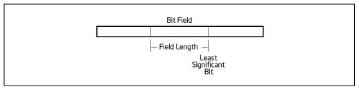
Figure 4-6. Bit Field Data Type
