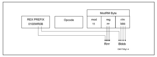
Figure 2-4. Register-Register Addressing (No Memory Operand); REX.X Not Used
