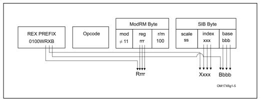
Figure 2-5. Memory Addressing With a SIB Byte
