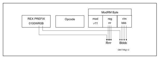
Figure 2-3. Memory Addressing Without an SIB Byte; REX.X Not Used
