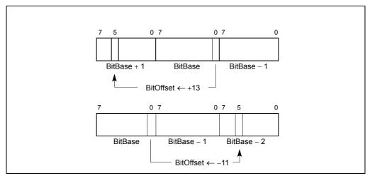
Figure 3-2. Memory Bit Indexing
