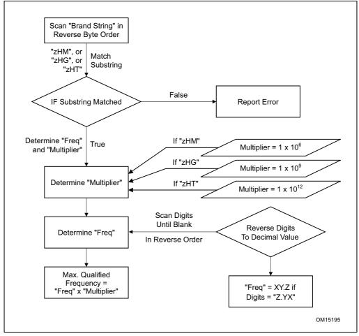
Figure 3-10. Algorithm for Extracting Maximum Processor Frequency
