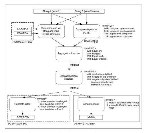
Figure 3-3. Operation of PCMPSTRx and PCMPESTRx
