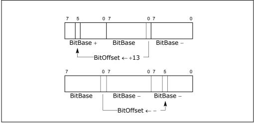
Figure 3-2. Memory Bit Indexing
