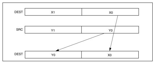
Figure 4-16. UNPCKLPD Instruction Low Unpack and Interleave Operation
