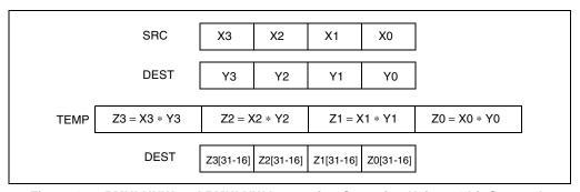
Figure 4-3. PMULHUW and PMULHW Instruction Operation Using 64-bit Operands
