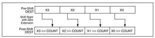
Figure 4-9. PSRLW, PSRLD, and PSRLQ Instruction Operation Using 64-bit Operand
