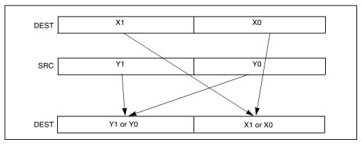
Figure 4-12. SHUFPD Shuffle Operation
