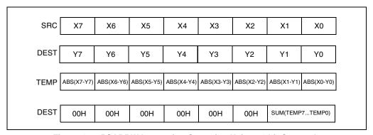
Figure 4-5. PSADBW Instruction Operation Using 64-bit Operands
