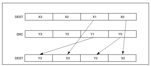
Figure 4-17. UNPCKLPS Instruction Low Unpack and Interleave Operation
