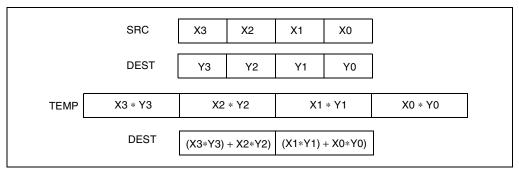
Figure 4-2. PMADDWD Execution Model Using 64-bit Operands
