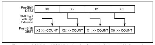
Figure 4-8. PSRAW and PSRAD Instruction Operation Using a 64-bit Operand
