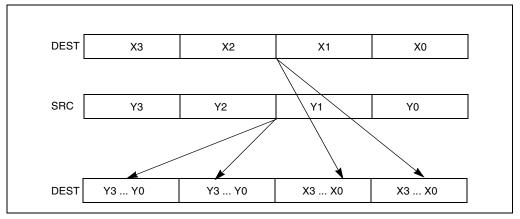
Figure 4-13. SHUFPS Shuffle Operation
