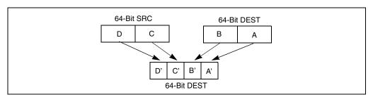
Figure 4-1. Operation of the PACKSSDW Instruction Using 64-bit Operands.
