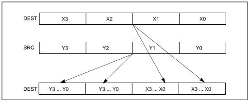
Figure 4-14. SHUFPS Shuffle Operation
