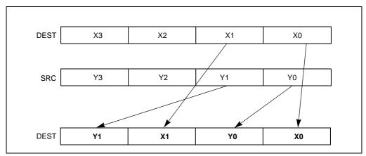
Figure 4-18. UNPCKLPS Instruction Low Unpack and Interleave Operation
