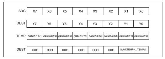
Figure 4-5. PSADBW Instruction Operation Using 64-bit Operands
