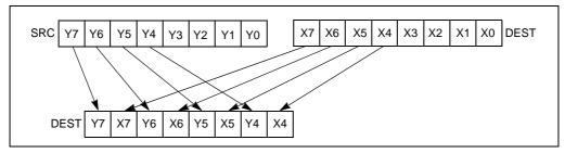
Figure 4-11. PUNPCKHBW Instruction Operation Using 64-bit Operands
