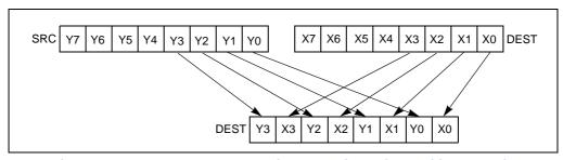
Figure 4-12. PUNPCKLBW Instruction Operation Using 64-bit Operands
