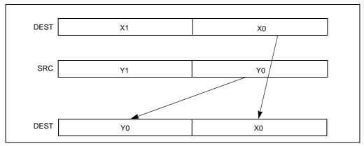
Figure 4-17. UNPCKLPD Instruction Low Unpack and Interleave Operation
