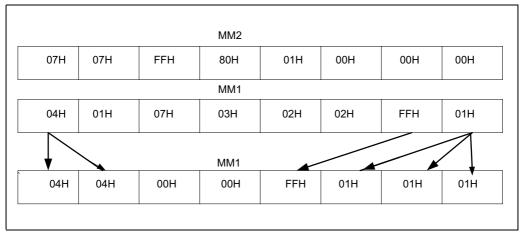
Figure 4-6. PSHUB with 64-Bit Operands
