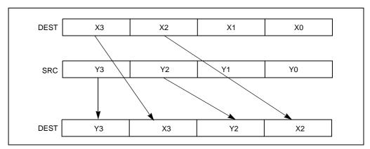
Figure 4-16. UNPCKHPS Instruction High Unpack and Interleave Operation
