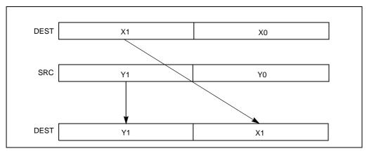
Figure 4-15. UNPCKHPD Instruction High Unpack and Interleave Operation
