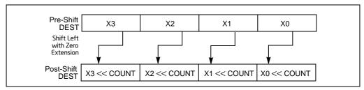
Figure 4-8. PSLLW, PSLLD, and PSLLQ Instruction Operation Using 64-bit Operand
