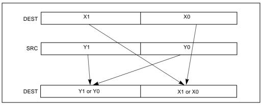
Figure 4-13. SHUFPD Shuffle Operation
