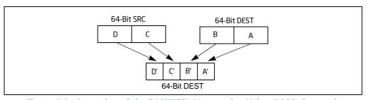
Figure 4-1. Operation of the PACKSSDW Instruction Using 64-bit Operands
