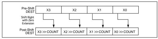
Figure 4-10. PSRLW, PSRLD, and PSRLQ Instruction Operation Using 64-bit Operand
