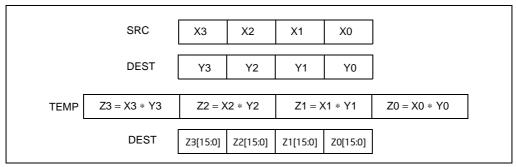
Figure 4-4. PMULLU Instruction Operation Using 64-bit Operands
