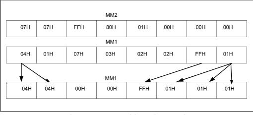
Figure 4-6. PSHUB with 64-Bit Operands
