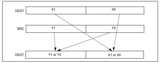
Figure 4-14. SHUFPD Shuffle Operation
