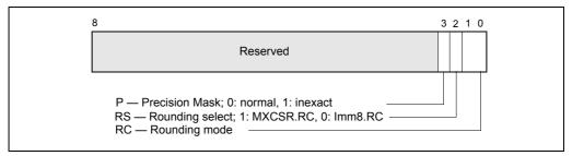
Figure 4-13. Bit Control Fields of Immediate Byte for ROUNDxx Instruction
