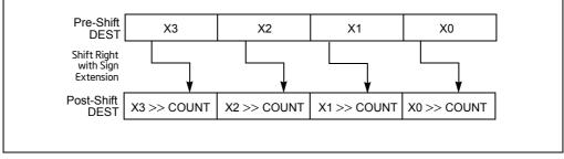
Figure 4-9. PSRAW and PSRAD Instruction Operation Using a 64-bit Operand
