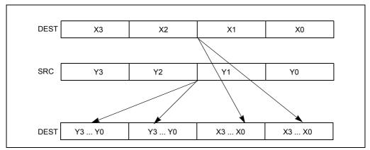
Figure 4-15. SHUFPS Shuffle Operation
