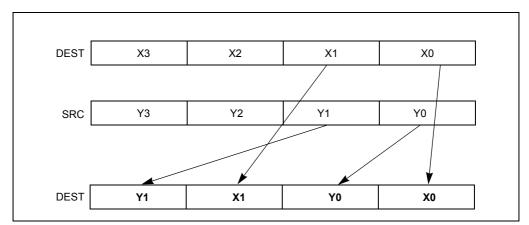
Figure 4-19. UNPCKLPS Instruction Low Unpack and Interleave Operation
