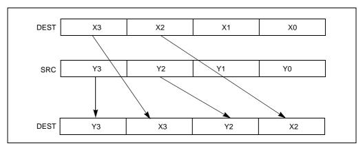
Figure 4-18. UNPCKHPS Instruction High Unpack and Interleave Operation
