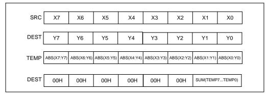
Figure 4-6. PSADBW Instruction Operation Using 64-bit Operands
