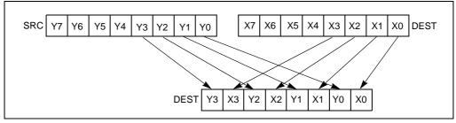
Figure 4-13. PUNPCKLBW Instruction Operation Using 64-bit Operands
