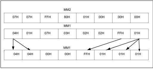
Figure 4-7. PSHUB with 64-Bit Operands
