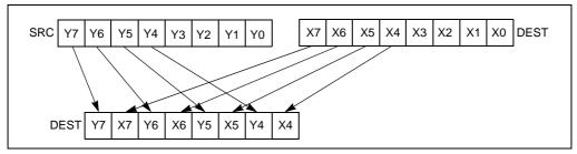
Figure 4-12. PUNPCKHBW Instruction Operation Using 64-bit Operands
