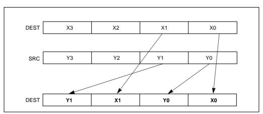
Figure 4-20. UNPCKLPS Instruction Low Unpack and Interleave Operation
