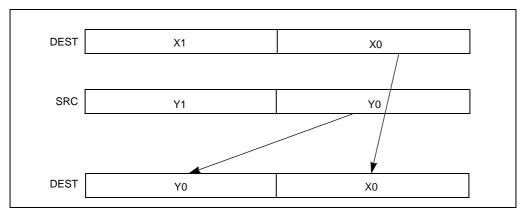
Figure 4-19. UNPCKLPD Instruction Low Unpack and Interleave Operation
