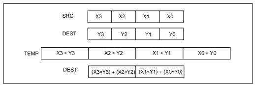
Figure 4-3. PMADDWD Execution Model Using 64-bit Operands
