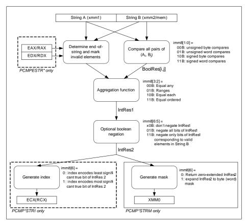
Figure 4-1. Operation of PCMPSTRx and PCMPESTRx
