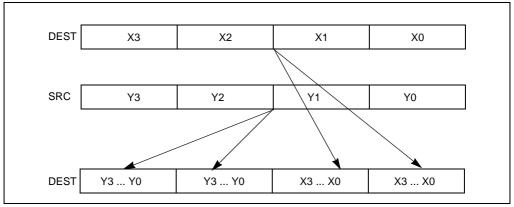
Figure 4-16. SHUFPS Shuffle Operation
