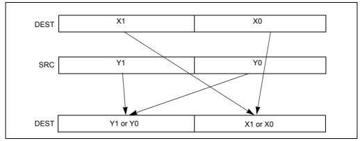
Figure 4-18. SHUFPD Shuffle Operation
