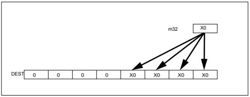
Figure 4-25. VBROADCASTSS Operation (128-bit version)
