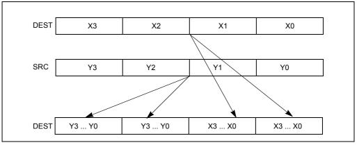
Figure 4-19. SHUFPS Shuffle Operation
