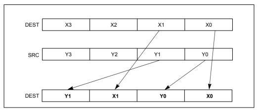
Figure 4-23. UNPCKLPS Instruction Low Unpack and Interleave Operation
