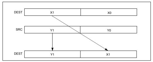
Figure 4-20. UNPCKHPD Instruction High Unpack and Interleave Operation
