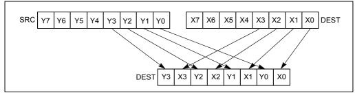
Figure 4-16. PUNPCKLBW Instruction Operation Using 64-bit Operands
