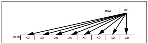
Figure 4-24. VBROADCASTSS Operation (VEX.256 encoded version)
