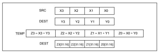
Figure 4-7. PMULHUW and PMULHW Instruction Operation Using 64-bit Operands
