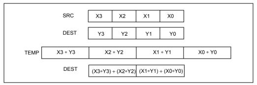
Figure 4-6. PMADDWD Execution Model Using 64-bit Operands
