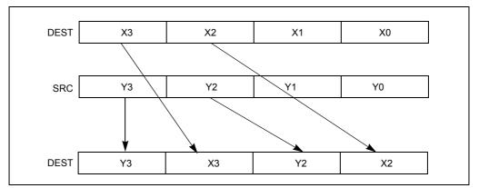
Figure 4-21. UNPCKHPS Instruction High Unpack and Interleave Operation
