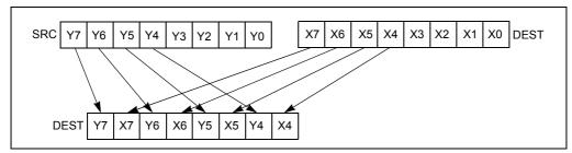
Figure 4-15. PUNPCKHBW Instruction Operation Using 64-bit Operands
