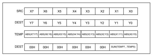
Figure 4-9. PSADBW Instruction Operation Using 64-bit Operands
