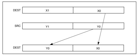
Figure 4-22. UNPCKLPD Instruction Low Unpack and Interleave Operation
