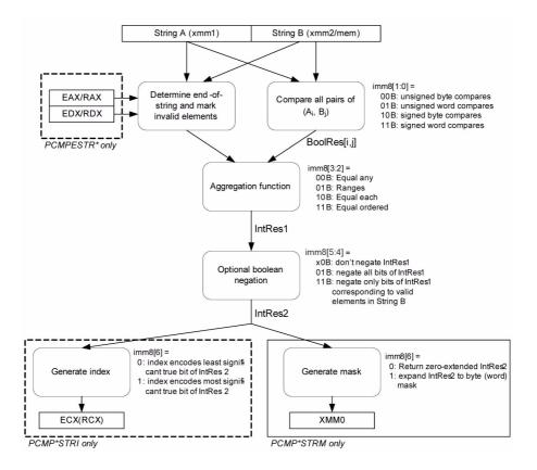
Figure 4-1. Operation of PCMPSTRx and PCMPESTRx
