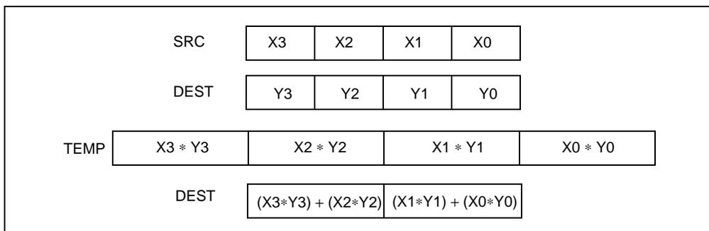
Figure 4-7. PMADDWD Execution Model Using 64-bit Operands
