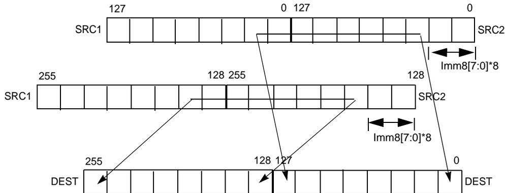
Figure 4-3. 256-bit VPALIGN Instruction Operation
