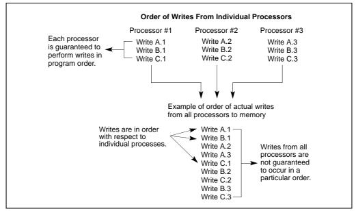
Figure 7-1. Example of Write Ordering in Multiple-Processor Systems
