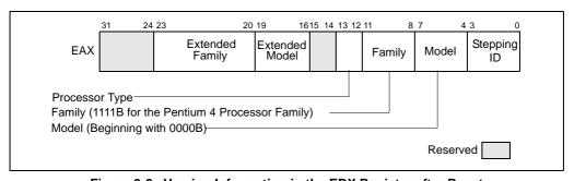
Figure 9-2. Version Information in the EDX Register after Reset
