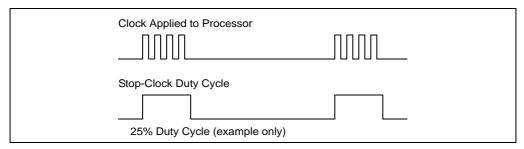
Figure 13-2. Processor Modulation Through Stop-Clock Mechanism
