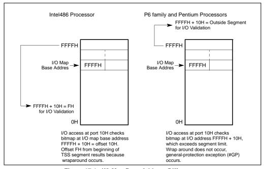
Figure 17-1. I/O Map Base Address Differences
