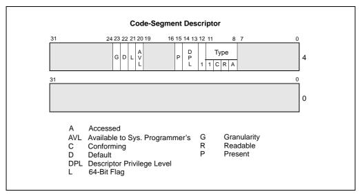
Figure 4-2. Descriptor Fields with Flags used in IA-32e Mode
