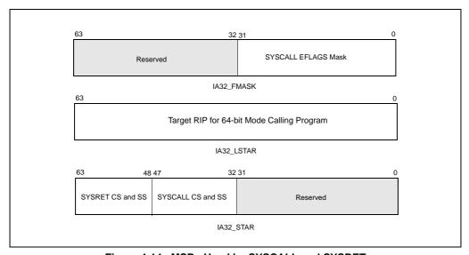
Figure 4-14. MSRs Used by SYSCALL and SYSRET
