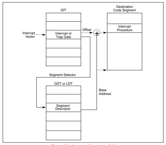
Figure 5-3. Interrupt Procedure Call
