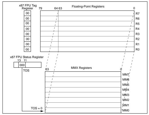
Figure 11-1. Mapping of MMX Registers to Floating-Point Registers
