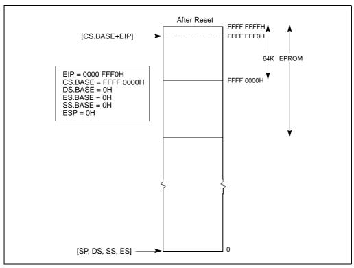
Figure 9-3. Processor State After Reset
