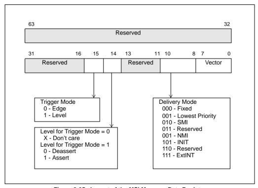
Figure 8-25. Layout of the MSI Message Data Register
