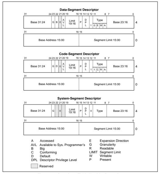
Figure 4-1. Descriptor Fields Used for Protection
