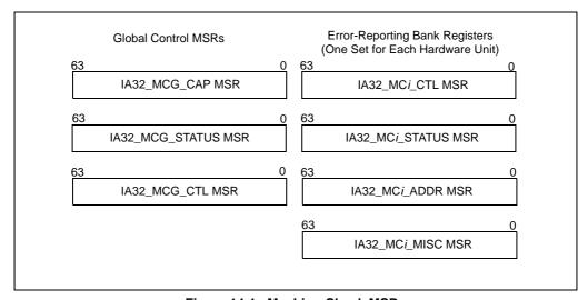
Figure 14-1. Machine-Check MSRs
