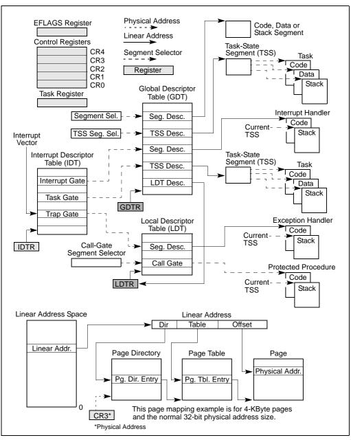
Figure 2-1. IA-32 System-Level Registers and Data Structures
