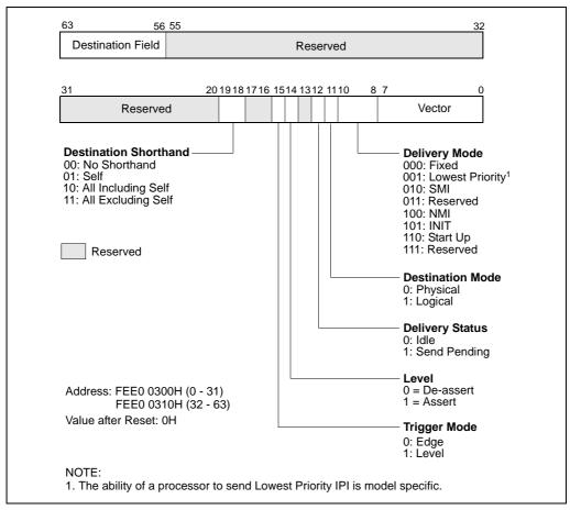
Figure 8-12. Interrupt Command Register (ICR)
