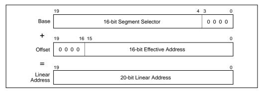
Figure 15-1. Real-Address Mode Address Translation
