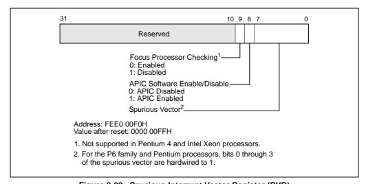
Figure 8-23. Spurious-Interrupt Vector Register (SVR)
