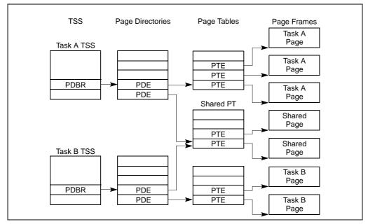
Figure 6-9. Overlapping Linear-to-Physical Mappings
