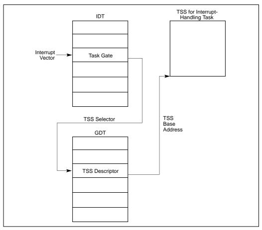
Figure 5-5. Interrupt Task Switch
