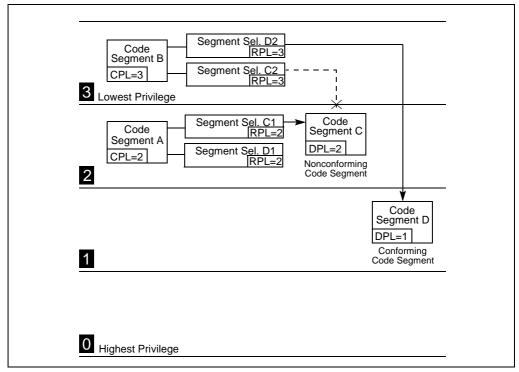
Figure 4-7. Examples of Accessing Conforming and Nonconforming Code Segments
