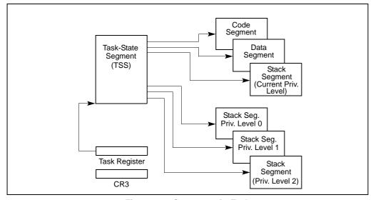
Figure 6-1. Structure of a Task
