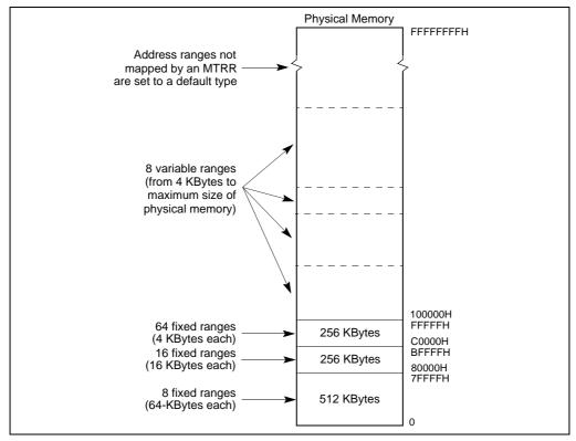
Figure 10-3. Mapping Physical Memory With MTRRs
