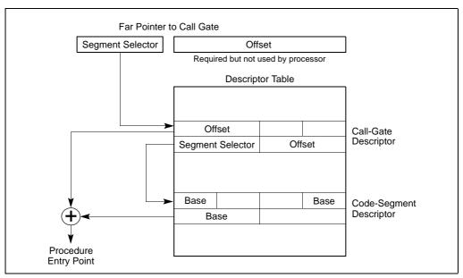
Figure 4-10. Call-Gate Mechanism
