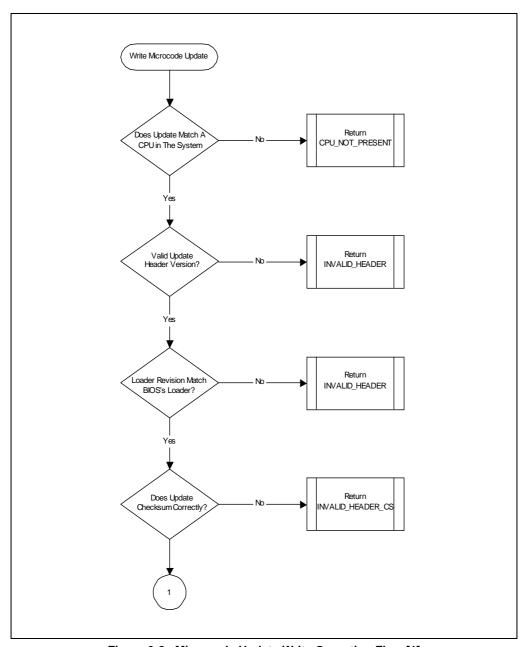
Figure 9-8. Microcode Update Write Operation Flow [1]
