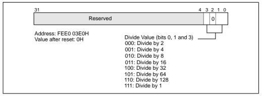
Figure 8-10. Divide Configuration Register
