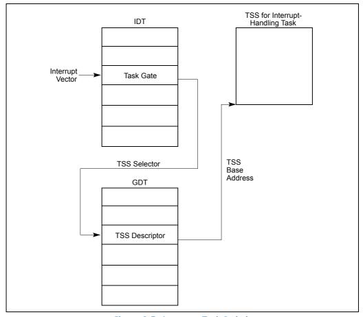
Figure 6-5. Interrupt Task Switch
