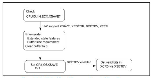
Figure 13-3. OS Enabling of Processor Extended State Support
