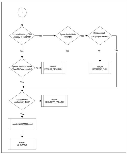
Figure 9-9. Microcode Update Write Operation Flow [2]
