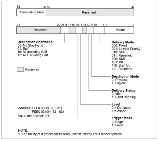
Figure 10-12. Interrupt Command Register (ICR)
