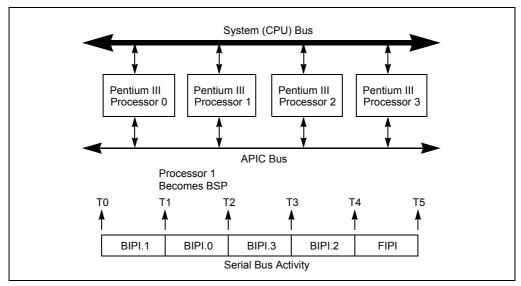
Figure 8-1. MP System With Multiple Pentium III Processors
