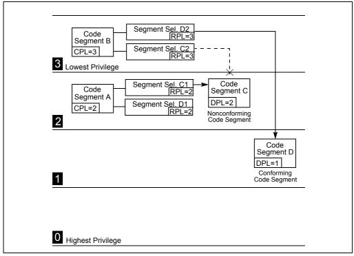
Figure 5-7. Examples of Accessing Conforming and Nonconforming Code Segments
