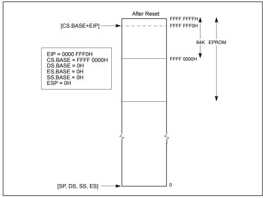
Figure 9-3. Processor State After Reset
