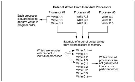
Figure 8-1. Example of Write Ordering in Multiple-Processor Systems
