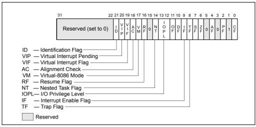
Figure 2-4. System Flags in the EFLAGS Register
