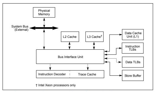
Figure 11-1. Cache Structure of the Pentium 4 and Intel Xeon Processors
