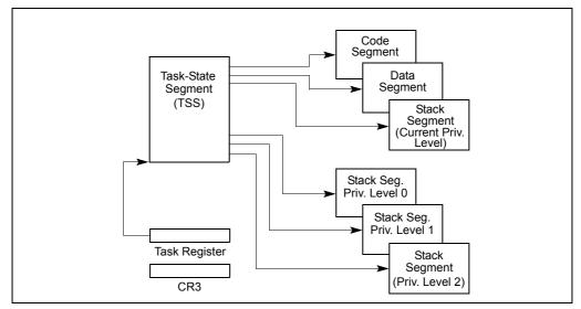
Figure 7-1. Structure of a Task
