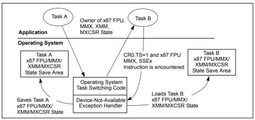
Figure 13-1. Example of Saving the x87 FPU, MMX, SSE, SSE2, SSE3, and SSSE3
