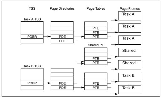
Figure 7-9. Overlapping Linear-to-Physical Mappings
