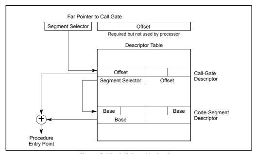
Figure 5-10. Call-Gate Mechanism
