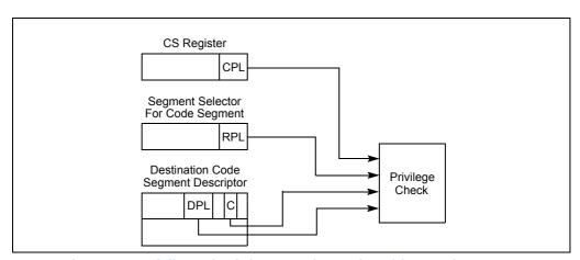
Figure 5-6. Privilege Check for Control Transfer Without Using a Gate
