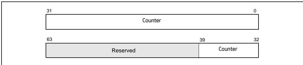
**Figure 30-24. Performance Counter (Pentium 4 and Intel Xeon Processors)**
