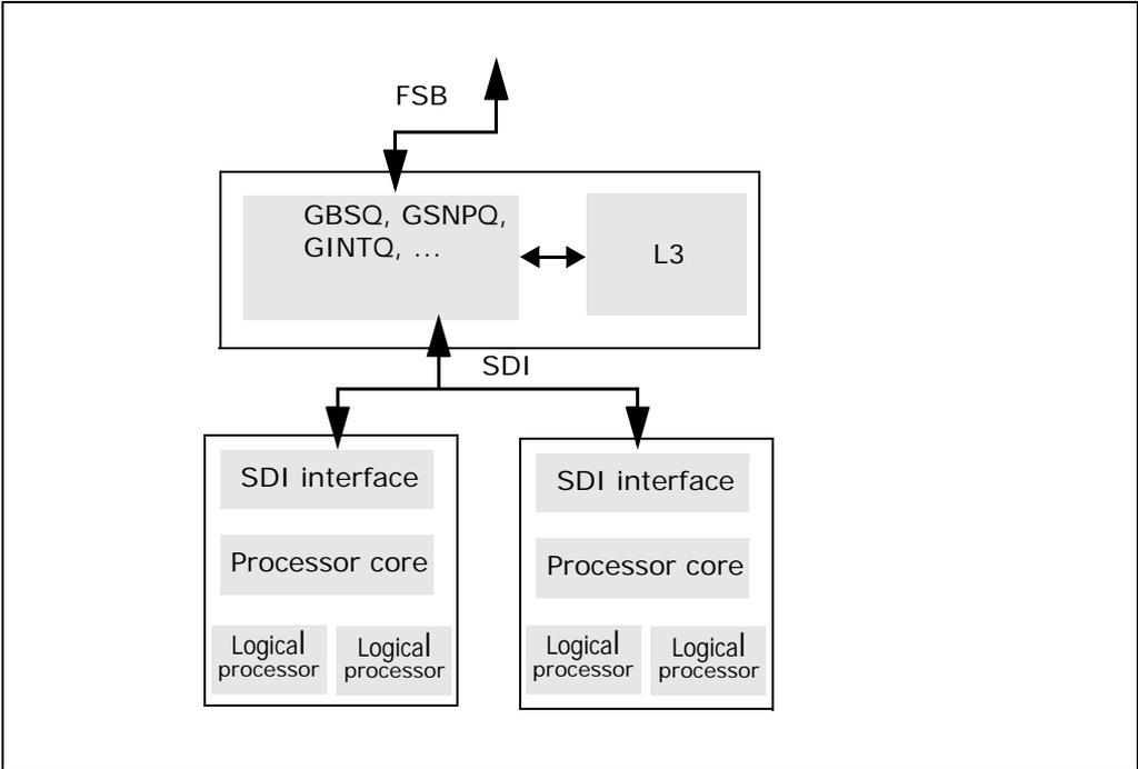
Figure 30-36. Block Diagram of Intel Xeon Processor 7100 Series
