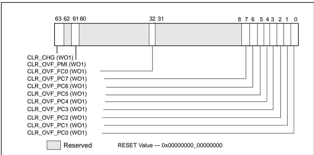
Figure 30-19. Layout of MSR\_UNCORE\_PERF\_GLOBAL\_OVF\_CTRL MSR
