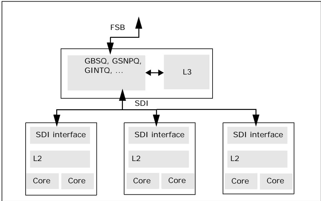
**Figure 30-35. Block Diagram of Intel Xeon Processor 7400 Series**
