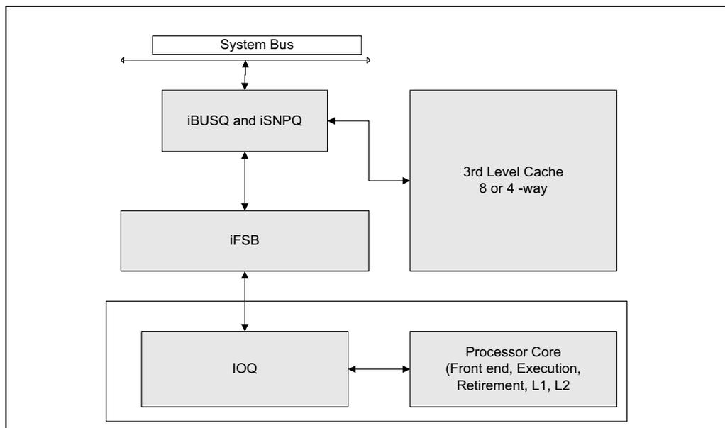
**Figure 30-30. Block Diagram of 64-bit Intel Xeon Processor MP with 8-MByte L3**
