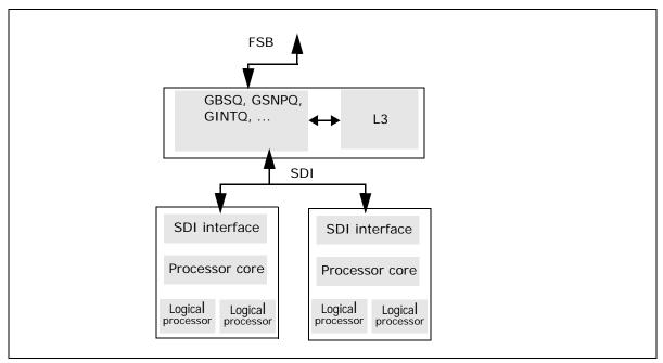
Figure 18-48. Block Diagram of Intel Xeon Processor 7100 Series
