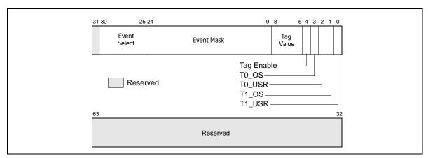
Figure 18-39. Event Selection Control Register (ESCR) for the Pentium 4 Processor, Intel Xeon Processor and Intel Xeon Processor MP Supporting Hyper-Threading Technology
