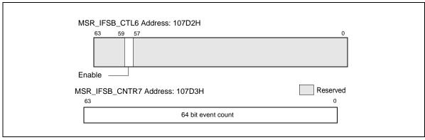
Figure 18-46. MSR\_IFSB\_CTL6, Address: 107D2H; MSR\_IFSB\_CNTR7, Address: 107D3H
