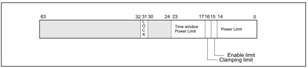
Figure 14-21. MSR PPO POWER LIMIT/MSR PP1 POWER LIMIT Register
