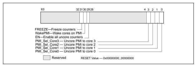
Figure 18-33. Layout of MSR\_UNC\_PERF\_GLOBAL\_CTRL MSR for Uncore
