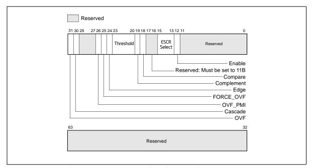
Figure 18-37. Counter Configuration Control Register (CCCR)
