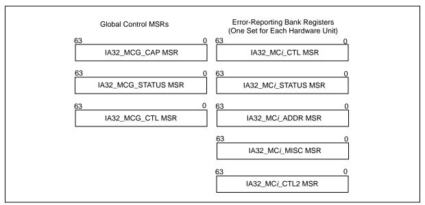
Figure 15-1. Machine-Check MSRs
