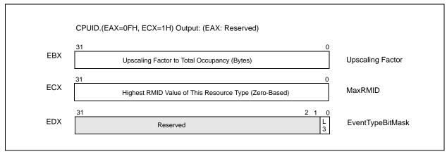
Figure 17-20. L3 Cache QoS Monitoring Capability Enumeration (CPUID.(EAX=0FH, ECX=1H))
