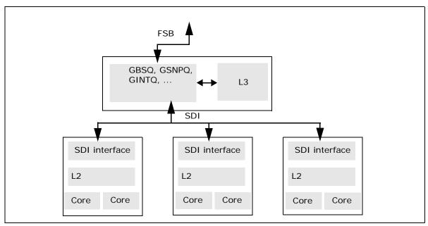
Figure 18-47. Block Diagram of Intel Xeon Processor 7400 Series
