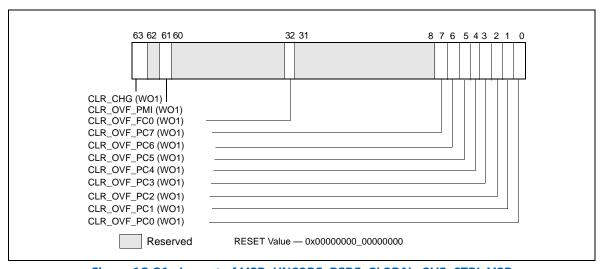
Figure 18-21. Layout of MSR\_UNCORE\_PERF\_GLOBAL\_OVF\_CTRL MSR
