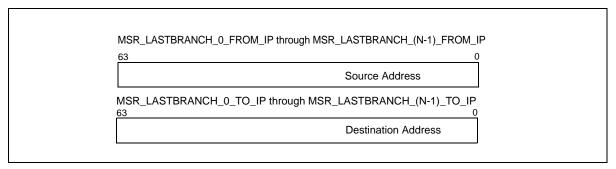
Figure 17-4. 64-bit Address Layout of LBR MSR
