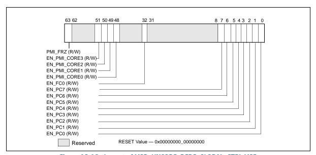
Figure 18-19. Layout of MSR\_UNCORE\_PERF\_GLOBAL\_CTRL MSR
