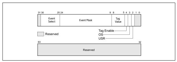
Figure 18-35. Event Selection Control Register (ESCR) for Pentium 4 and Intel Xeon Processors without Intel HT Technology Support
