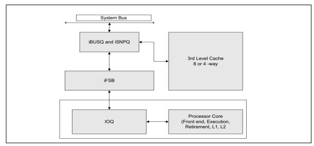
Figure 18-42. Block Diagram of 64-bit Intel Xeon Processor MP with 8-MByte L3
