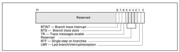
Figure 17-14. IA32\_DEBUGCTL MSR for Intel Core Solo and Intel Core Duo Processors
