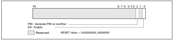
Figure 18-23. Layout of MSR UNCORE FIXED CTR CTRL MSR
