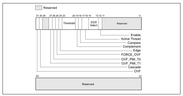
Figure 18-40. Counter Configuration Control Register (CCCR)
