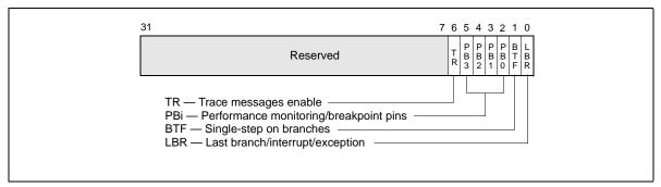
Figure 17-18. DEBUGCTLMSR Register (P6 Family Processors)
