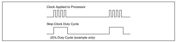
Figure 14-5. Processor Modulation Through Stop-Clock Mechanism
