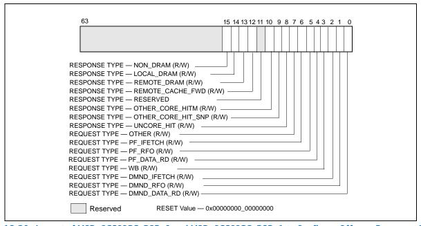
Figure 18-20. Layout of MSR\_OFFCORE\_RSP\_0 and MSR\_OFFCORE\_RSP\_1 to Configure Off-core Response Events
