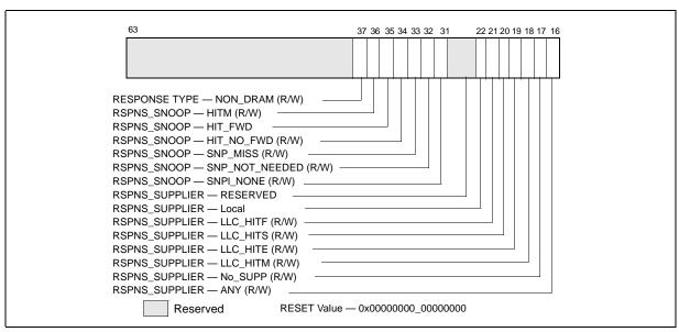
Figure 18-33. Response\_Supplier and Snoop Info Fields for MSR\_OFFCORE\_RSP\_x
