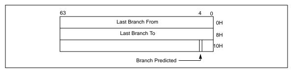
Figure 17-9. 64-bit Branch Trace Record Format
