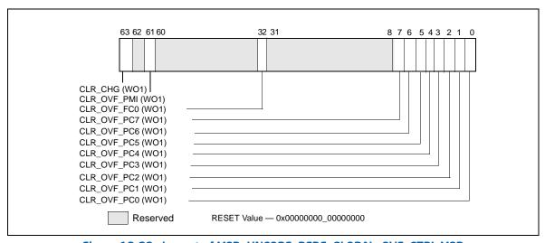
Figure 18-23. Layout of MSR\_UNCORE\_PERF\_GLOBAL\_OVF\_CTRL MSR
