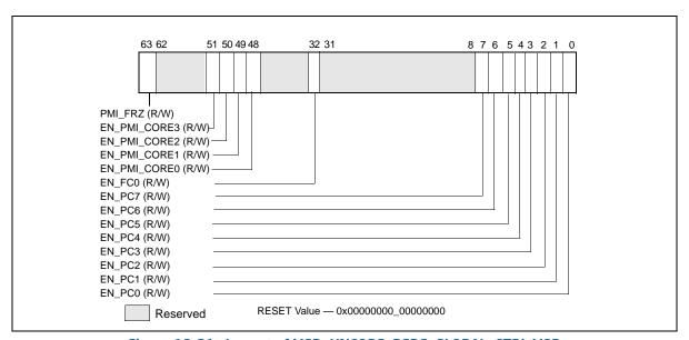
Figure 18-21. Layout of MSR\_UNCORE\_PERF\_GLOBAL\_CTRL MSR
