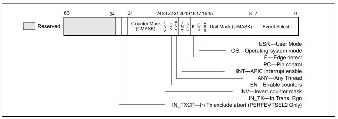
Figure 18-36. Layout of IA32\_PERFEVTSELx MSRs Supporting Intel TSX
