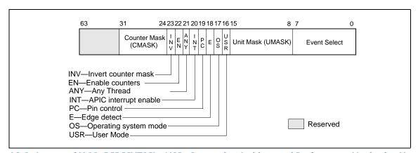
Figure 18-6. Layout of IA32\_PERFEVTSELx MSRs Supporting Architectural Performance Monitoring Version 3
