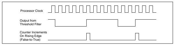
Figure 18-40. Effects of Edge Filtering
