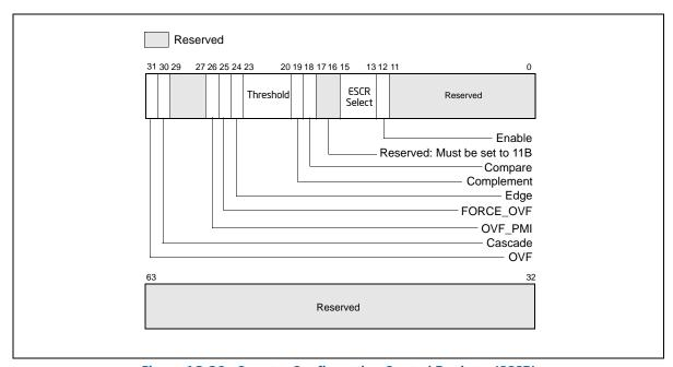
Figure 18-39. Counter Configuration Control Register (CCCR)
