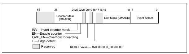
Figure 18-34. Layout of Uncore PERFEVTSEL MSR for a C-Box Unit or the ARB Unit
