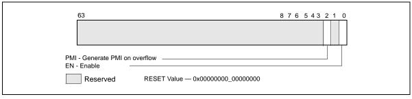
Figure 18-25. Layout of MSR UNCORE FIXED CTR CTRL MSR
