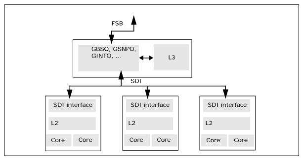
Figure 18-49. Block Diagram of Intel Xeon Processor 7400 Series
