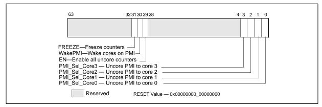
Figure 18-35. Layout of MSR\_UNC\_PERF\_GLOBAL\_CTRL MSR for Uncore
