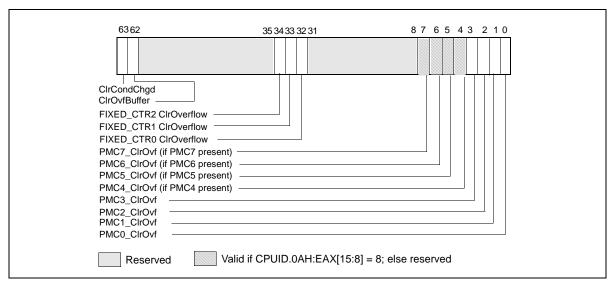
Figure 18-30. IA32\_PERF\_GLOBAL\_OVF\_CTRL MSR in Intel microarchitecture code name Sandy Bridge
