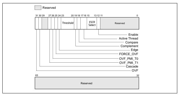
Figure 18-42. Counter Configuration Control Register (CCCR)
