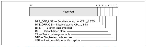
Figure 17-12. MSR\_DEBUGCTLA MSR for Pentium 4 and Intel Xeon Processors
