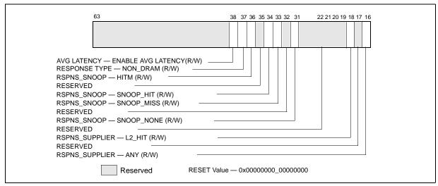
Figure 18-15. Response Supplier and Snoop Info Fields for MSR OFFCORE RSPx
