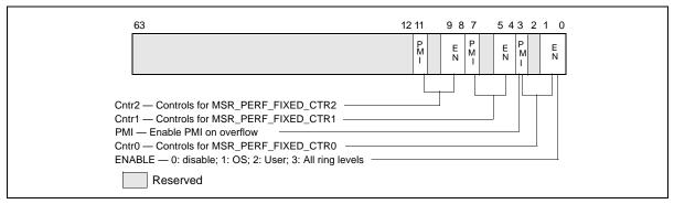
Figure 18-10. Layout of MSR\_PERF\_FIXED\_CTR\_CTRL MSR
