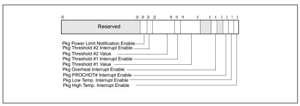
Figure 14-15. IA32\_PACKAGE\_THERM\_INTERRUPT Register
