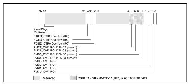
Figure 18-29. IA32\_PERF\_GLOBAL\_STATUS MSR in Intel® Microarchitecture Code Name Sandy Bridge
