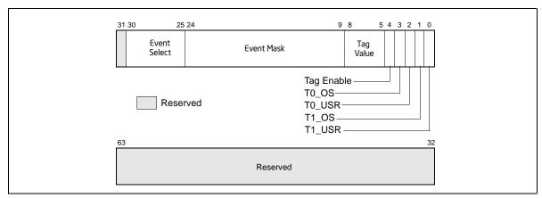
Figure 18-41. Event Selection Control Register (ESCR) for the Pentium 4 Processor, Intel Xeon Processor and Intel Xeon Processor MP Supporting Hyper-Threading Technology
