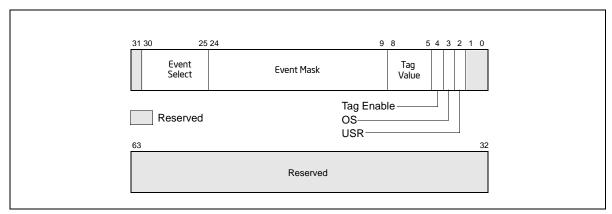
Figure 18-37. Event Selection Control Register (ESCR) for Pentium 4 and Intel Xeon Processors without Intel HT Technology Support
