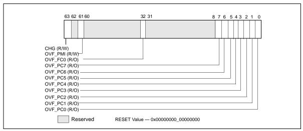
Figure 18-22. Layout of MSR\_UNCORE\_PERF\_GLOBAL\_STATUS MSR
