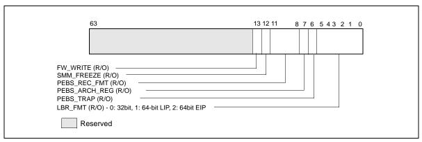
Figure 18-43. Layout of IA32\_PERF\_CAPABILITIES MSR
