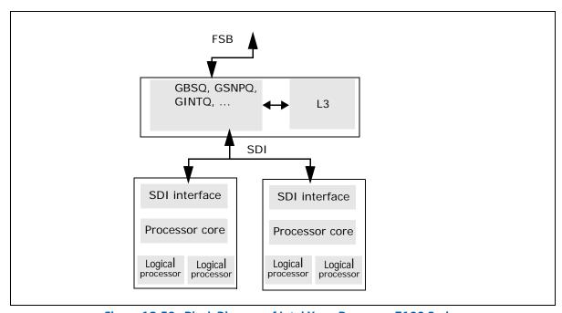
Figure 18-50. Block Diagram of Intel Xeon Processor 7100 Series
