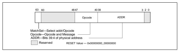
Figure 18-26. Layout of MSR UNCORE ADDR OPCODE MATCH MSR
