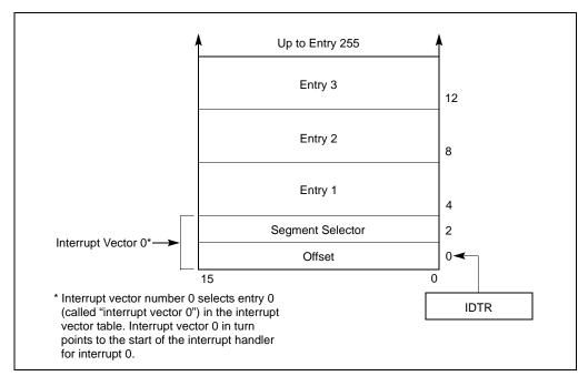
Figure 20-2. Interrupt Vector Table in Real-Address Mode
