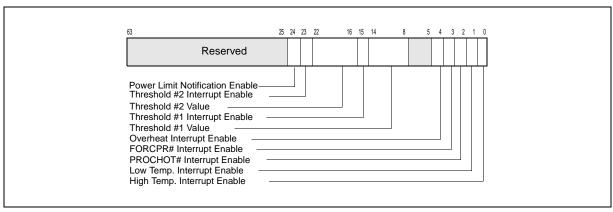
Figure 14-13. IA32\_THERM\_INTERRUPT Register
