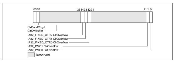
Figure 18-5. Layout of IA32 PERF GLOBAL OVF CTRL MSR
