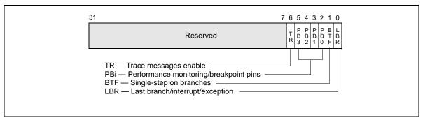
Figure 17-18. DEBUGCTLMSR Register (P6 Family Processors)
