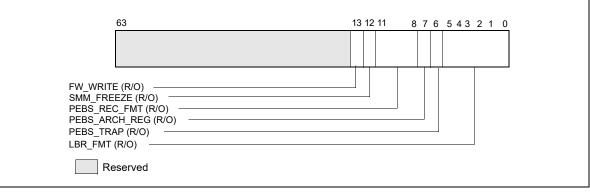
Figure 18-49. Layout of IA32\_PERF\_CAPABILITIES MSR
