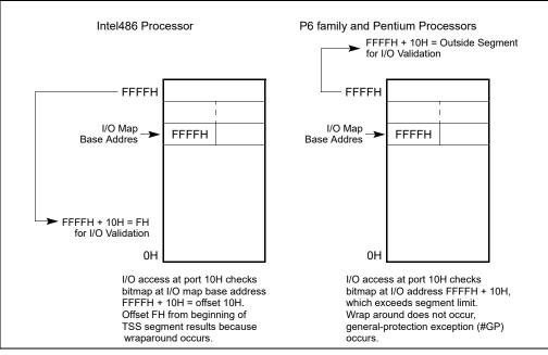
Figure 22-1. I/O Map Base Address Differences
