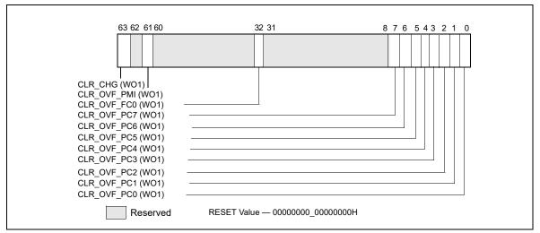
Figure 18-27. Layout of MSR\_UNCORE\_PERF\_GLOBAL\_OVF\_CTRL MSR
