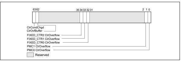
Figure 18-17. Layout of MSR\_PERF\_GLOBAL\_OVF\_CTRL MSR
