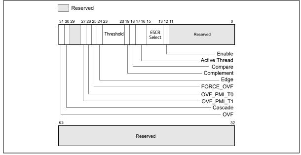
Figure 18-48. Counter Configuration Control Register (CCCR)
