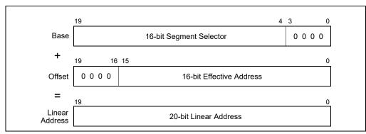
Figure 20-1. Real-Address Mode Address Translation
