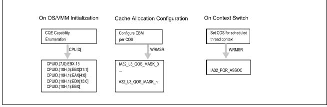
Figure 17-30. Cache Allocation Technology Usage Flow
