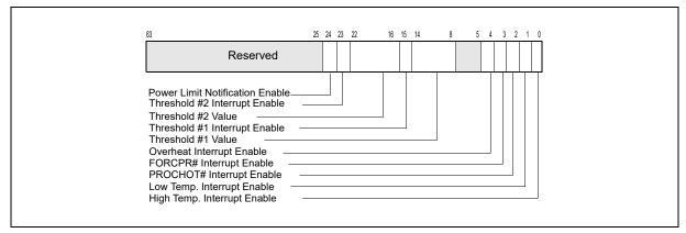
Figure 14-28. IA32\_THERM\_INTERRUPT Register
