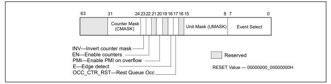
Figure 18-28. Layout of MSR\_UNCORE\_PERFEVTSELx MSRs
