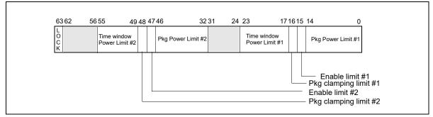
Figure 14-32. MSR\_PKG\_POWER\_LIMIT Register
