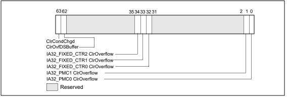
Figure 18-5. Layout of IA32\_PERF\_GLOBAL\_OVF\_CTRL MSR
