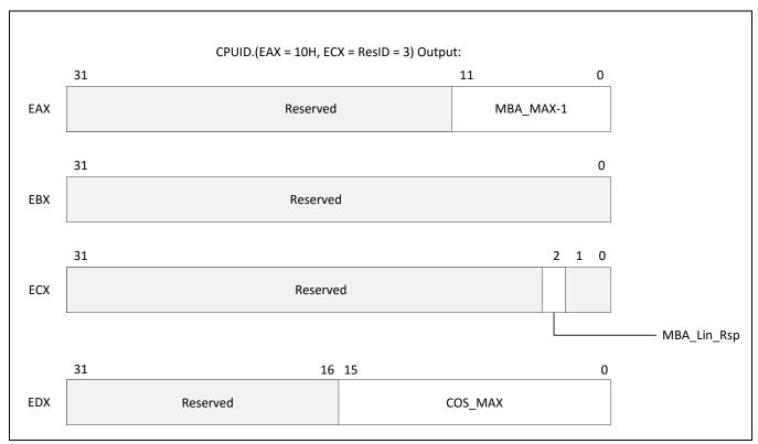
Figure 17-38. CPUID.(EAX=10H, ECX=3H) MBA Feature Details Identification
