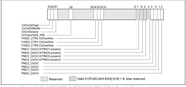
Figure 18-42. IA32\_PERF\_GLOBAL\_OVF\_CTRL MSR in Broadwell microarchitecture
