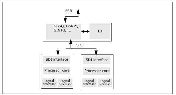
Figure 18-56. Block Diagram of Intel Xeon Processor 7100 Series
