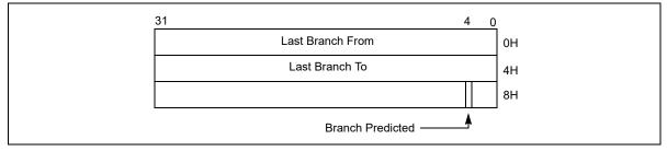
Figure 17-6. 32-bit Branch Trace Record Format
