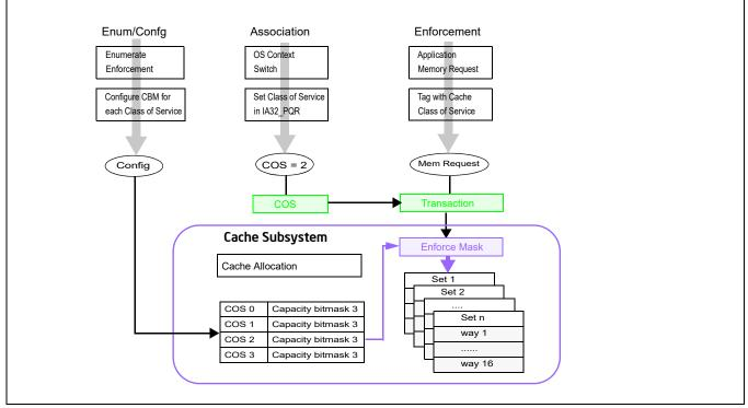
Figure 17-28. Class of Service and Cache Capacity Bitmasks
