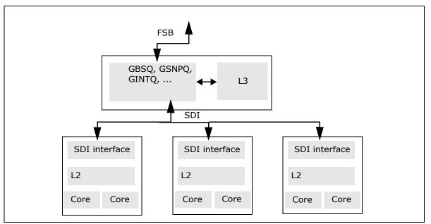
Figure 18-55. Block Diagram of Intel Xeon Processor 7400 Series
