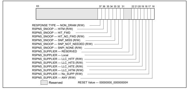
Figure 18-37. Response\_Supplier and Snoop Info Fields for MSR\_OFFCORE\_RSP\_x
