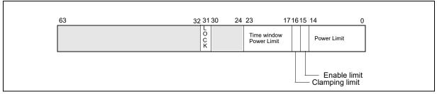
Figure 14-36. MSR\_PP0\_POWER\_LIMIT/MSR\_PP1\_POWER\_LIMIT Register
