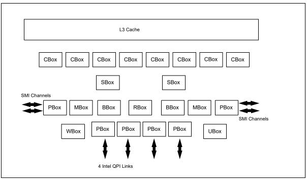
Figure 18-31. Distributed Units of the Uncore of Intel<sup>®</sup> Xeon<sup>®</sup> Processor 7500 Series
