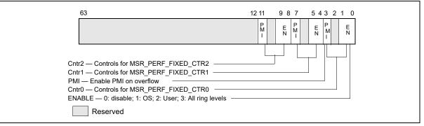
Figure 18-14. Layout of MSR\_PERF\_FIXED\_CTR\_CTRL MSR
