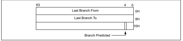
Figure 17-9. 64-bit Branch Trace Record Format
