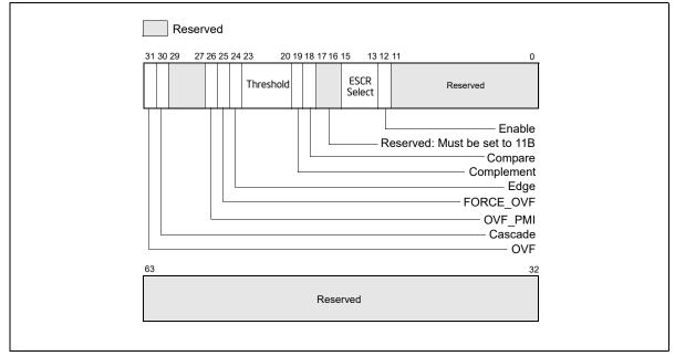
Figure 18-45. Counter Configuration Control Register (CCCR)
