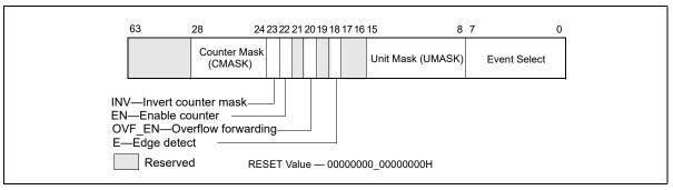
Figure 18-38. Layout of Uncore PERFEVTSEL MSR for a C-Box Unit or the ARB Unit
