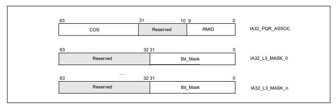
Figure 17-34. IA32\_PQR\_ASSOC, IA32\_L3\_MASK\_n MSRs
