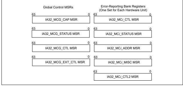
Figure 15-1. Machine-Check MSRs
