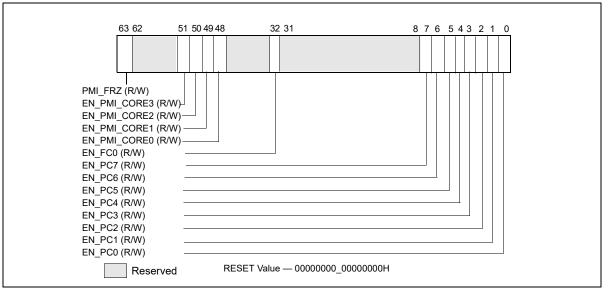
Figure 18-25. Layout of MSR\_UNCORE\_PERF\_GLOBAL\_CTRL MSR
