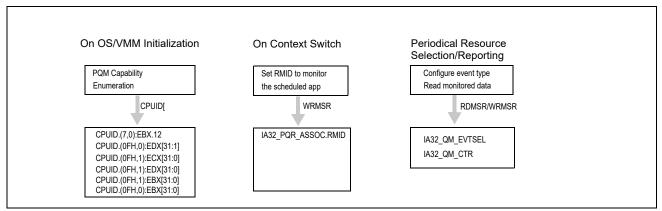
Figure 17-19. Platform Shared Resource Monitoring Usage Flow
