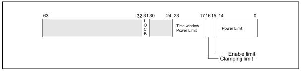
Figure 14-40. MSR\_DRAM\_POWER\_LIMIT Register
