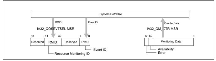
Figure 17-25. Software Usage of Cache Monitoring Resources
