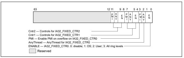
Figure 18-7. IA32\_FIXED\_CTR\_CTRL MSR Supporting Architectural Performance Monitoring Version 3
