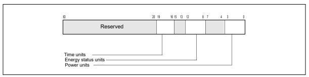
Figure 14-31. MSR\_RAPL\_POWER\_UNIT Register
