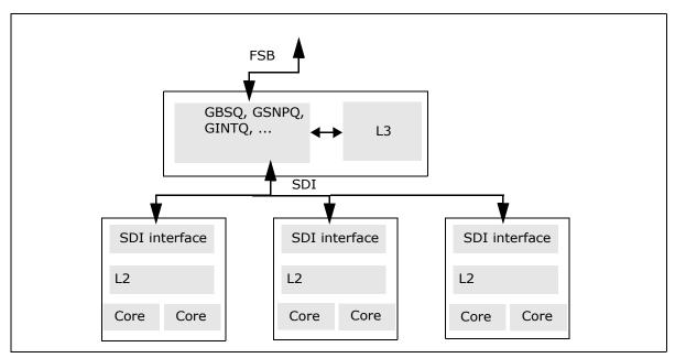
Figure 18-56. Block Diagram of Intel Xeon Processor 7400 Series
