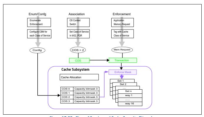
Figure 17-28. Class of Service and Cache Capacity Bitmasks
