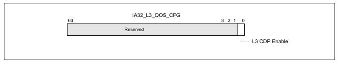
Figure 17-36. Layout of IA32 L3 QOS CFG
