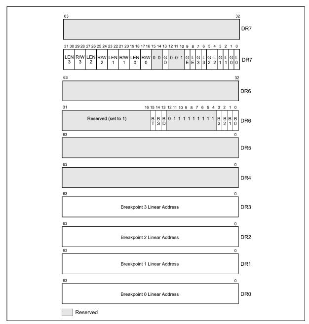
Figure 17-2. DR6/DR7 Layout on Processors Supporting Intel® 64 Architecture
