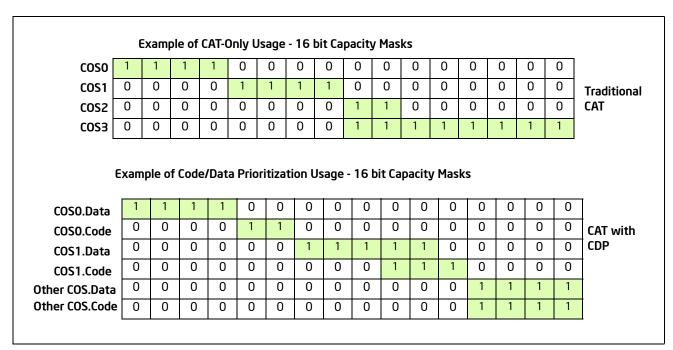
Figure 17-29. Code and Data Capacity Bitmasks of CDP
