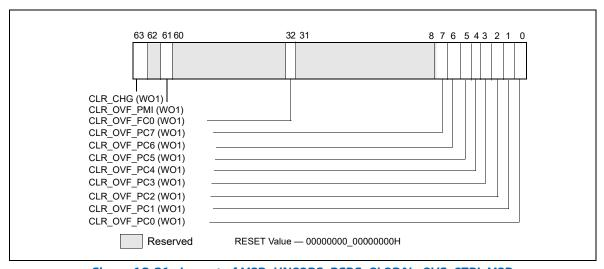
Figure 18-21. Layout of MSR\_UNCORE\_PERF\_GLOBAL\_OVF\_CTRL MSR
