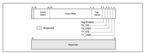
Figure 18-49. Event Selection Control Register (ESCR) for the Pentium 4 Processor, Intel Xeon Processor and Intel Xeon Processor MP Supporting Hyper-Threading Technology
