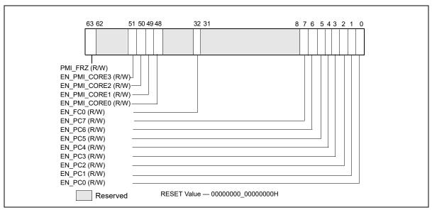
Figure 18-19. Layout of MSR\_UNCORE\_PERF\_GLOBAL\_CTRL MSR
