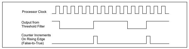
Figure 18-48. Effects of Edge Filtering
