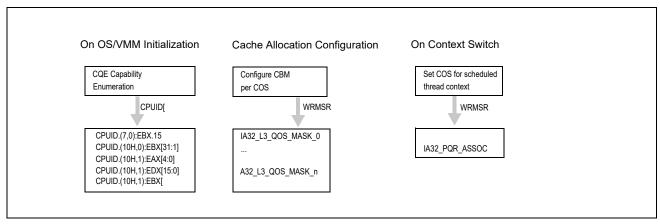
Figure 17-30. Cache Allocation Technology Usage Flow
