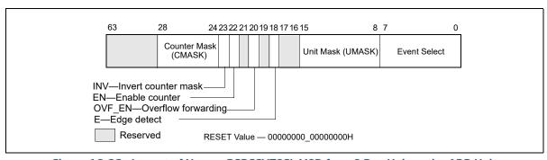
Figure 18-32. Layout of Uncore PERFEVTSEL MSR for a C-Box Unit or the ARB Unit
