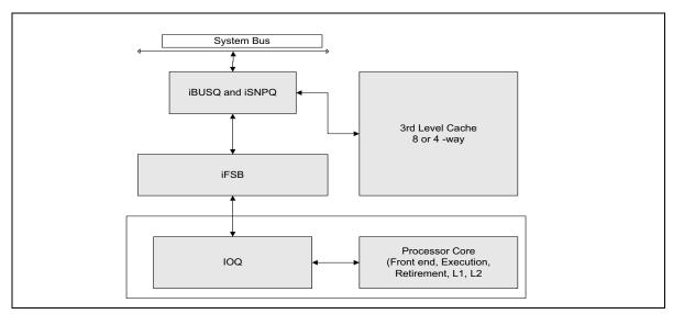
Figure 18-51. Block Diagram of 64-bit Intel Xeon Processor MP with 8-MByte L3
