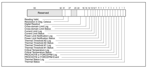
Figure 14-9. IA32\_THERM\_STATUS Register With HWP Feedback
