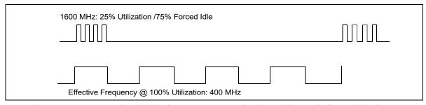
Figure 14-19. Example of Effective Frequency Reduction and Forced Idle Period of HDC
