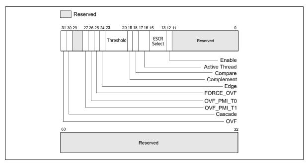
Figure 18-50. Counter Configuration Control Register (CCCR)
