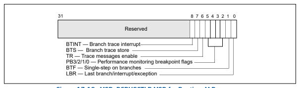
Figure 17-16. MSR\_DEBUGCTLB MSR for Pentium M Processors
