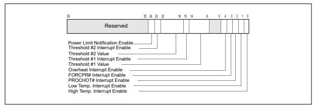
Figure 14-28. IA32\_THERM\_INTERRUPT Register
