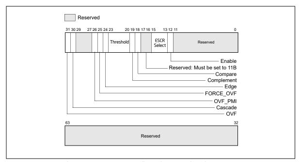
Figure 18-47. Counter Configuration Control Register (CCCR)
