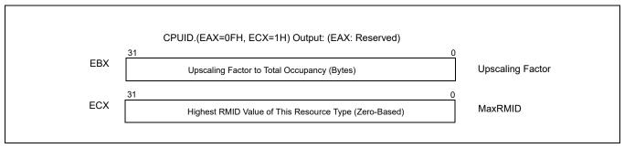
Figure 17-21. L3 Cache Monitoring Capability Enumeration Data (CPUID.(EAX=0FH, ECX=1H))
