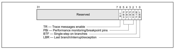
Figure 17-18. DEBUGCTLMSR Register (P6 Family Processors)
