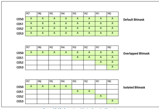
Figure 17-27. Examples of Cache Capacity Bitmasks
