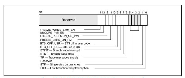
Figure 17-11. IA32\_DEBUGCTL MSR for Processors based on Intel microarchitecture code name Nehalem
