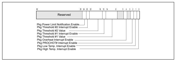
Figure 14-30. IA32\_PACKAGE\_THERM\_INTERRUPT Register
