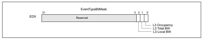
Figure 17-22. L3 Cache Monitoring Capability Enumeration Event Type Bit Vector (CPUID.(EAX=0FH, ECX=1H))
