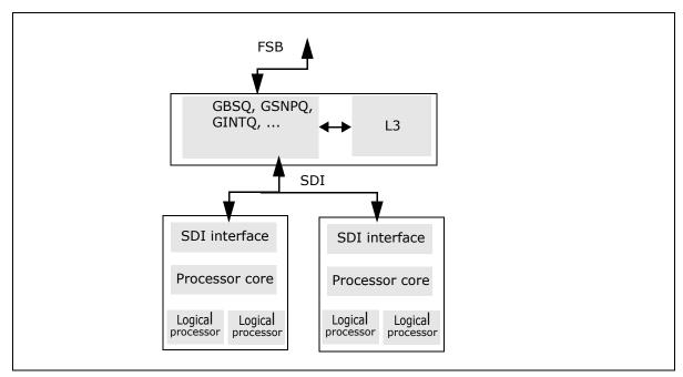
Figure 18-57. Block Diagram of Intel Xeon Processor 7100 Series
