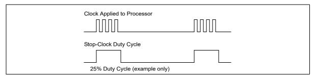
Figure 14-20. Processor Modulation Through Stop-Clock Mechanism
