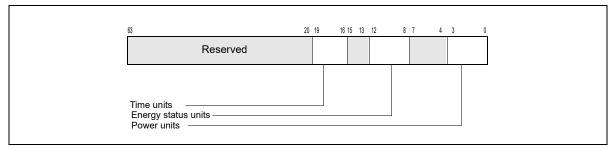
Figure 14-31. MSR\_RAPL\_POWER\_UNIT Register
