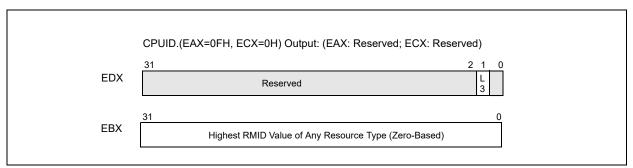
Figure 17-20. CPUID.(EAX=0FH, ECX=0H) Monitoring Resource Type Enumeration
