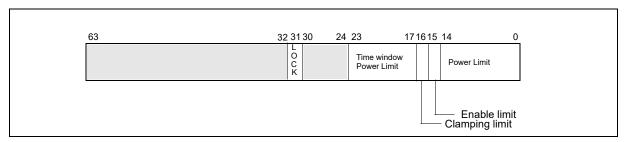
Figure 14-36. MSR\_PP0\_POWER\_LIMIT/MSR\_PP1\_POWER\_LIMIT Register
