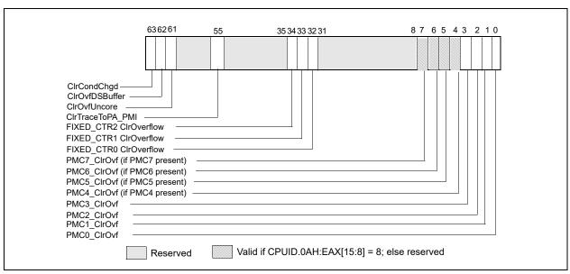
Figure 18-36. IA32\_PERF\_GLOBAL\_OVF\_CTRL MSR in Broadwell microarchitecture
