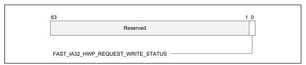
Figure 14-15. FAST\_UNCORE\_MSRS\_STATUS MSR
