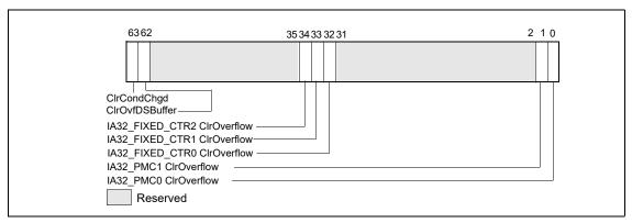
Figure 18-5. Layout of IA32\_PERF\_GLOBAL\_OVF\_CTRL MSR
