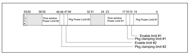
Figure 14-36. MSR\_PKG\_POWER\_LIMIT Register
