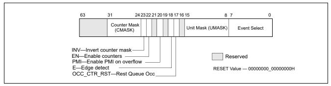
Figure 18-22. Layout of MSR\_UNCORE\_PERFEVTSELx MSRs
