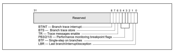
Figure 17-16. MSR\_DEBUGCTLB MSR for Pentium M Processors
