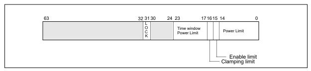
Figure 14-40. MSR\_PP0\_POWER\_LIMIT/MSR\_PP1\_POWER\_LIMIT Register
