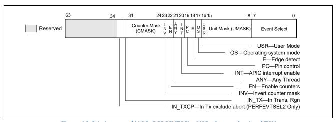
Figure 18-34. Layout of IA32\_PERFEVTSELx MSRs Supporting Intel TSX
