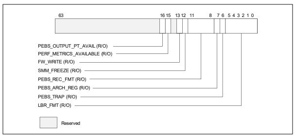
Figure 18-63. Layout of IA32\_PERF\_CAPABILITIES MSR
