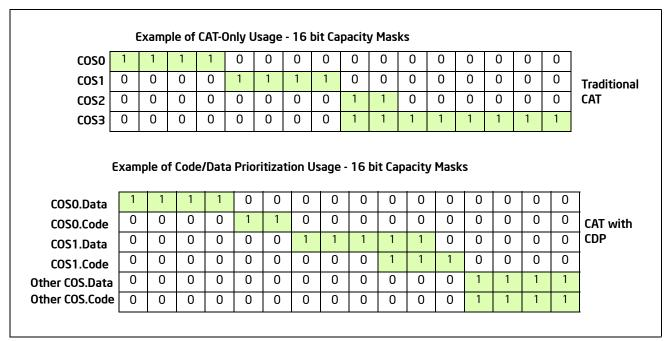
Figure 17-29. Code and Data Capacity Bitmasks of CDP
