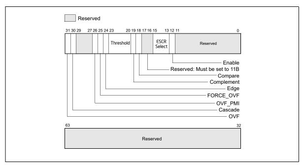
Figure 18-47. Counter Configuration Control Register (CCCR)
