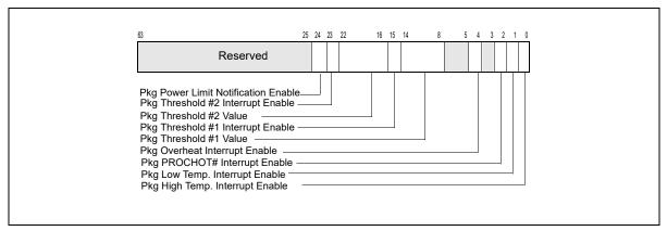
Figure 14-34. IA32\_PACKAGE\_THERM\_INTERRUPT Register
