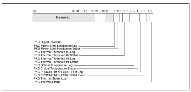
Figure 14-33. IA32\_PACKAGE\_THERM\_STATUS Register
