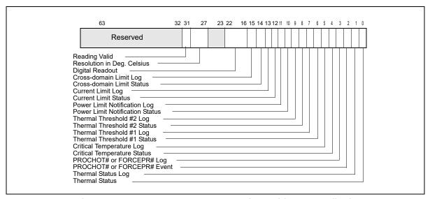
Figure 14-10. IA32\_THERM\_STATUS Register With HWP Feedback
