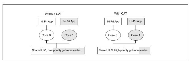
Figure 17-26. Cache Allocation Technology Enables Allocation of More Resources to High Priority Applications
