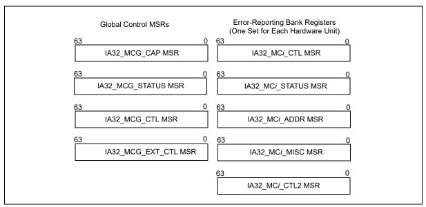
Figure 15-1. Machine-Check MSRs
