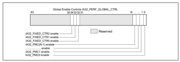
Figure 18-8. Layout of Global Performance Monitoring Control MSR
