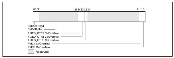
Figure 18-44. Layout of MSR\_PERF\_GLOBAL\_OVF\_CTRL MSR
