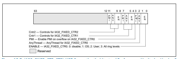
Figure 18-7. IA32\_FIXED\_CTR\_CTRL MSR Supporting Architectural Performance Monitoring Version 3
