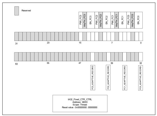
Figure 18-66. Layout of IA32\_FIXED\_CTR\_CTRL MSR Supporting Adaptive PEBS
