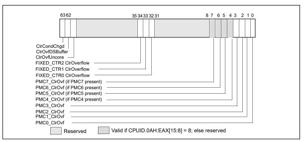
Figure 18-28. IA32\_PERF\_GLOBAL\_OVF\_CTRL MSR in Intel microarchitecture code name Sandy Bridge
