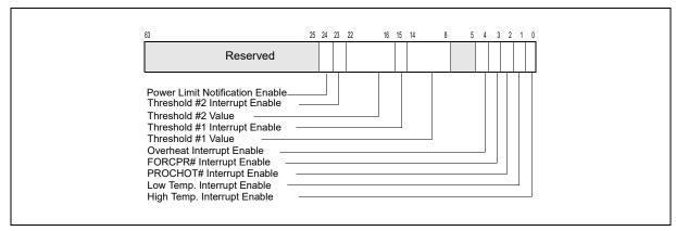
Figure 14-32. IA32\_THERM\_INTERRUPT Register
