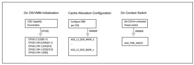
Figure 17-30. Cache Allocation Technology Usage Flow
