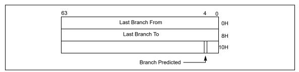
Figure 17-9. 64-bit Branch Trace Record Format
