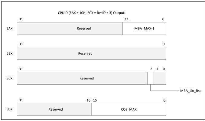
Figure 17-39. CPUID.(EAX=10H, ECX=3H) MBA Feature Details Identification
