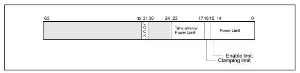
Figure 14-44. MSR\_DRAM\_POWER\_LIMIT Register
