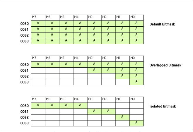
Figure 17-27. Examples of Cache Capacity Bitmasks
