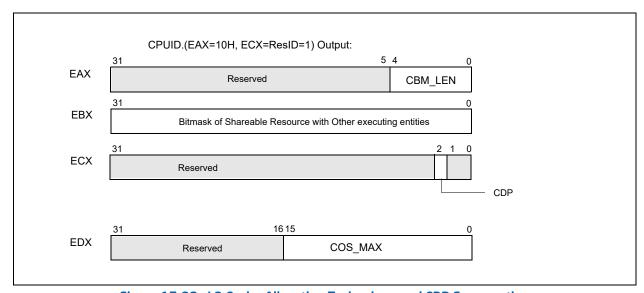
Figure 17-32. L3 Cache Allocation Technology and CDP Enumeration
