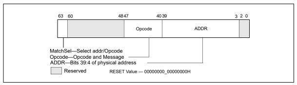
Figure 18-24. Layout of MSR UNCORE ADDR OPCODE MATCH MSR
