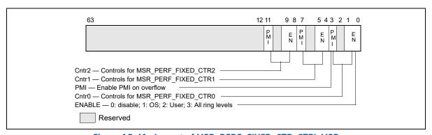
Figure 18-41. Layout of MSR\_PERF\_FIXED\_CTR\_CTRL MSR
