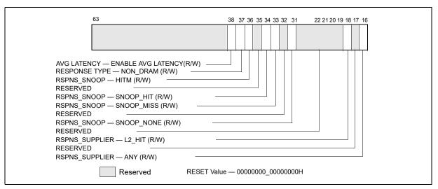
Figure 18-39. Response Supplier and Snoop Info Fields for MSR OFFCORE RSPx
