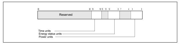
Figure 14-35. MSR\_RAPL\_POWER\_UNIT Register
