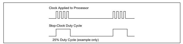
Figure 14-24. Processor Modulation Through Stop-Clock Mechanism
