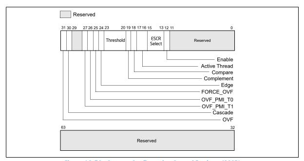
Figure 18-50. Counter Configuration Control Register (CCCR)
