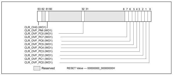
Figure 18-21. Layout of MSR\_UNCORE\_PERF\_GLOBAL\_OVF\_CTRL MSR
