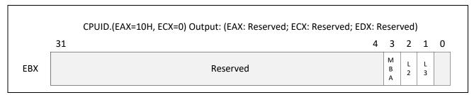
Figure 17-31. CPUID.(EAX=10H, ECX=0H) Available Resource Type Identification
