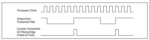
Figure 18-48. Effects of Edge Filtering
