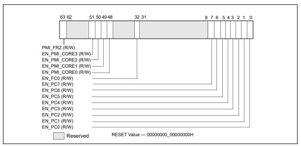
Figure 18-19. Layout of MSR\_UNCORE\_PERF\_GLOBAL\_CTRL MSR
