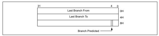
Figure 17-6. 32-bit Branch Trace Record Format
