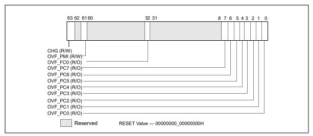
Figure 18-20. Layout of MSR\_UNCORE\_PERF\_GLOBAL\_STATUS MSR
