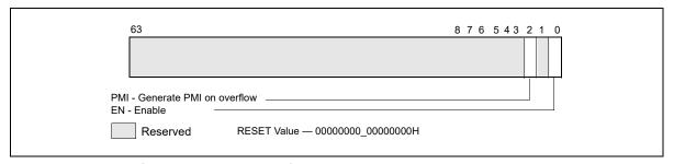
Figure 18-23. Layout of MSR\_UNCORE\_FIXED\_CTR\_CTRL MSR
