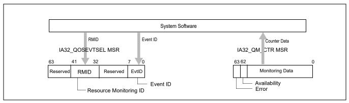
Figure 17-25. Software Usage of Cache Monitoring Resources
