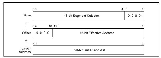
Figure 20-1. Real-Address Mode Address Translation
