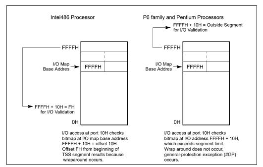
Figure 22-1. I/O Map Base Address Differences
