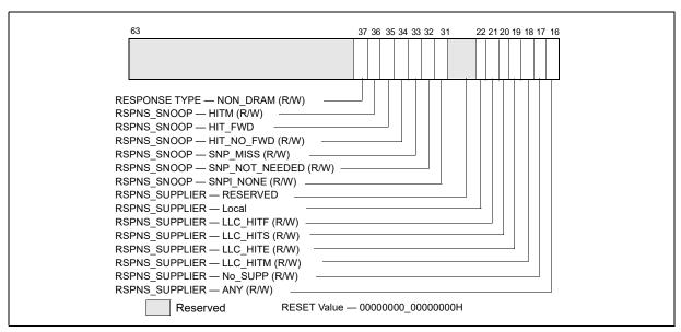
Figure 18-31. Response\_Supplier and Snoop Info Fields for MSR\_OFFCORE\_RSP\_x
