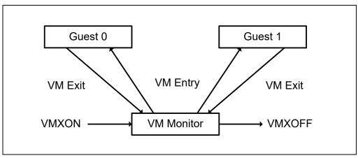
Figure 24-1. Interaction of a Virtual-Machine Monitor and Guests
