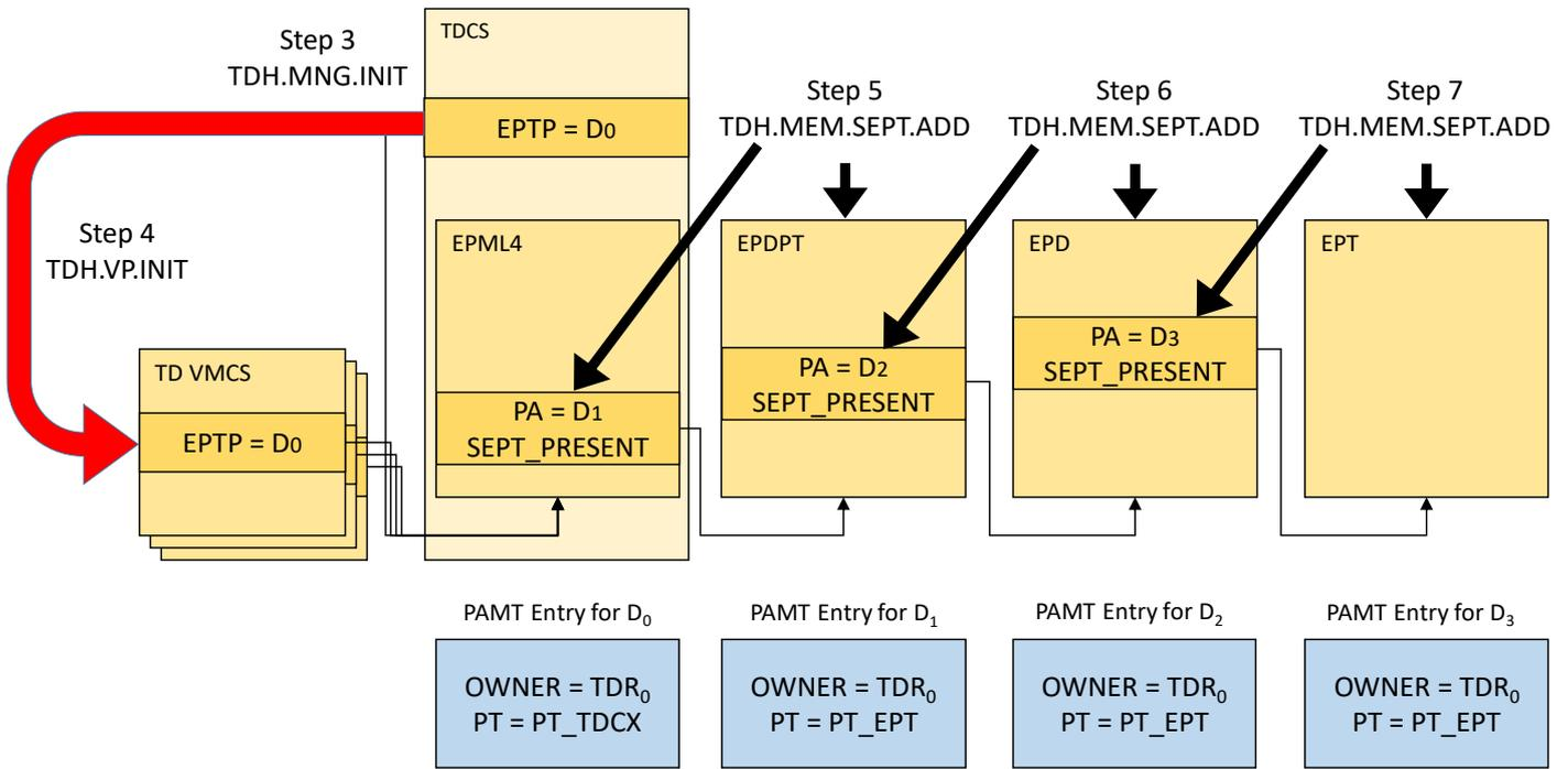
**Figure 7.3: Typical Secure EPT Hierarchy Build Process**
