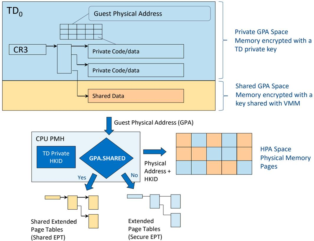
Figure 2.3: Secure EPT Concept
