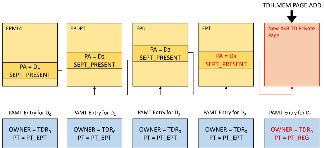
Figure 7.4: Typical Sequence for Adding a TD Private Page during TD Build Time
