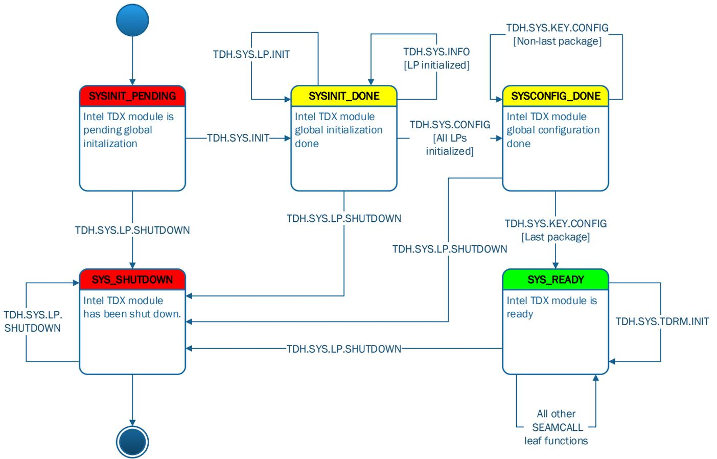
Figure 12.1: Intel TDX Module Lifecycle State Machine
