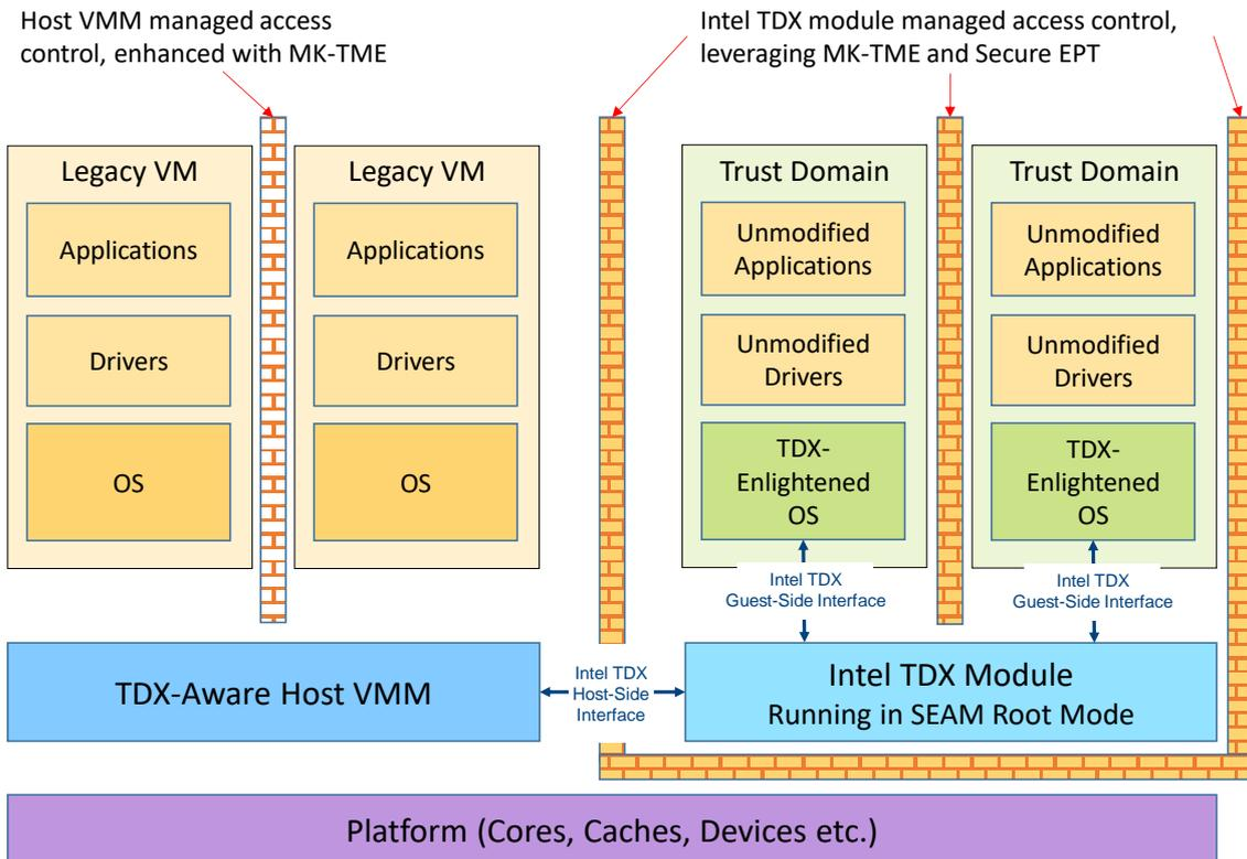
Figure 2.1: Intel® Trust Domain Extension Components Overview
