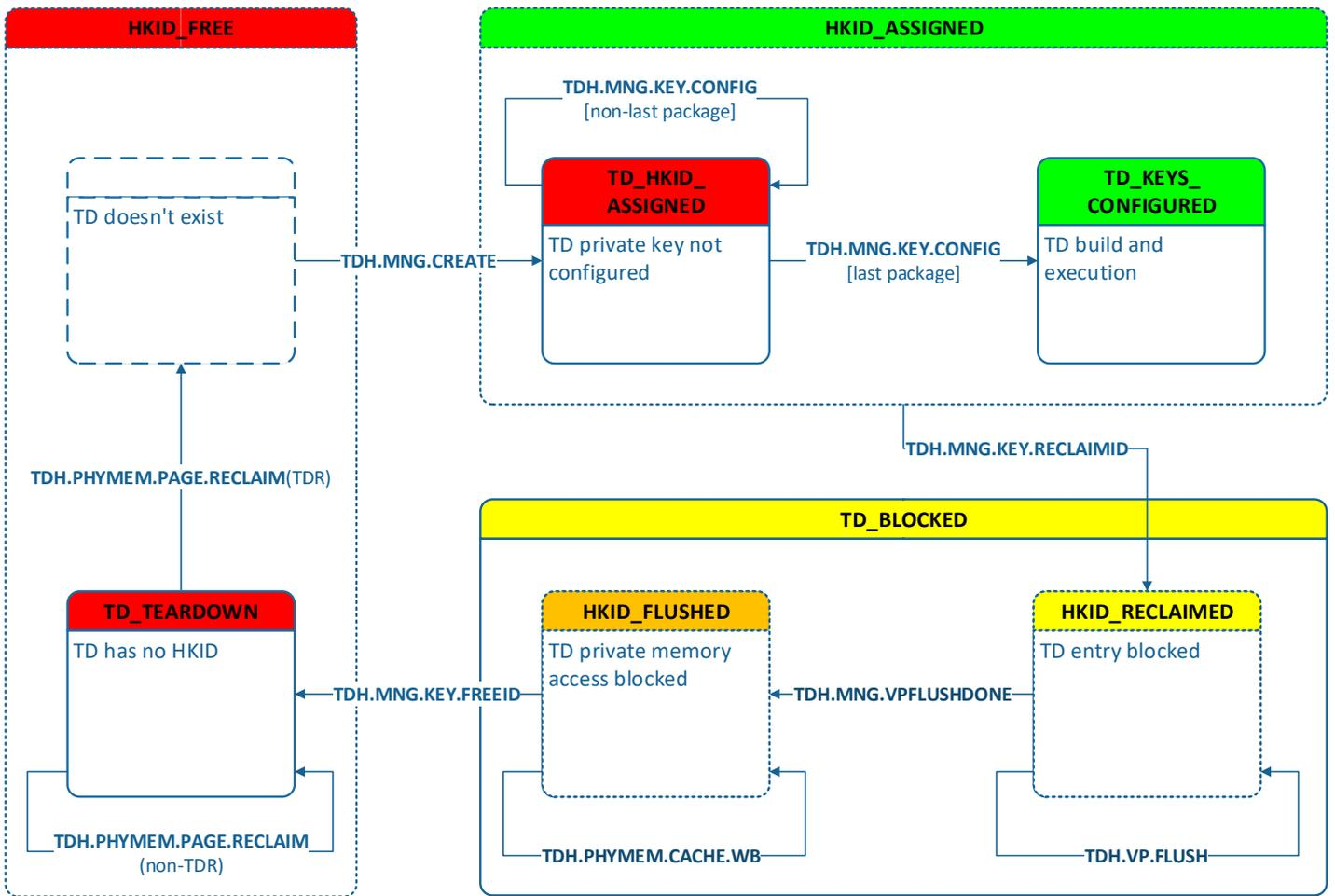
Figure 4.2: Simplified Combined TD Key Management State Diagram
