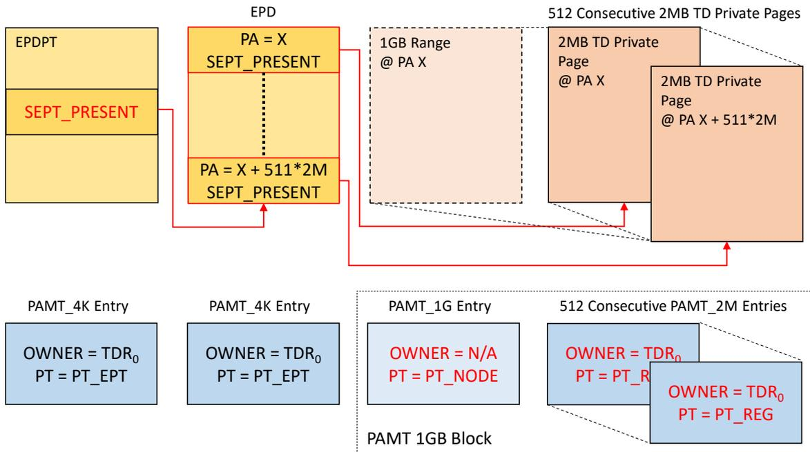
**Figure 7.10: Typical State of a 1GB TD Private Range after TDH.MEM.PAGE.DEMOTE**
