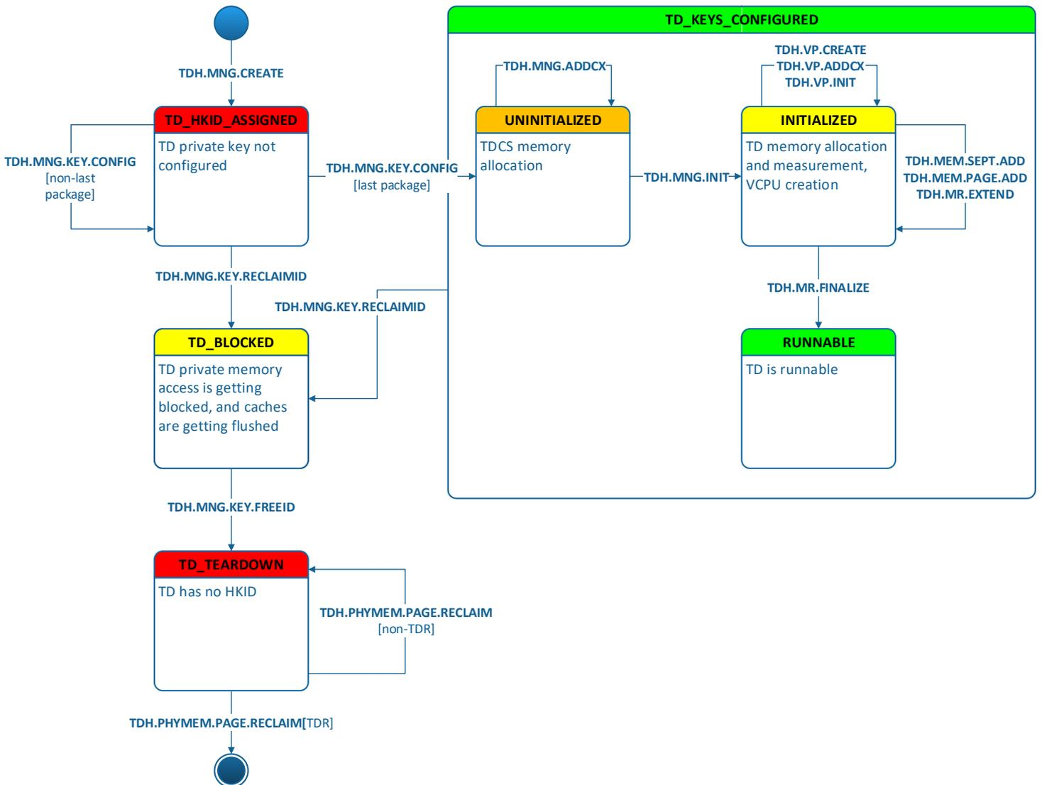
**Figure 5.3: High-Level TD Life Cycle State Diagram**
