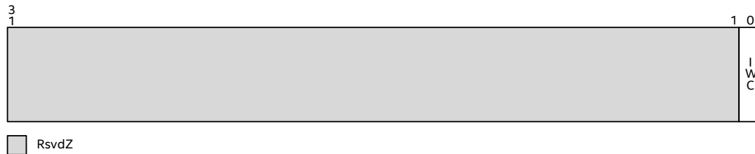
Figure 11-24. Invalidation Completion Status Register
